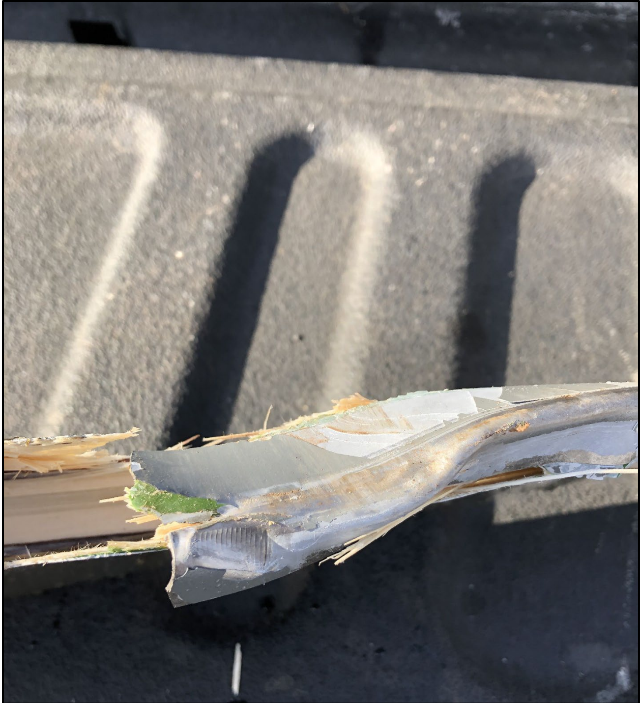
Figure 10: Thread Impression on Right Engine Propeller
