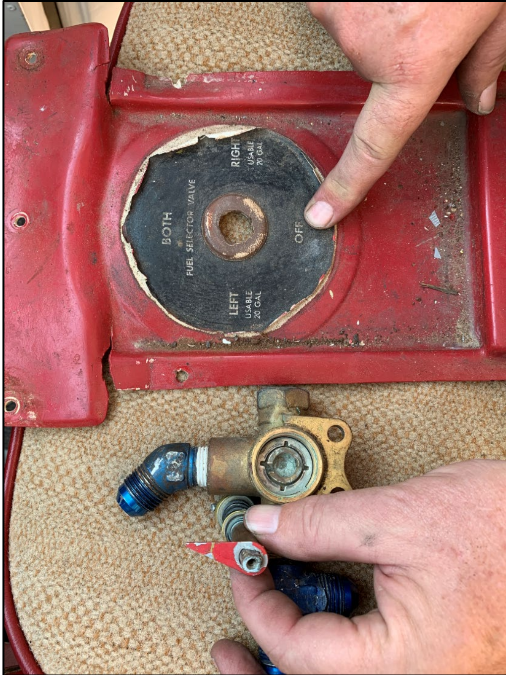
Figure 3 – View of the removed fuel selector.
