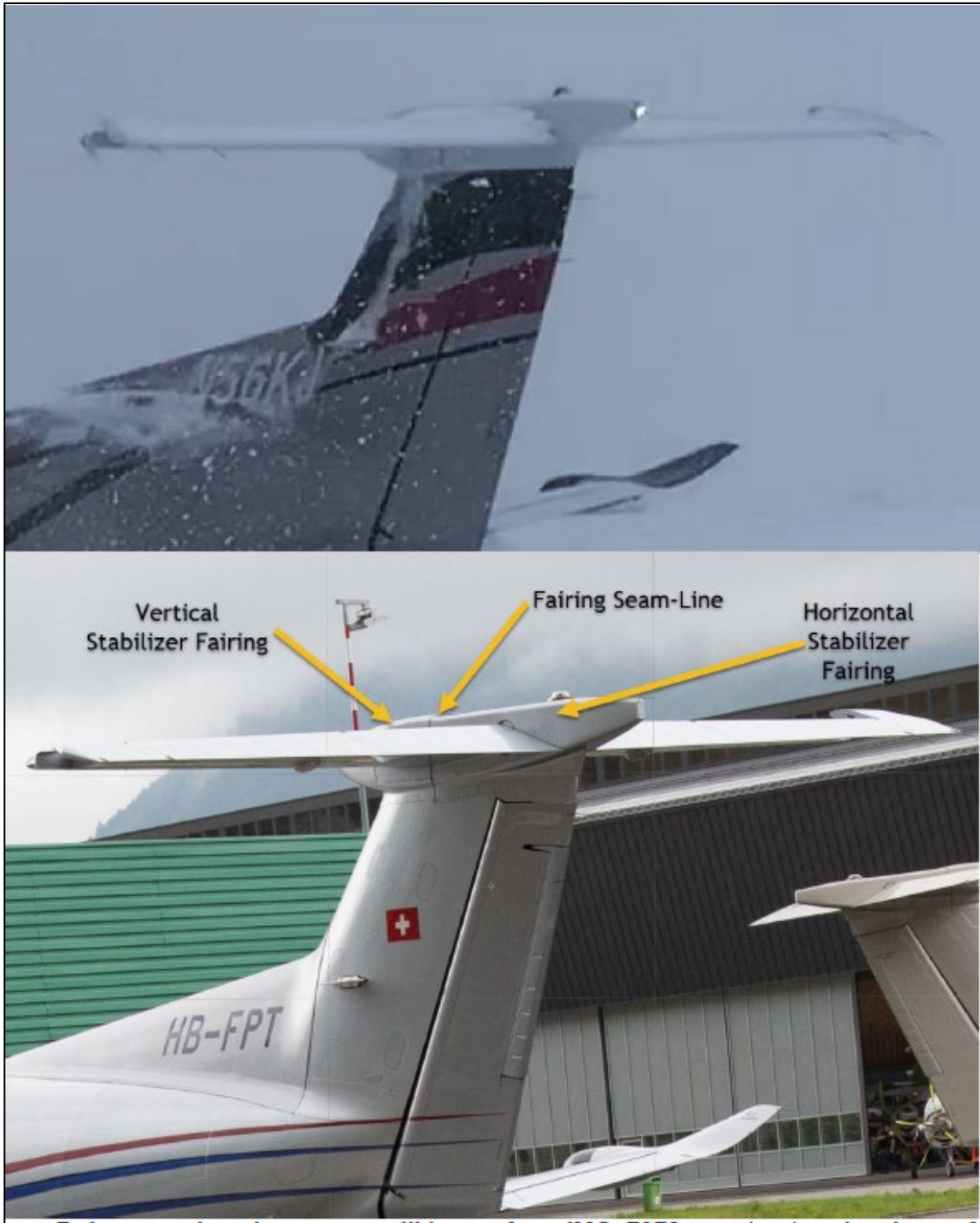
Figure 3. Comparison of N56KJ's horizontal tail area before takeoff on the accident flight with an exemplar airplane (from Reference 2).
