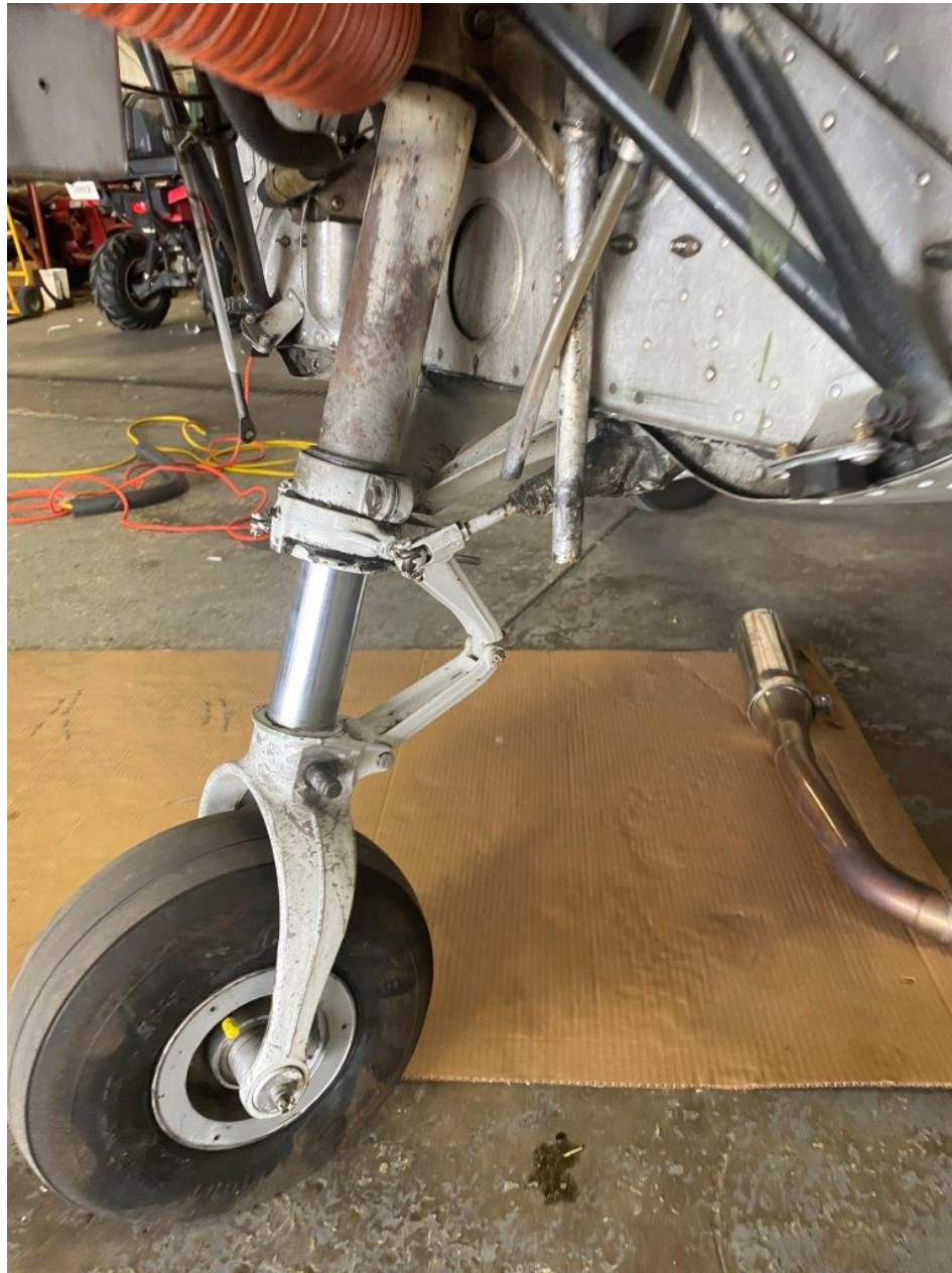
Photo 1 – Damage to the Nosewheel and Lower Fuselage
