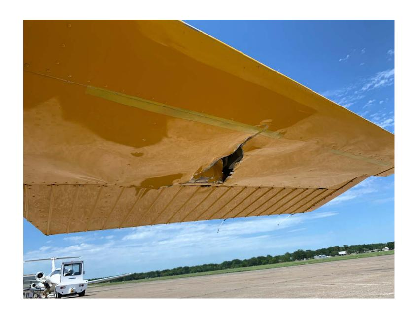
**Photo 1 – Entire Left Horizontal Stabilizer with Damage**
