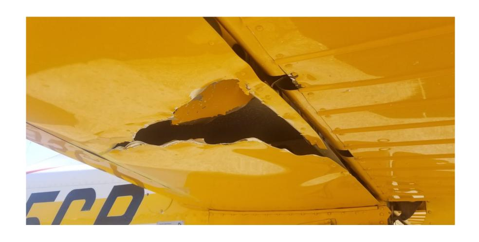
Photo 2 – Closer View of Damage to Left Horizontal Stabilizer
