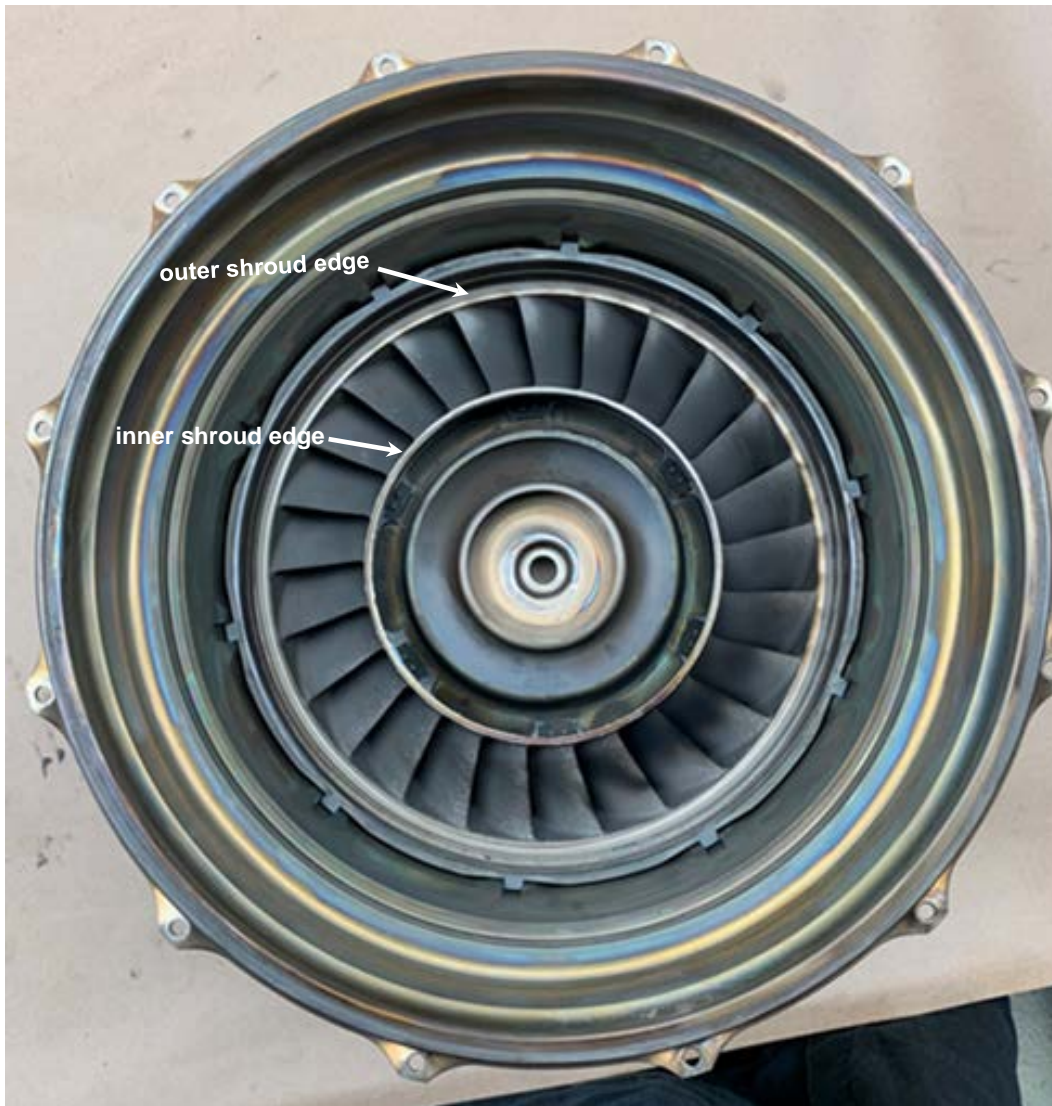
Figure 42. Downstream face of S1 PT guide vane ring and interstage baffle showing 360° inner and outer baffle shroud edge scoring
