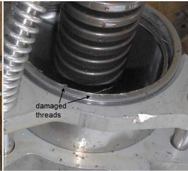
Figure 19. Cylinder separation from hub
