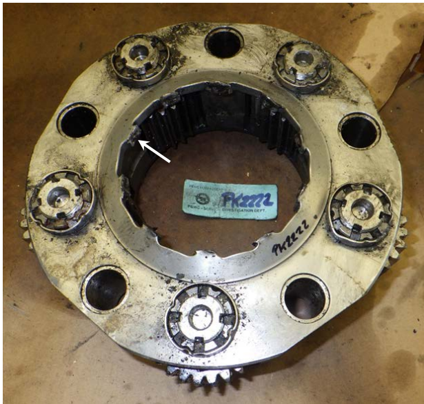
Figure 62. Aft side of S2 reduction gearbox planet gear with one web fracture surface noted
