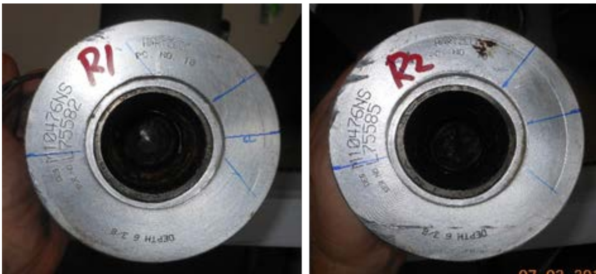
Figure 27. Blade butts with witness marks noted
