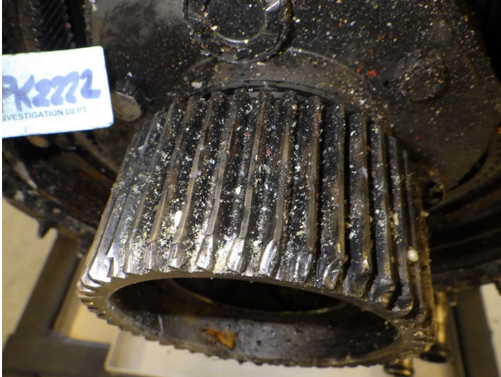
Figure 61. S2 sun gear tooth damage
