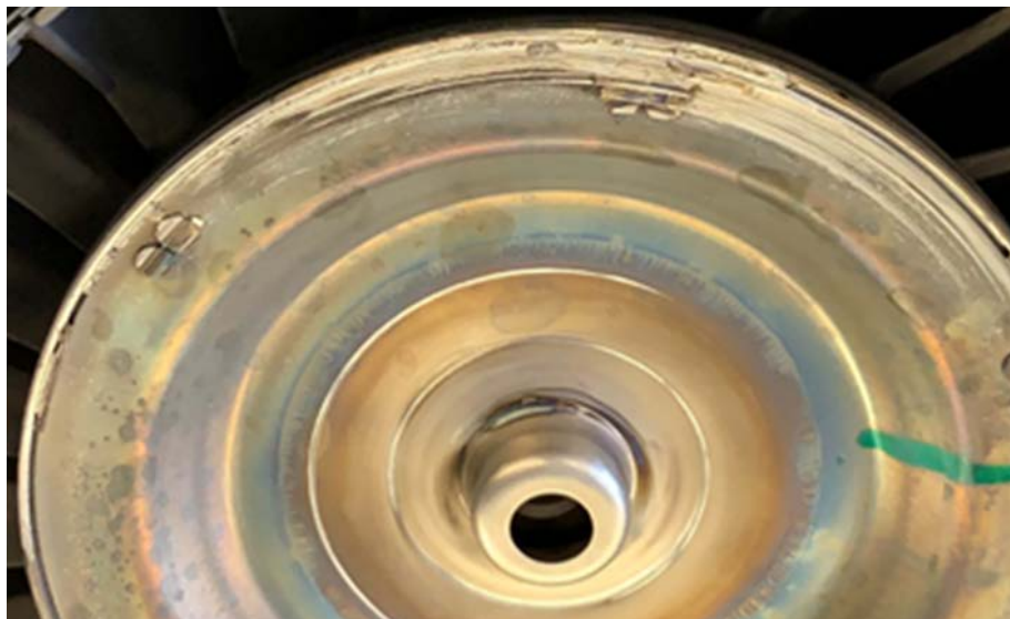
Figure 41. Detail of Figure 40 showing rotational damage signatures
