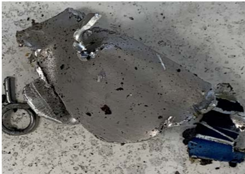
Figure 8. Propeller blade tip recovered inside hangar
