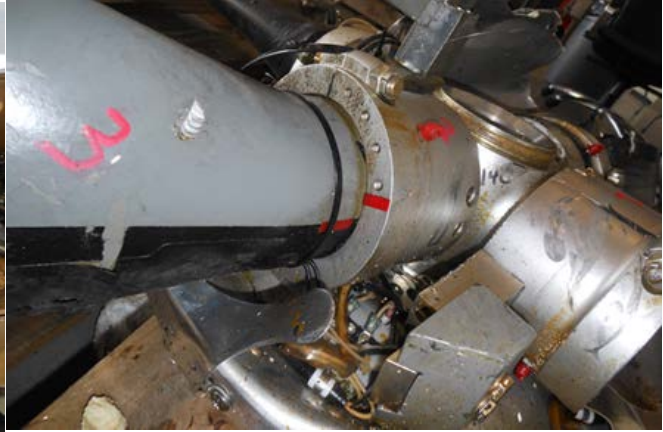
Figure 16. Blade-clamp interface showing slippage
