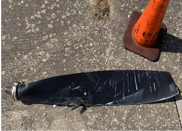
Figure 3. Liberated propeller blade showing transfer of white paint
