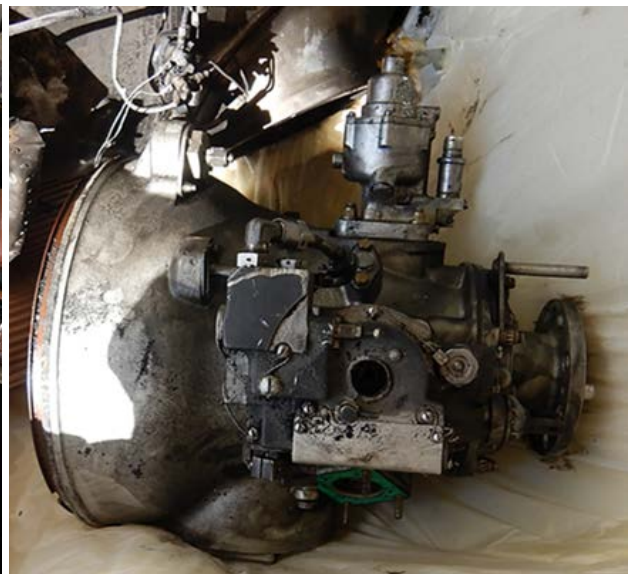
Figure 52. RGB section that separated with propeller
