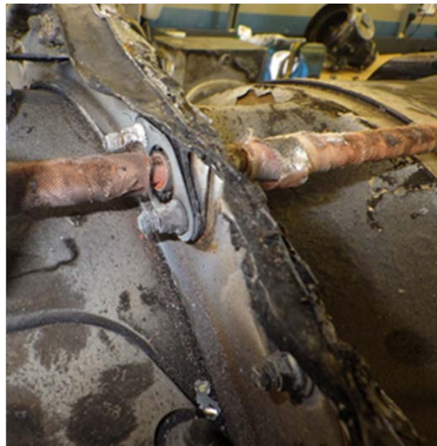
Figure 54. Propeller governor, showing impact damage Figure 55. Typical right engine thermal damage
