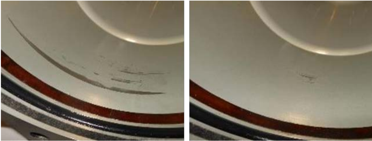
Figure 17 . Left propeller internal piston witness marks
