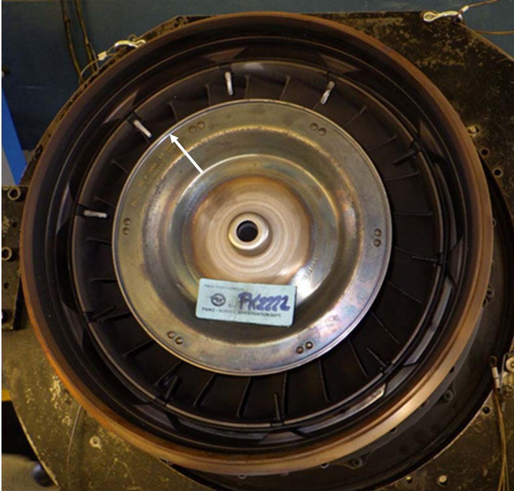
Figure 57. Upstream face of S1 PT guide vane ring and interstage baffle showing shroud edge scoring
