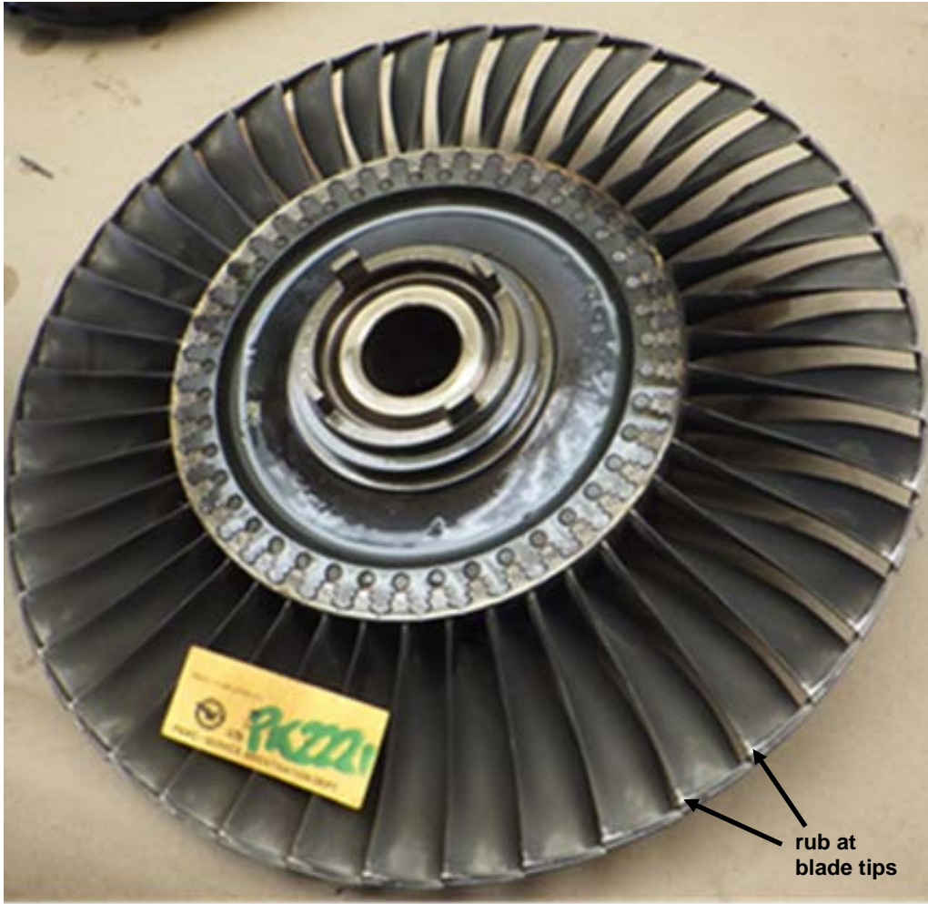
Figure 45. S2 PT disk assembly upstream face showing 360° blade tip rub
