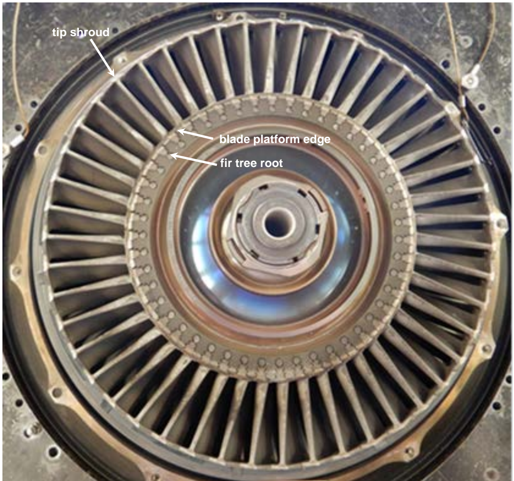
Figure 43. Upstream face of S1 PT disk assembly showing 360° scoring along the fir tree roots and blade platform edges, and at the blade tip shrouds
