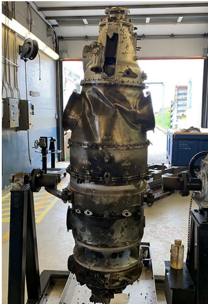
Figure 33. Bottom view of engine showing distortion
