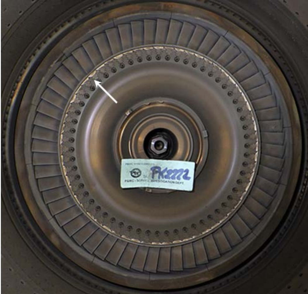
Figure 56. CT disk assembly downstream face showing 360° scoring in the fir tree root area
