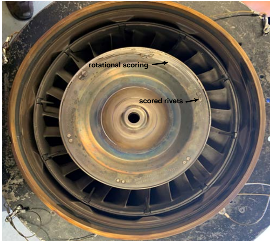
Figure 40. Upstream face of S1 PT guide vane ring and interstage baffle showing 360° scoring/material loss across retaining rivets
