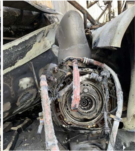
Figure 14. Right engine, showing A-flange separation
