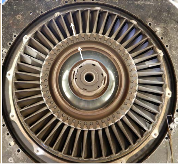
Figure 59. Rotational scoring S1 PT disk upstream face
