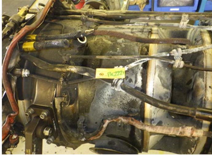
Figure 32. Typical left engine thermal damage
