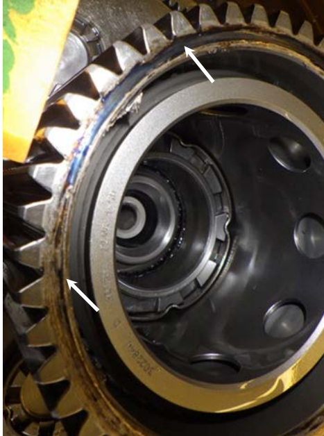
Figure 47. S2 sun gear showing scoring damage
