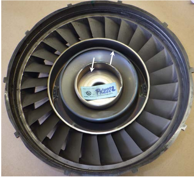
Figure 58. Scoring on downstream face of S1 PT guide vane ring and interstage baffle
