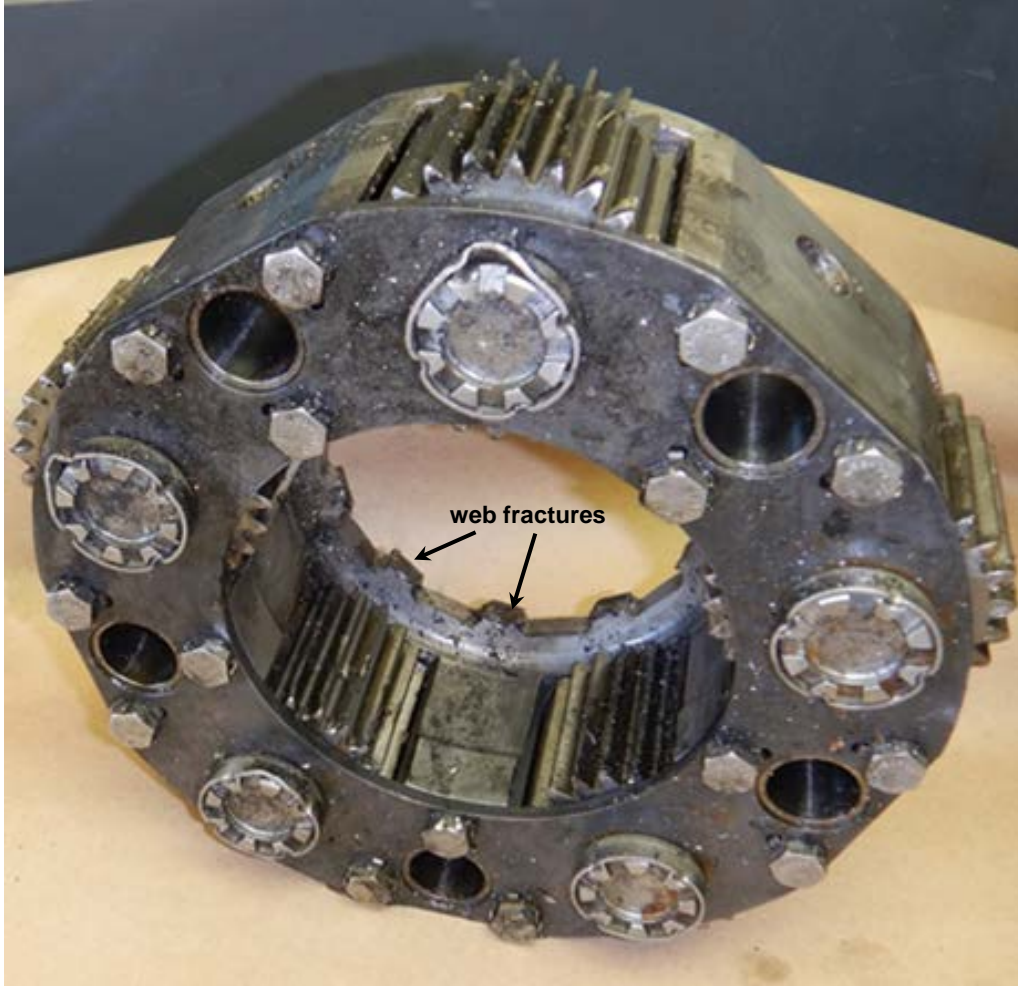
Figure 53. Liberated S2 planet gear carrier with several of the 10 web fractures noted
