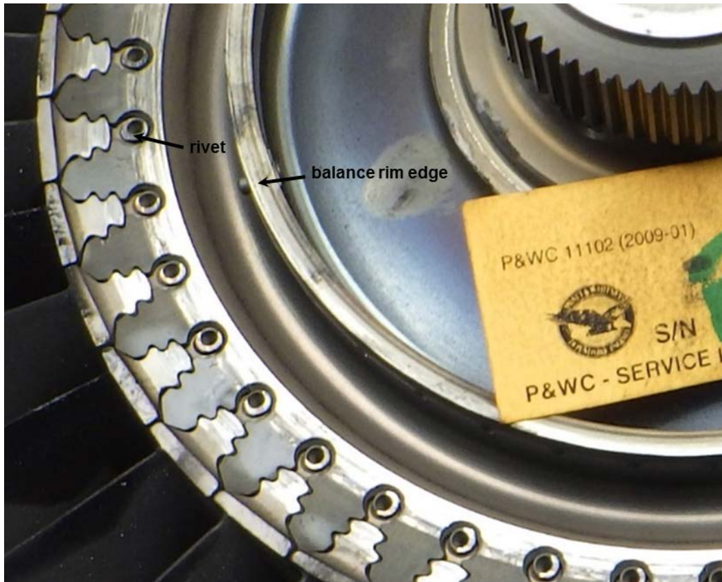
Figure 46. S2 PT disk assembly downstream face showing 360° scoring along retaining rivets and edge of balance rim
