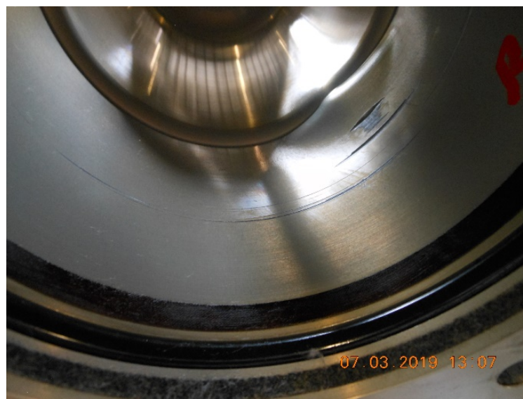
Figure 25. Internal piston impact marks
