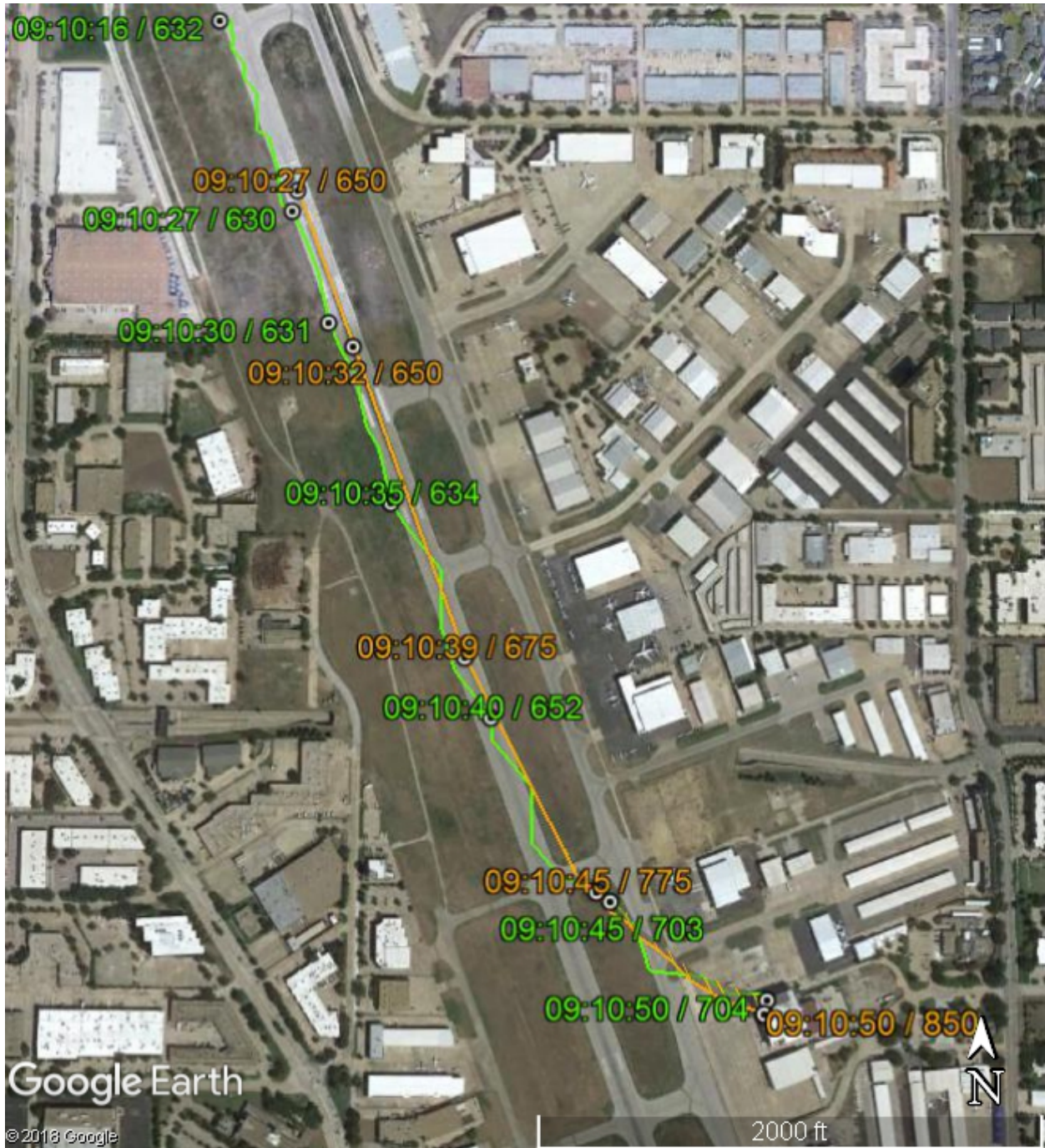
Figure 2. Accident flight with ADS-B data in orange and TAWS data in green.
