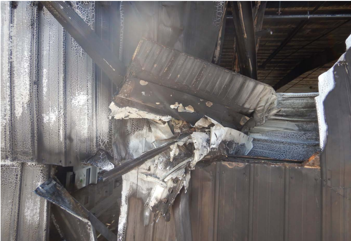
Figure 14 - Section of right wing found in hangar wall at initial impact point (Piece C).
