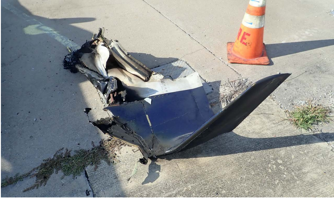
Figure 18 - Left wing tip section (Piece G), found outside hangar on the ramp area.
