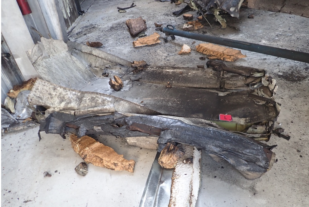
Figure 17 - Portion of Left Wing (Piece F), as found in the hangar, below the initial impact point.
