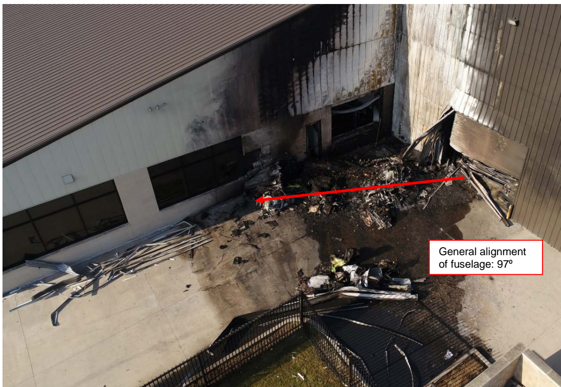
Figure 11 – Orientation and location of main wreckage area
