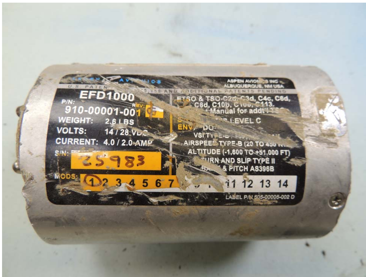
Figure 1. Photo of damage to EFD 1000
