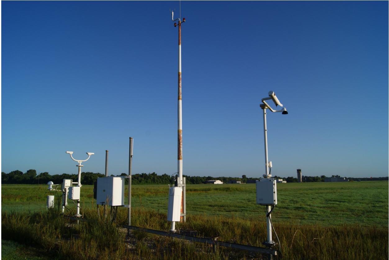
Figure 9 – SGR ASOS equipment and air traffic control tower
