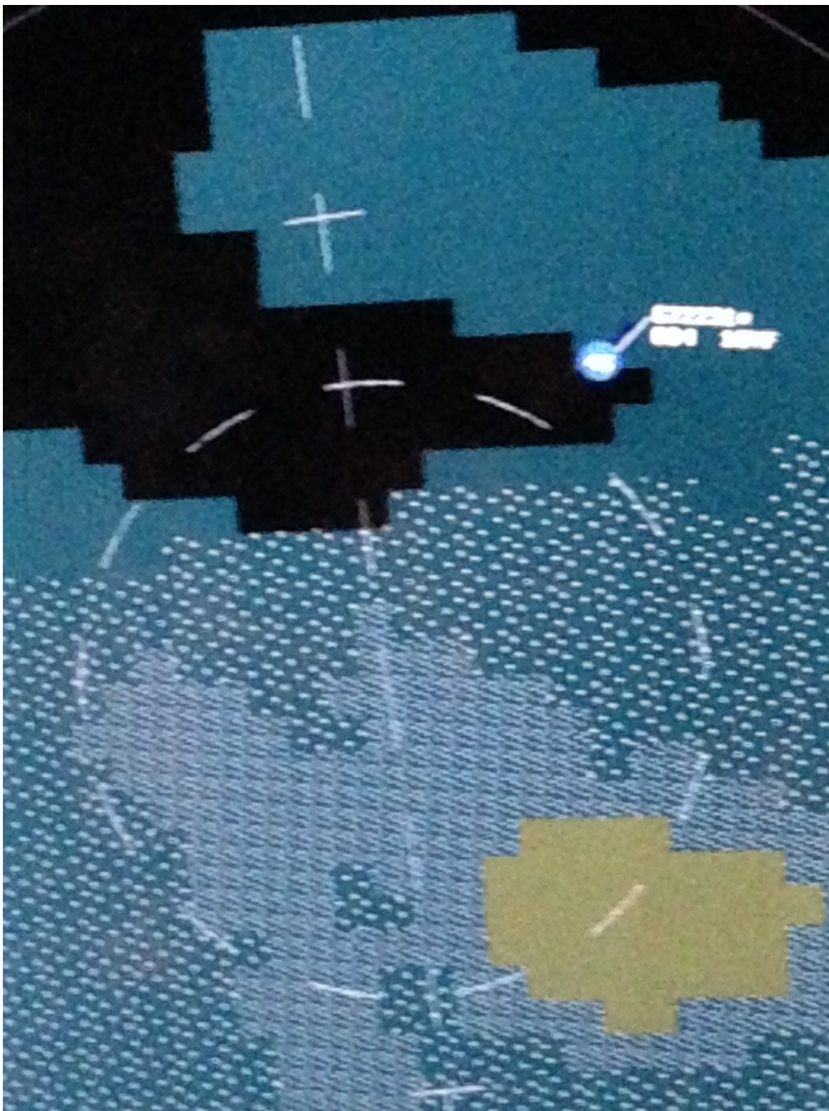
Figure 35 – STARS weather and precipitation level display used and seen by accident controller from 1506 CDT with SGR in the middle of the image
