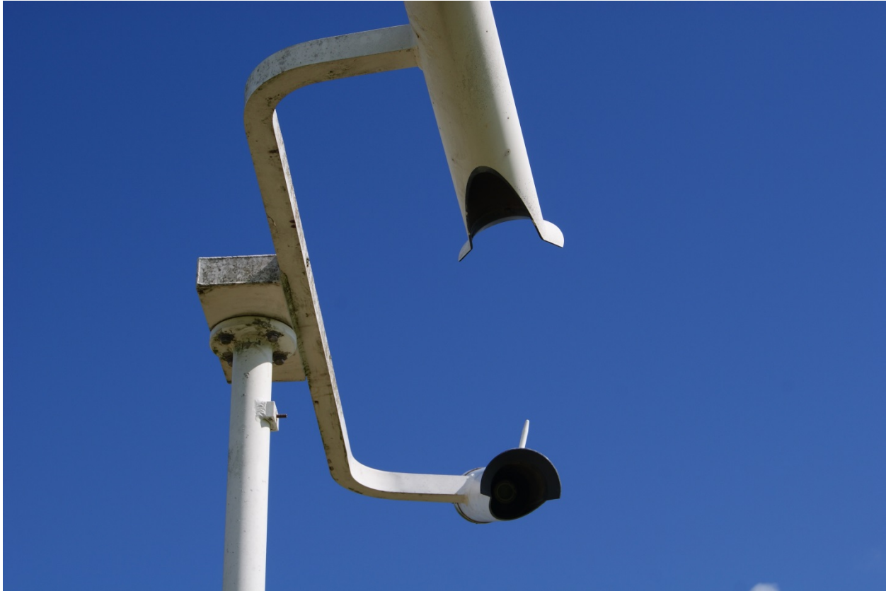
Figure 10 – SGR ASOS visibility equipment
