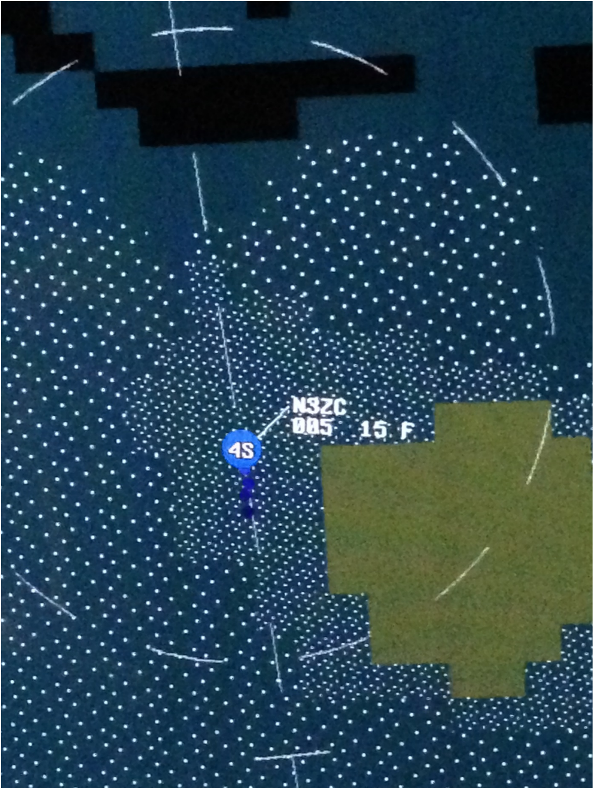
Figure 31 – STARS weather and precipitation level display used and seen by accident controller from 1458 CDT with SGR in the middle of the image
