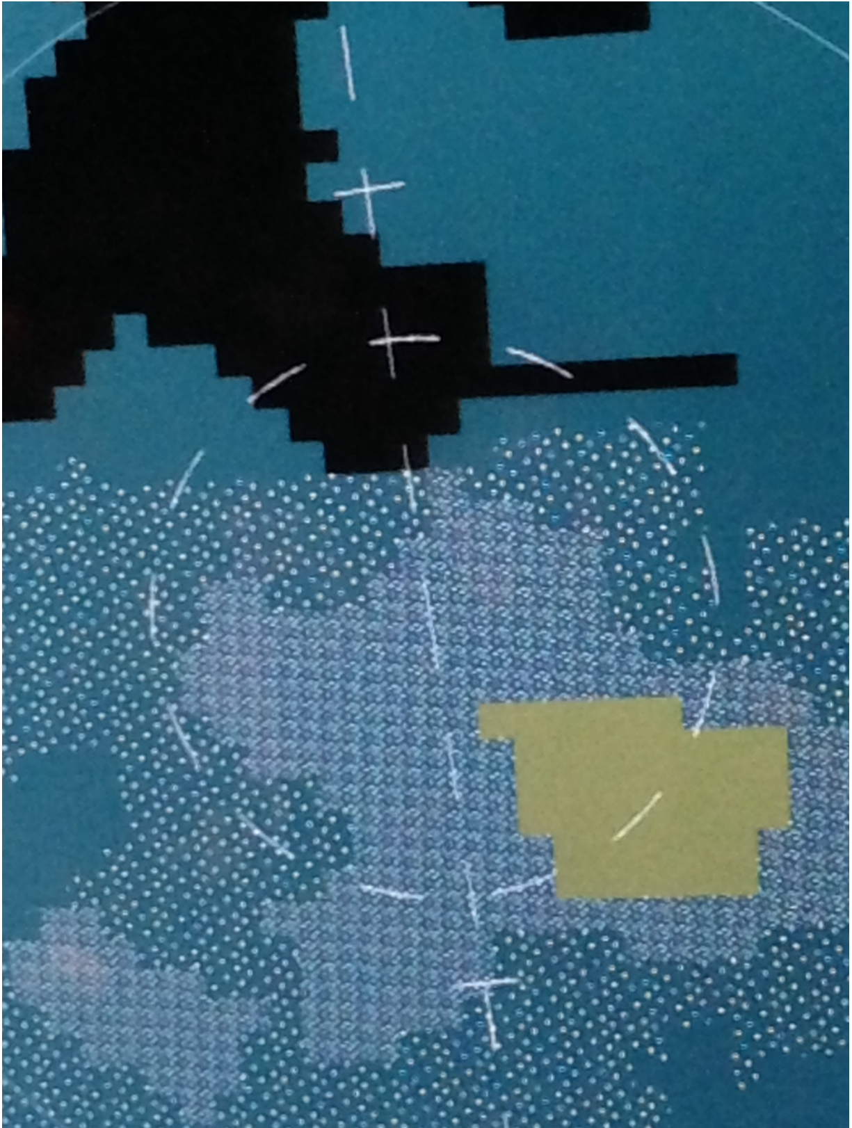
Figure 33 – STARS weather and precipitation level display used and seen by accident controller from 1502 CDT with SGR in the middle of the image
