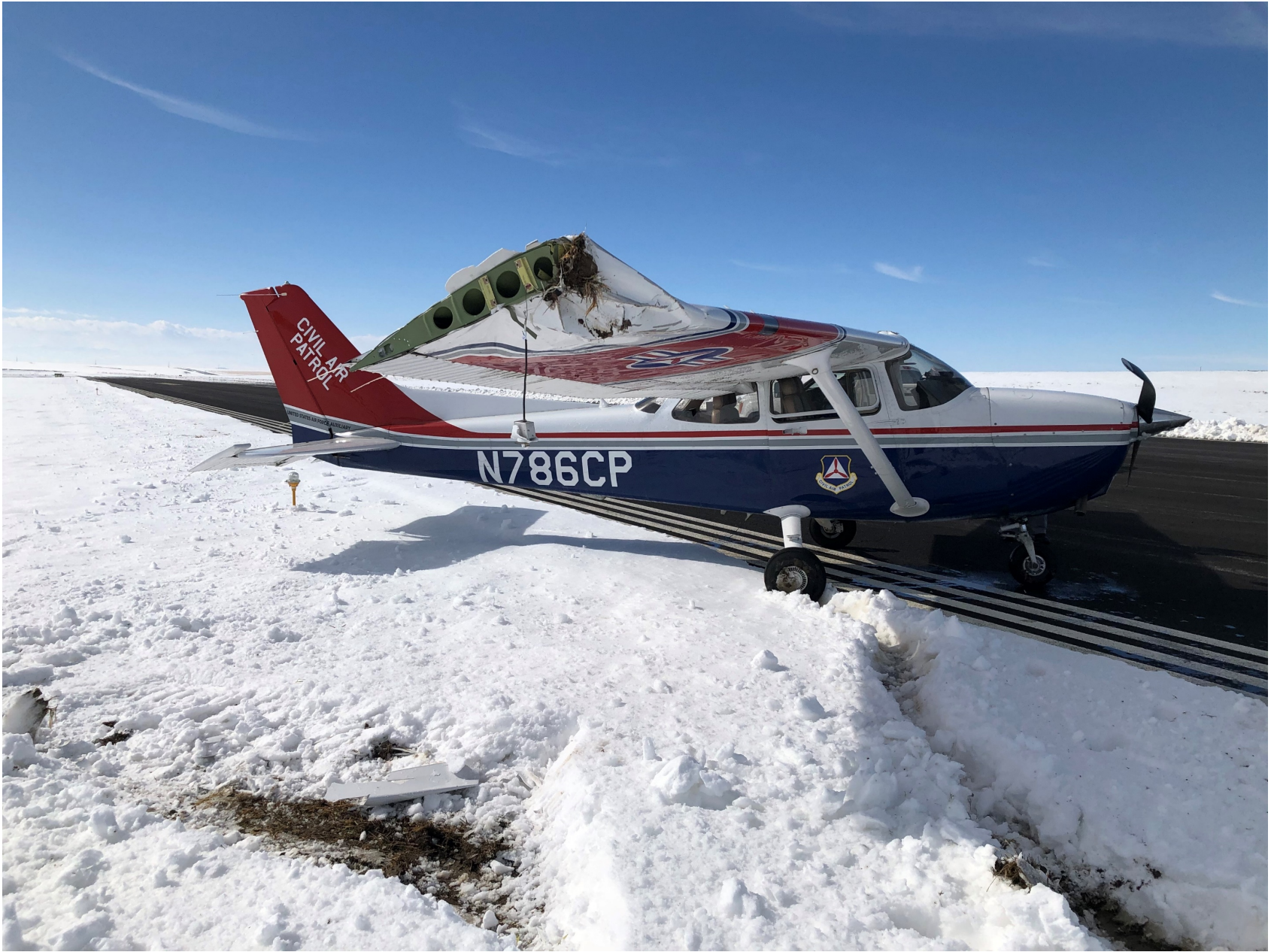
Photo 1 – Right Wing Damage
