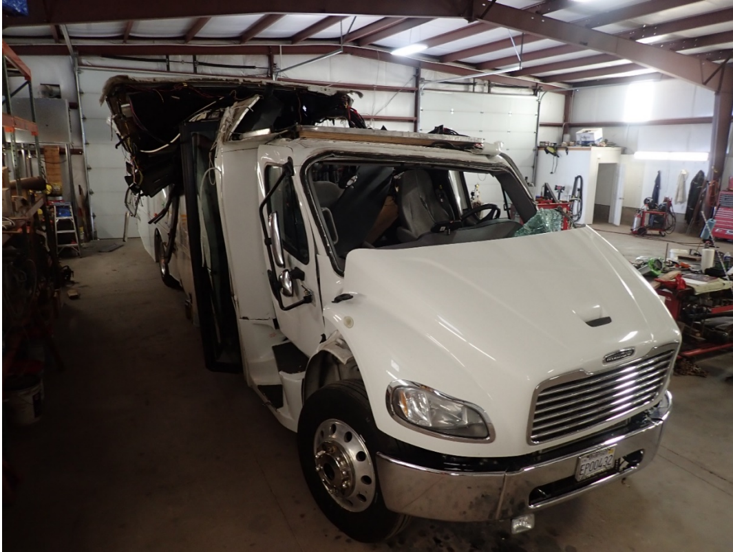
Figure 2: View of the damage and roof shift to the right side of the Freightliner
