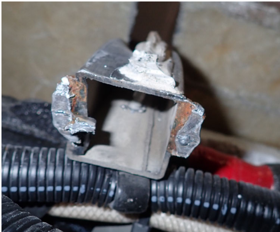
Figure 4: Separated roof bow with attached weld material.
