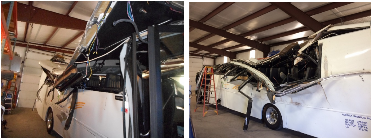
Figure 1. Right side view of roof crush and rollover damage. Figure 2. Left side view of damage to roof.
