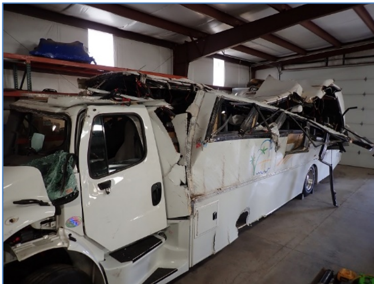
Figure 1. View of bus's left side showing roof damage.
