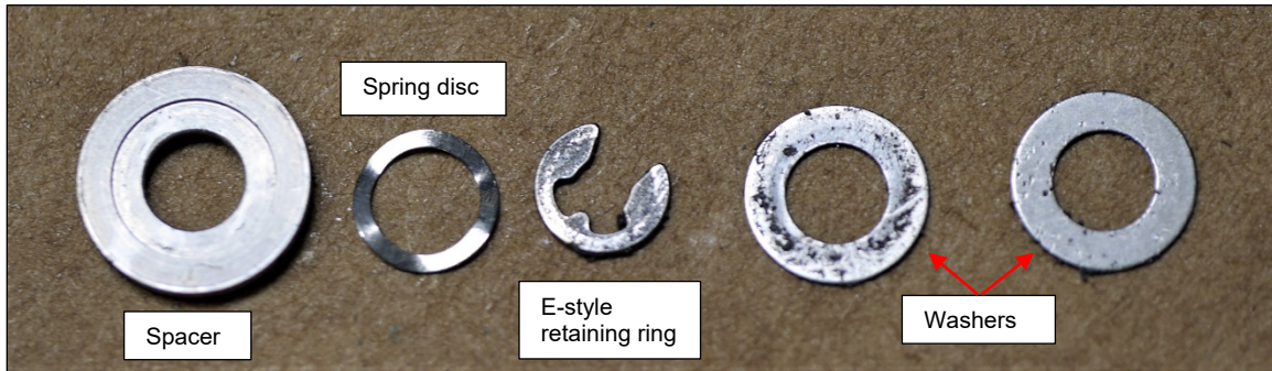
Figure 31: Component located between pinion gear and shaft.
