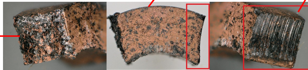
Broken end: 48% Cu / 52% graphite
