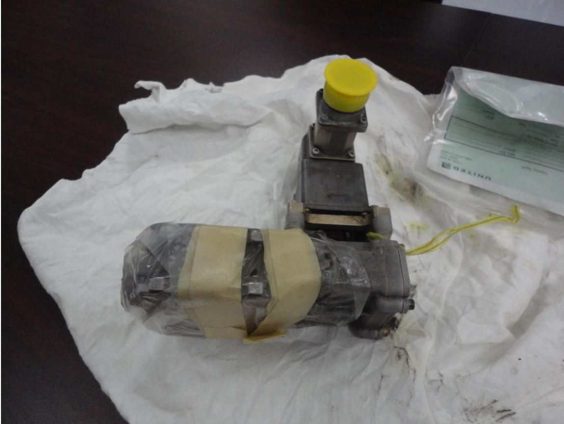
Figure 1 EDP supply shutoff valve – overall view
