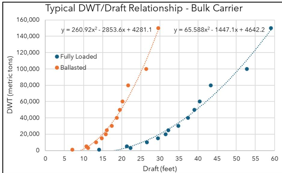
**Figure 44.** Plot of relationship between DWT to vessel draft for fully loaded and ballasted bulk carrier ships along with a best fit equation.
