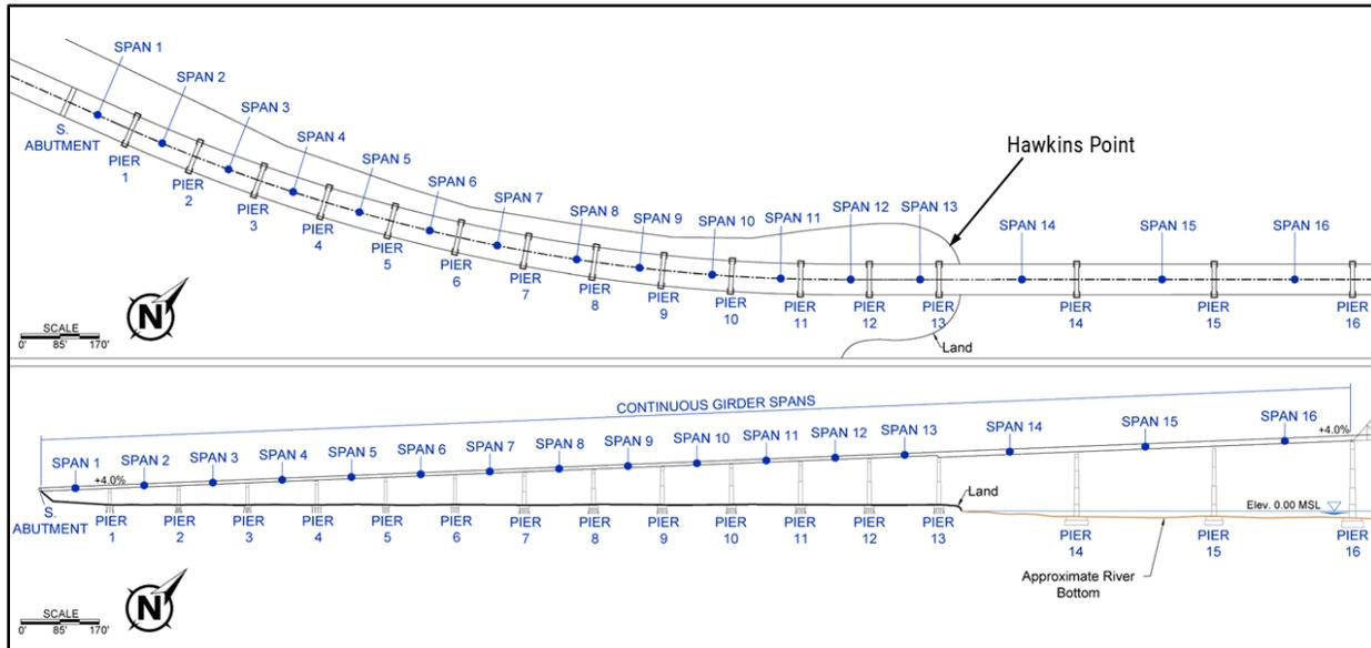
**Figure 17:** Plan (top) and elevation (bottom) views of the South Approach Spans of the Key Bridge.
