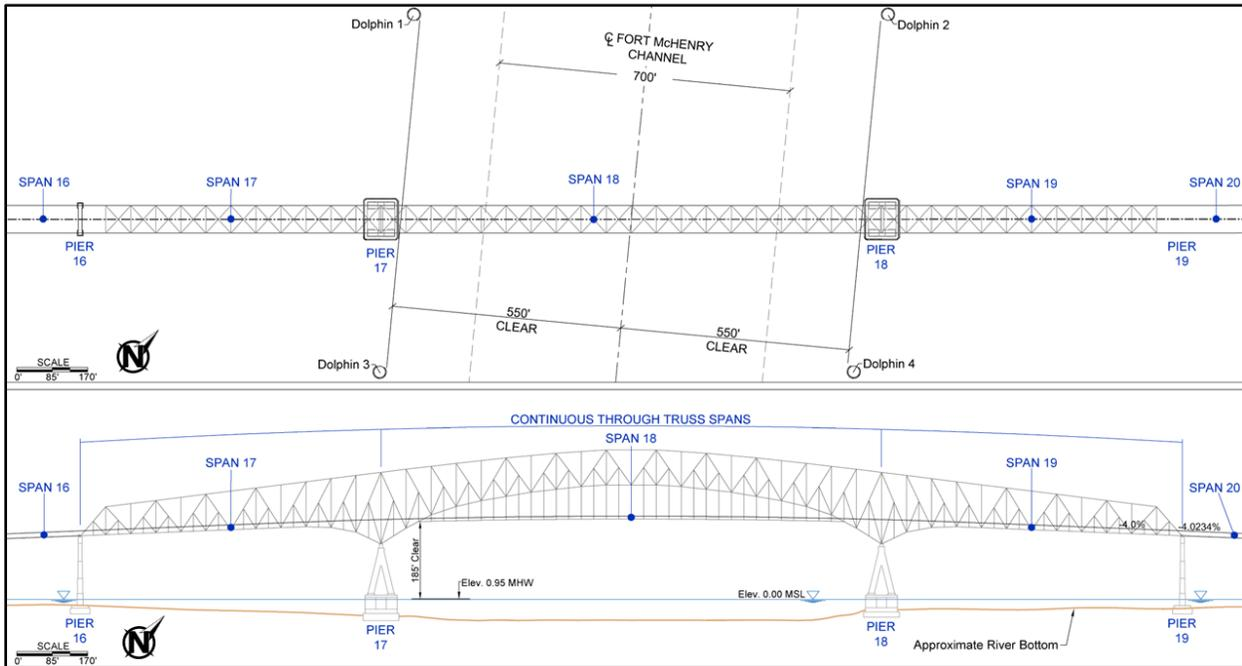
**Figure 18:** Plan (top) and elevation (bottom) views of the Main Spans of the Key Bridge.
