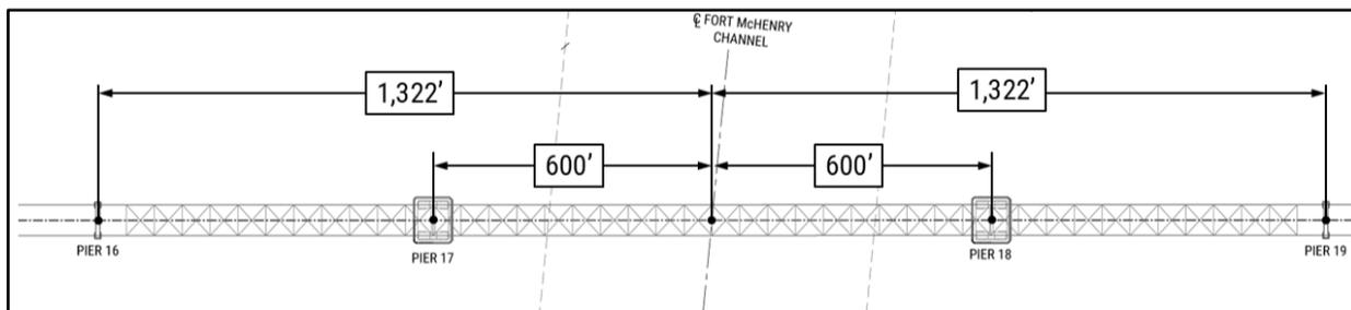
**Figure 51.** Distances between centerlines of the channel and analyzed piers.
