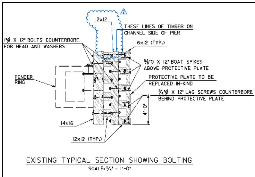
**Figure 14.** Typical section view of the fender system at Pier 17 and Pier 18 (source: MDTA)
