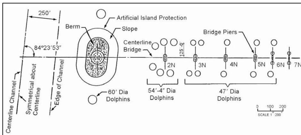
**Figure 64:** Dolphin and Island Protection System Plan for the Sunshine Skyway Bridge, Tampa Bay, FL (source: AASHTO).
