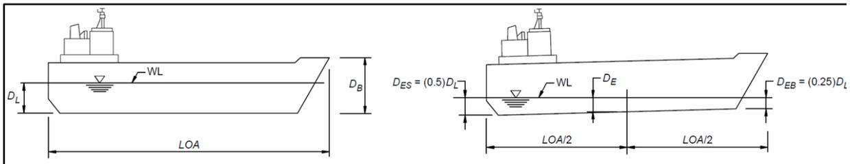
**Figure 42.** Vessel profiles of a loaded vessel (left) and ballasted vessel (right) (source: AASHTO)
