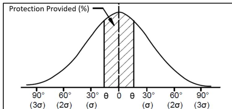
**Figure 54.** Normal distribution of vessel collision trajectories around a bridge pier (source: AASHTO)
