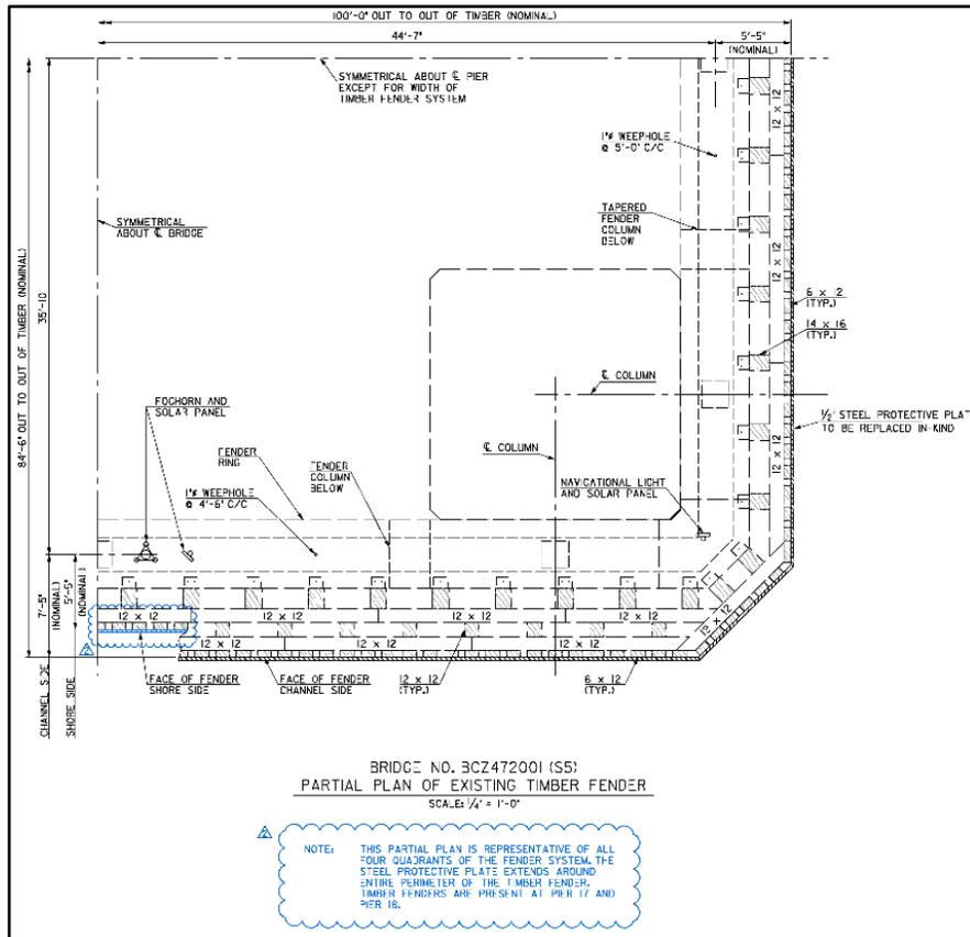
**Figure 13.** Partial plan view of fender system at Pier 17 and Pier 18 (source: MDTA).
