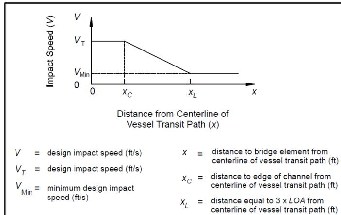
**Figure 52.** Triangular distribution used to calculate impact speed.
