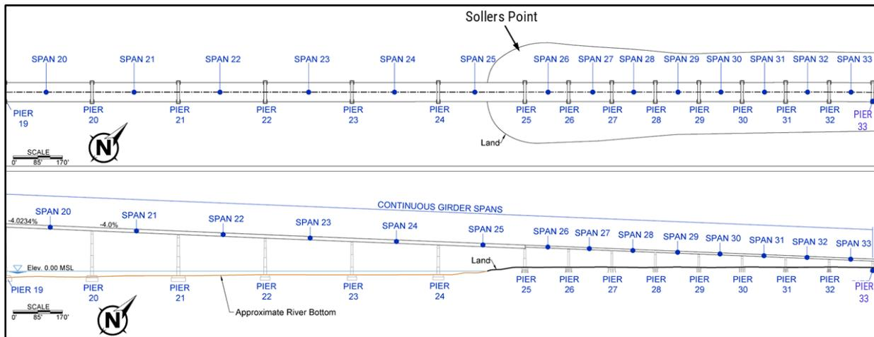
**Figure 19:** Plan (top) and elevation (bottom) views of the End Approach Spans of the Key Bridge.
