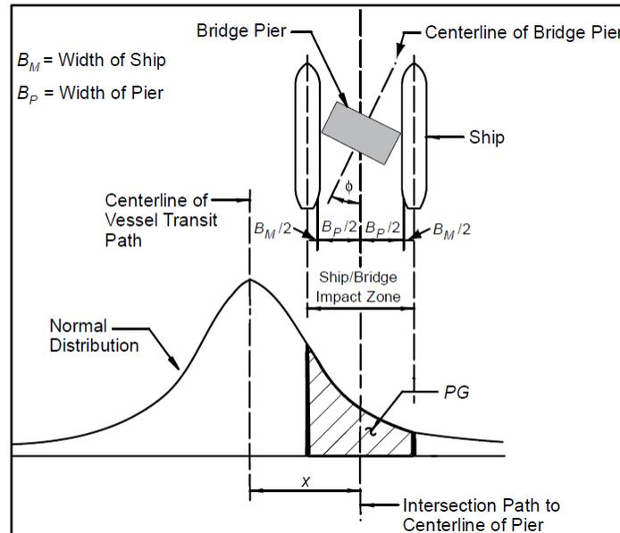
**Figure 50.** Parameters necessary to determine the geometric probability.
