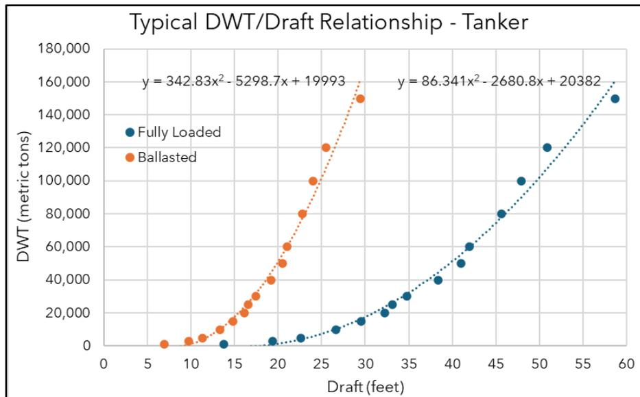
**Figure 45.** Plot of relationship between DWT to vessel draft for fully loaded and ballasted tanker ships along with a best fit equation.
