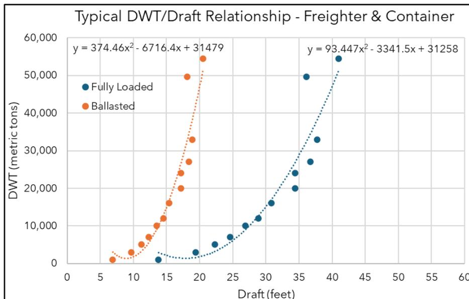
**Figure 43.** Plot of relationship between DWT to vessel draft for fully loaded and ballasted freighter/container ships along with a best fit equation.
