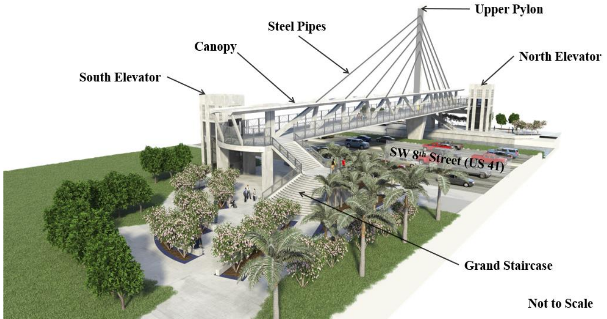
Figure 6 – Rendering of what the signature pedestrian bridge would look like when completed looking to the northwest (Source: FIU modified)
