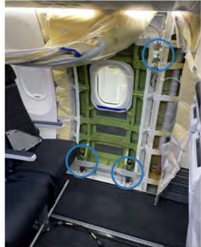
Figure 16. Photo showing the left MED plug immediately before interior restoration and the circles show the three locations without the retaining bolts, two vertical movement arrestor
