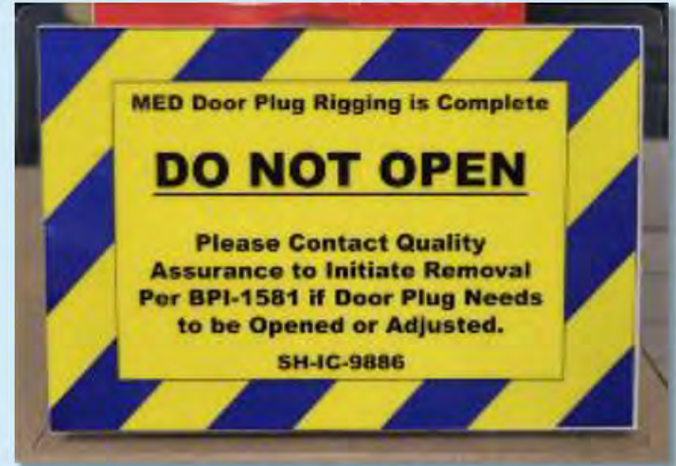
Sign placed on Mid-Exit Door (MED) plug in the factory
