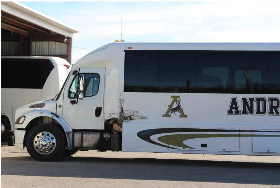
Figure 9. View of damage to left forward edge of the bus body.
