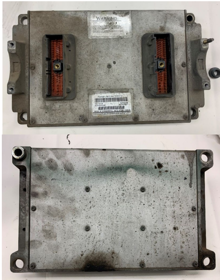
Figure 1. Front and back of DDEC V as received.
