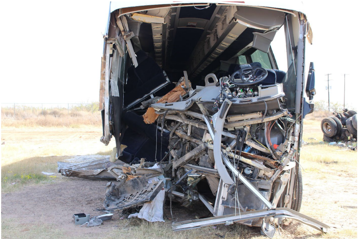
Figure 10. View of frontal damage to the 2005 MCI motorcoach.
