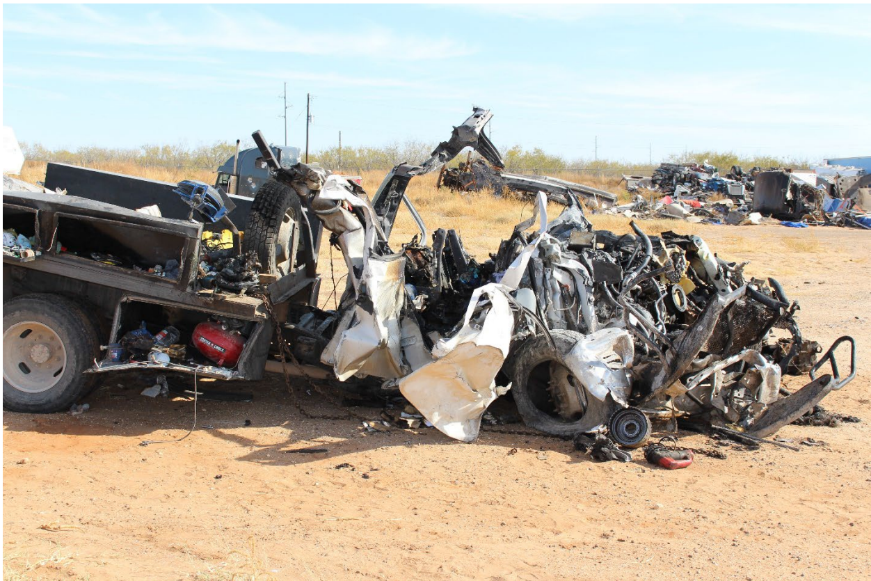
Figure 13. View of damage to the Ford F-350 pickup truck.
