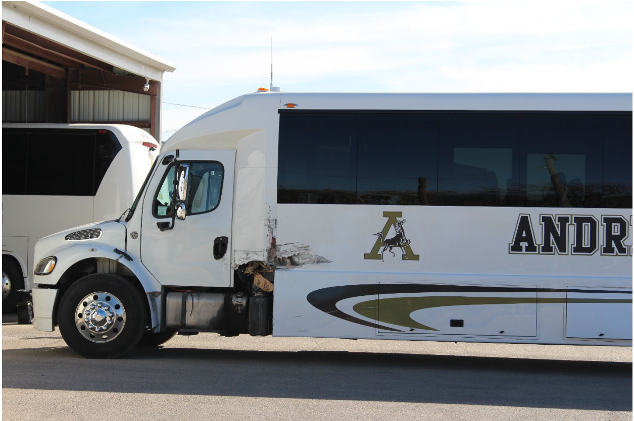
Figure 11. View of damage to left forward edge of the bus body.
