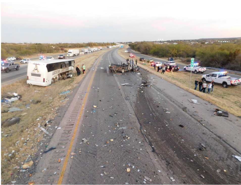
Figure 3. View of impact area near mile marker 179 with motorcoach at final position in the median and the pickup in the right-hand eastbound traffic lane.
