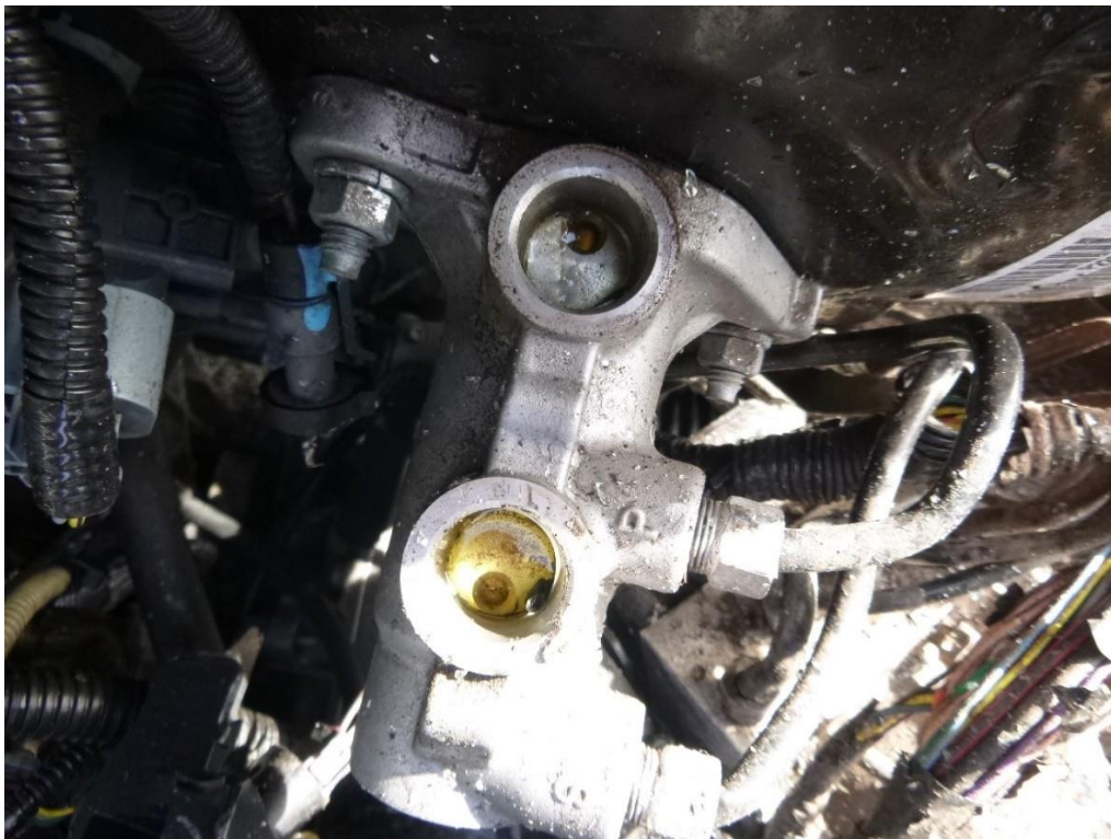
Photograph 8 - Depicting the damage to the master cylinder on the 2015 Chevrolet Equinox.
