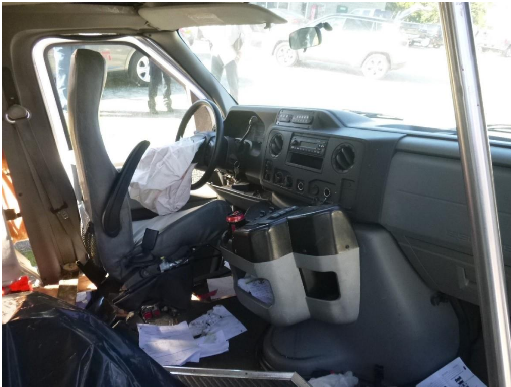
Photograph 1 – View of the 2009 Goshen Coach medium-size bus drivers' compartment depicting driver controls and deployed airbag.
