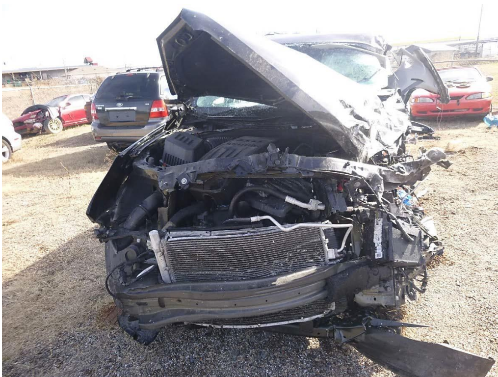
Photograph 2 – Front view of the 2015 Chevrolet Equinox depicting collision damage.
