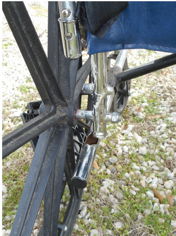
Photo 28 – View of separated weld on wheelchair cross member.
