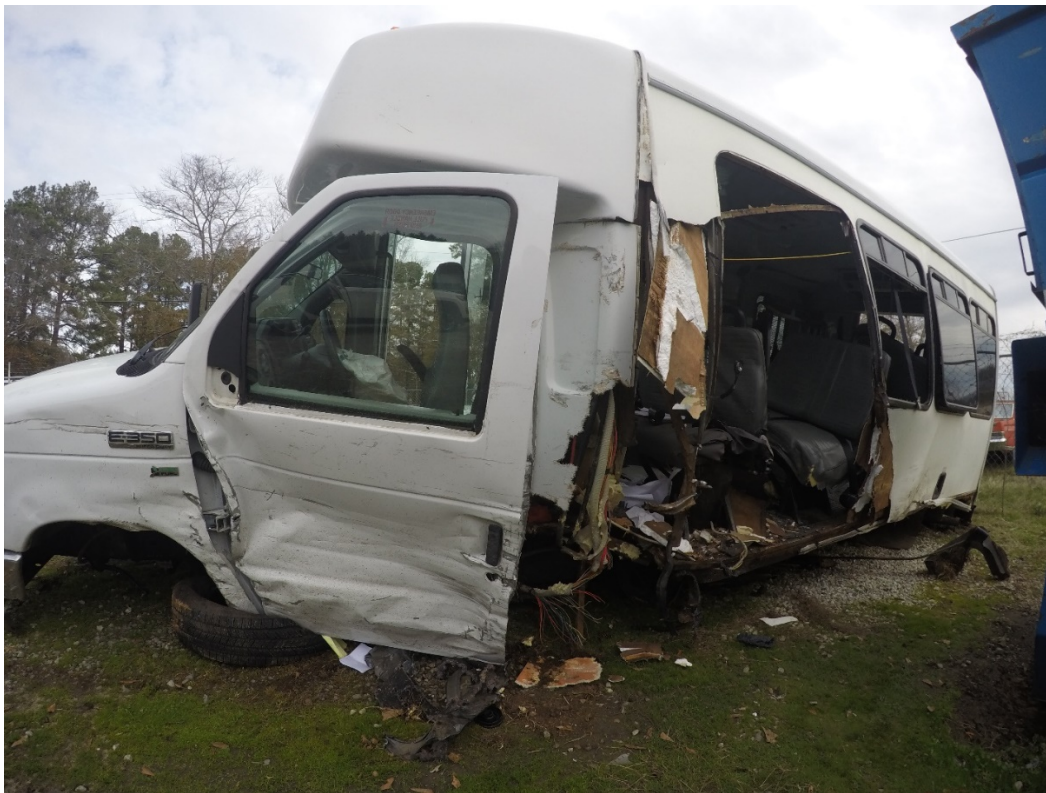
Figure 7. Wide-angle-lens photo of the crash-involved bus, with damage visible to the left side beginning at the front wheel.
