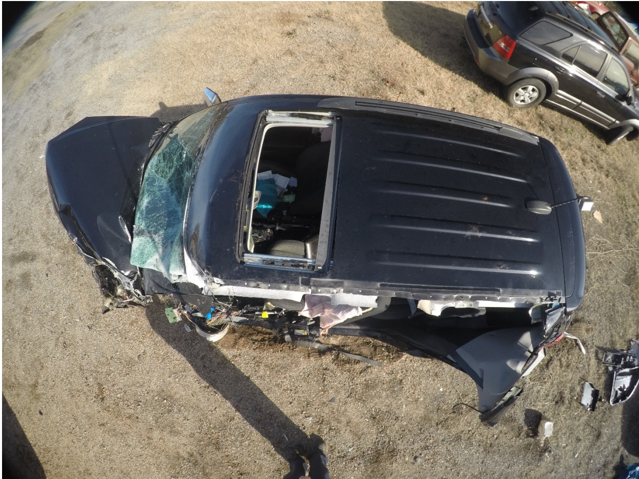
Figure 6. Top view of damaged SUV with open sunroof.
