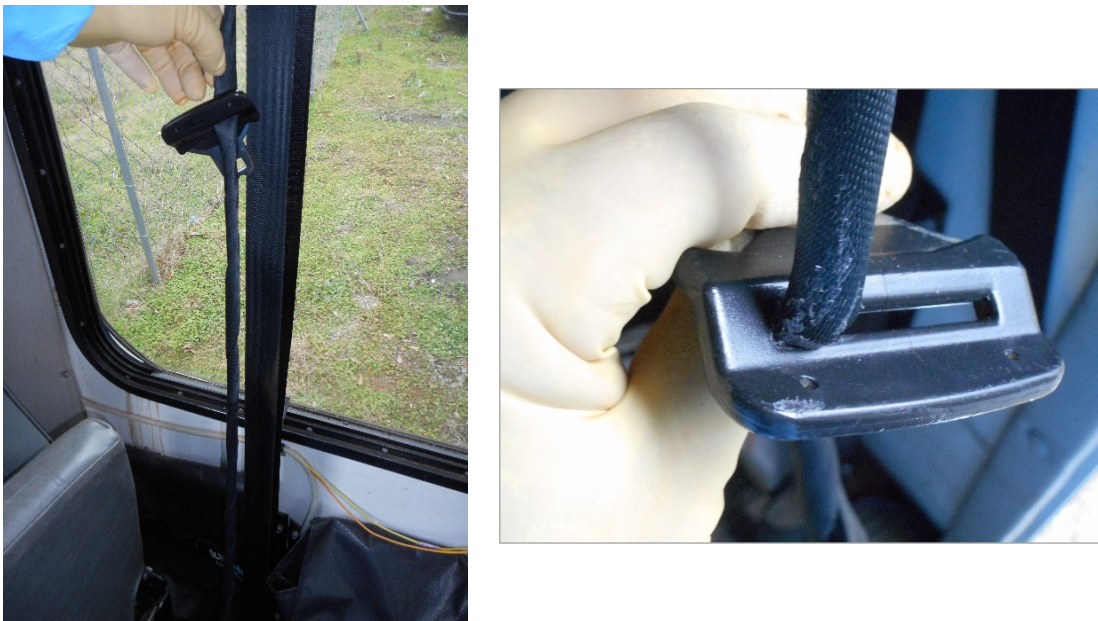
Figure 3. Lap/shoulder belts used to restrain the wheelchair occupants. Left, the twisted shoulder restraint for the wheelchair occupant on the left side of the bus. Right, close-up view of the shoulder restraint for the wheelchair occupant on the right side of the bus.
