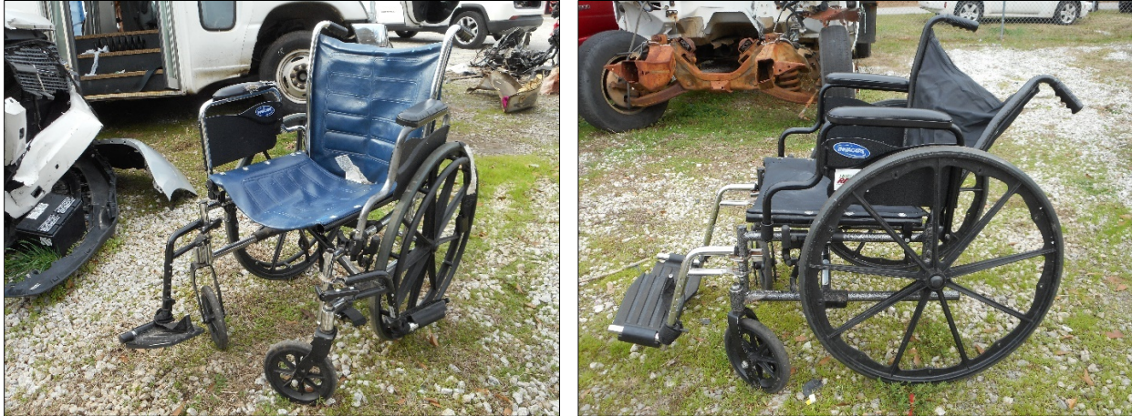
Figure 4. Wheelchairs damaged in the collision. Left, the wheelchair that was positioned on the bus's left side. Right, the wheelchair positioned on the bus's right side.
