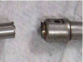
Depending on whether safety wire or a safety clip is used to secure the turnbuckle, any corrosion such as this may be hidden from view by the safety wire, which needs to be removed in order to perform an adequate inspection. The following photograph shows a typical safety wire configuration.
