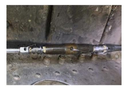
The following photograph shows a failure that occurred on a cable fitting located under a ventilation/heating duct on a Beechcraft Bonanza airplane.
