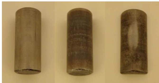
Figure 8. Control Set Roller, Lube Stain Roller, Rub Test
