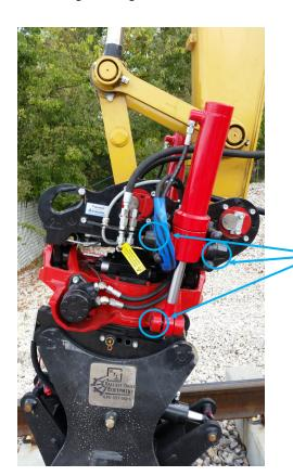
GREASE—2 lubrications points, On each side of RotoTils
