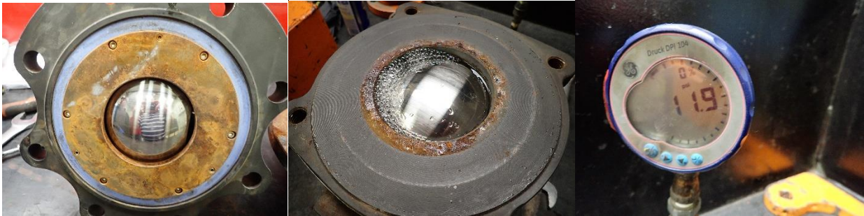
Gasket to car saddle intact. Valve started leaking at 11.9 psi
