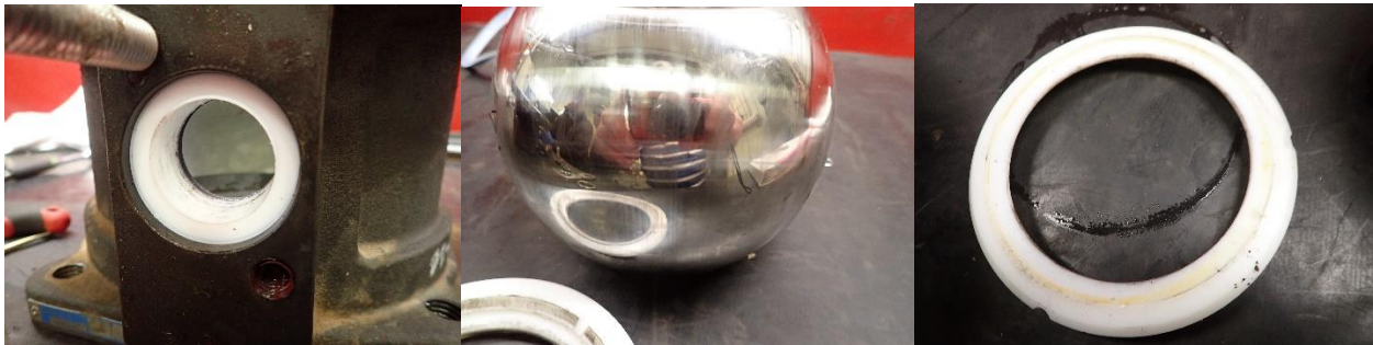
Stem and seat packing appearance is good.
