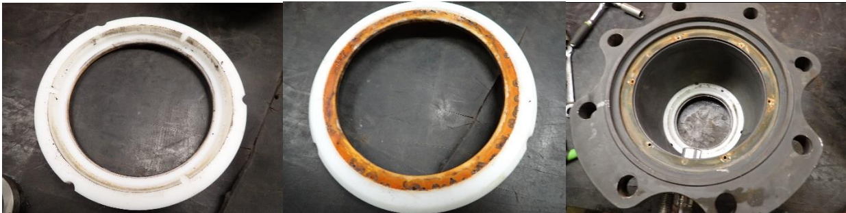
Seats intact and in original configuration.
