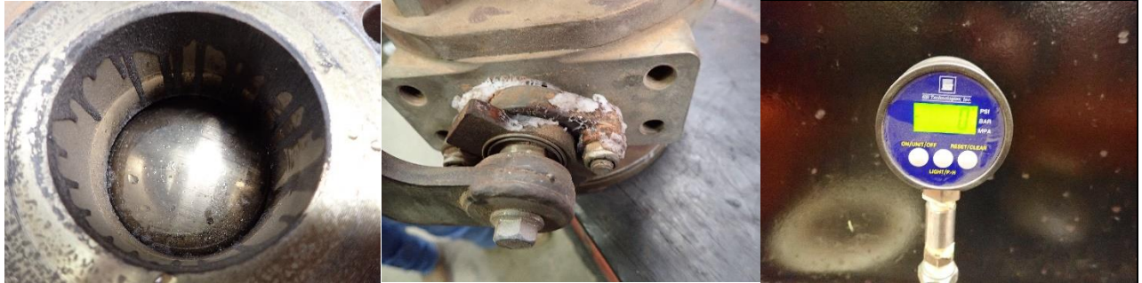
Valve would not hold pressure to test.
