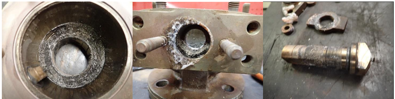
Seat residue in bottom of body. Stem packing residue in bottom 1/2.
