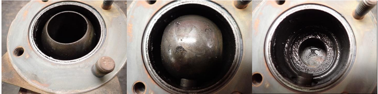
Only residue of seats remaining
