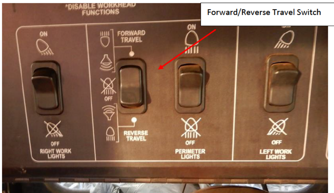
Figure 4. GS 15022 MCC with Forward/Reverse Travel Switch. Icons indicate the intended function of lights/alarms. (NTSB Photograph)
