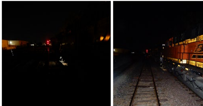
Figure 3 – Side by side comparison of view from the railcar that was being ridden by the Familiarizing Conductor and the fatally injured Conductor (TBOX 642811). Picture on left shows view with no lighting as probably seen by Conductor. Picture on right shows perspective when ambient lighting is provided. ( Photos courtesy of NTSB )
