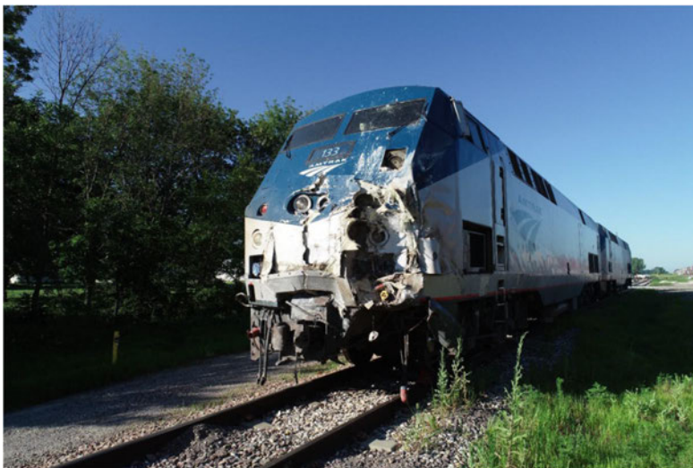
Figure 1 – Photo showing damage to lead locomotive ATK No. 133 ( Photo courtesy of NTSB Highway Factual Report )
