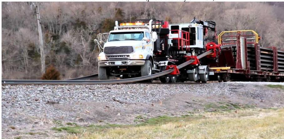
Photo below is a photo of the work train the day prior to the accident (June 4, 2019). The Rail Unloading Machine (RUM) truck is attached to the rear of the work train (photo courtesy of BNSF).
