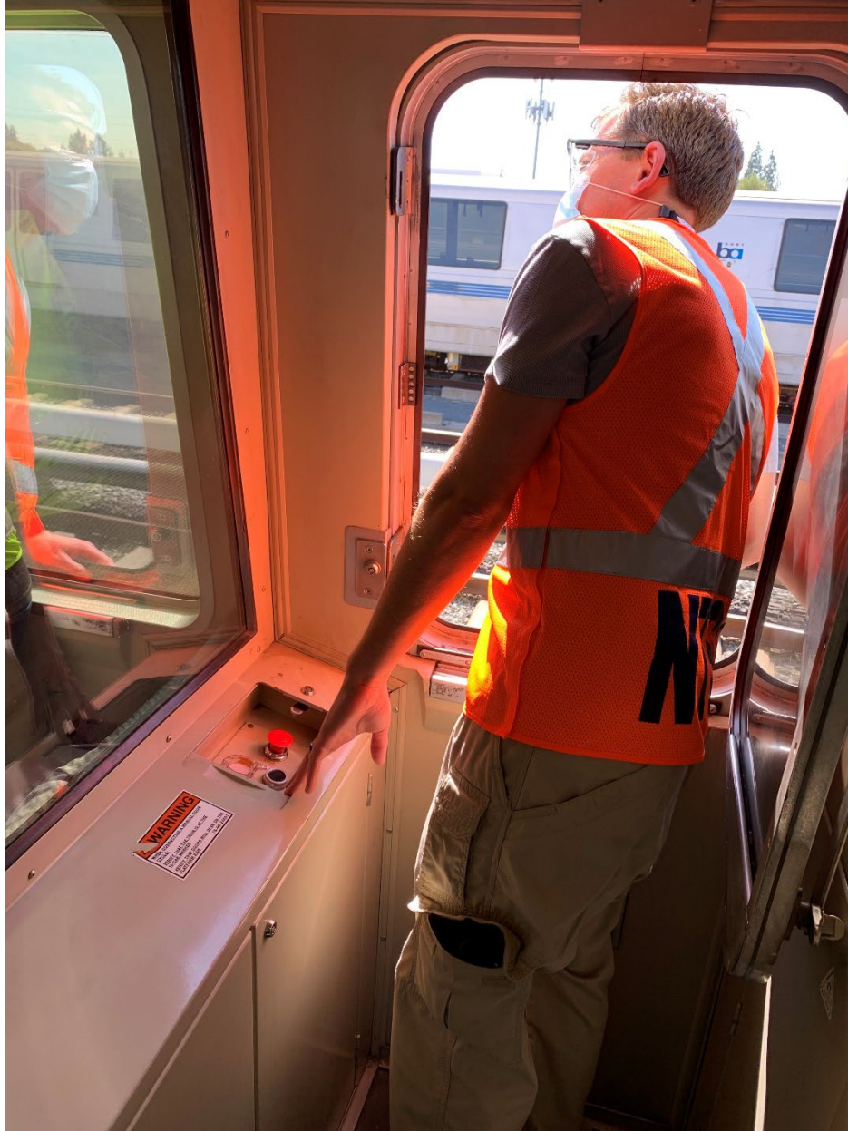
Figure 2: Investigator performing door cycling operations on accident train
