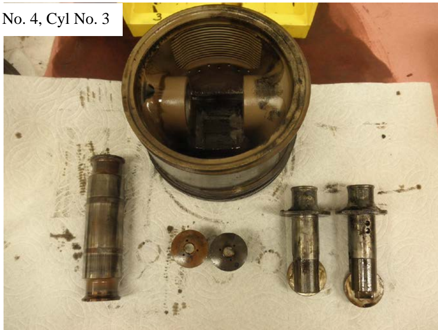
Photo No. 167: View of underside of No. 3 cylinder's piston along with the piston pin, piston pin buttons, and the cam followers showing all were intact and undamaged.
