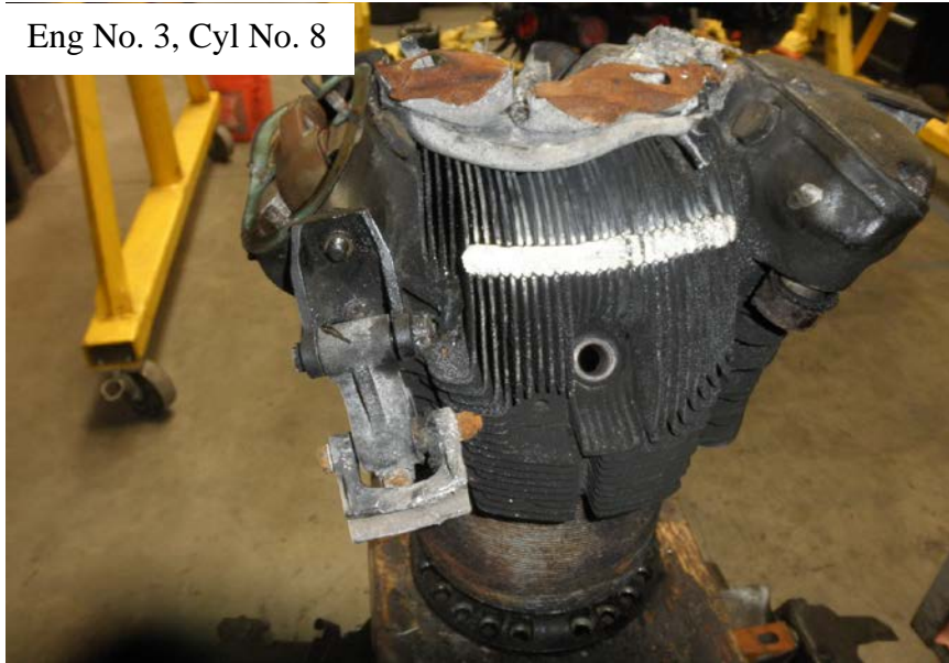
Photo No. 106: View of the front of No. 8 cylinder showing that it was intact with the head in place.
