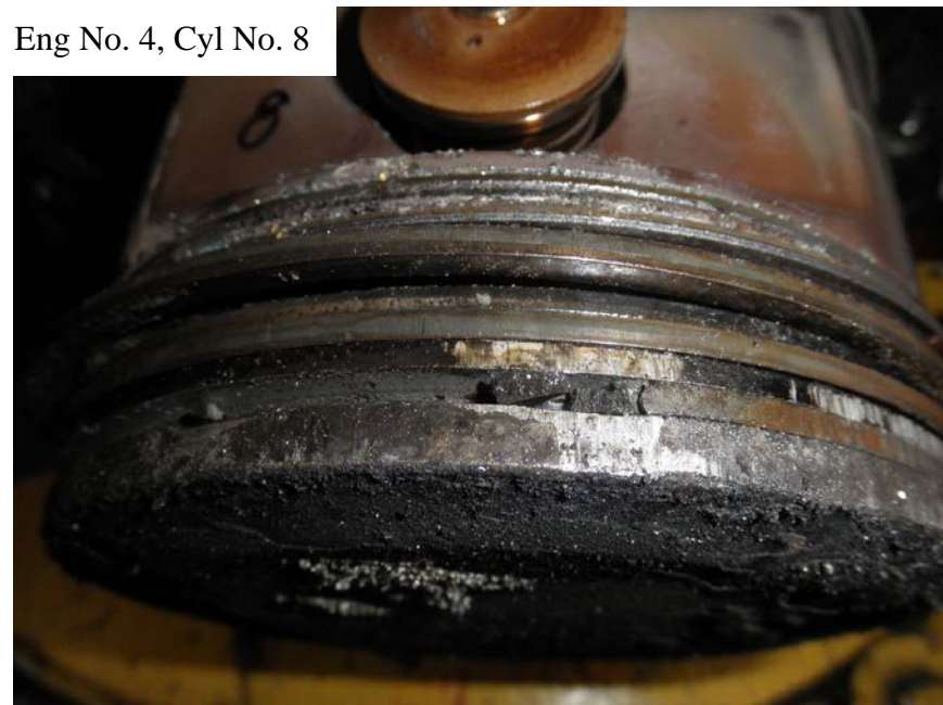
Photo No. 186: Close up No. 8 cylinder's piston showing broken No.1 piston ring.
