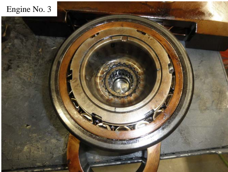
Photo No. 48: View of rear crank shaft bearing showing that it was intact and the rollers were in place.
