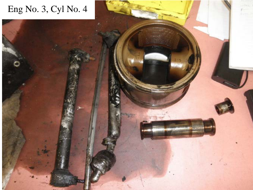
Photo No. 77: View of No. 4 cylinder's piston, wrist pin, push rod shrouds, and push rods.
