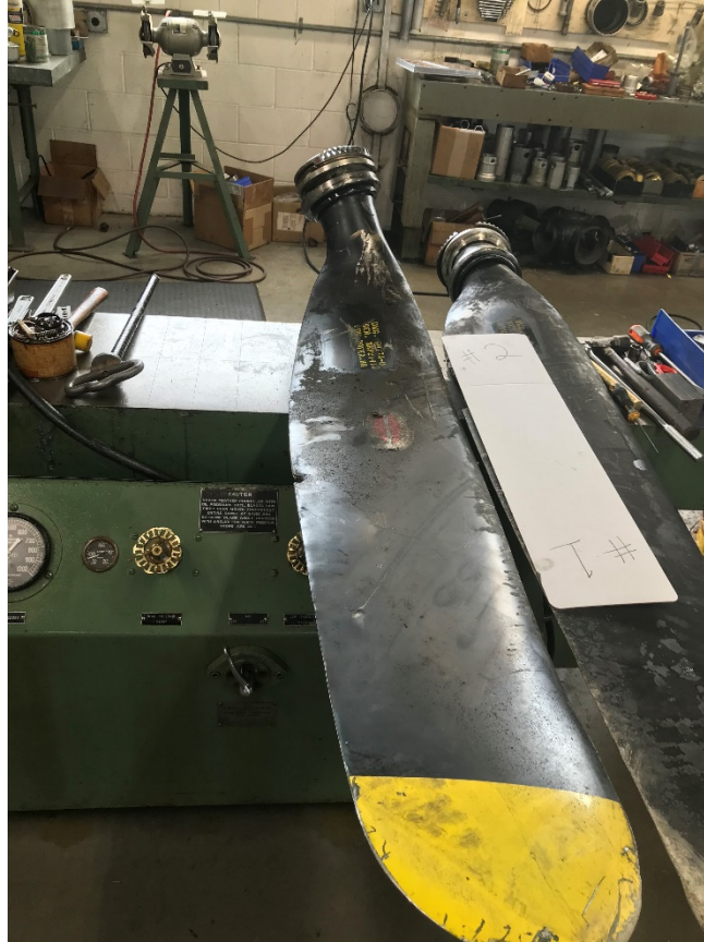
Photo No. 207: View of blade No. 2 camber side showing the blade full length and the bend as well as no thermal damage.
