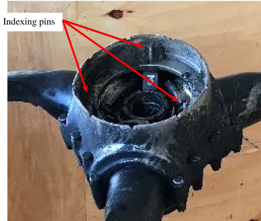
Photo No. 202: Enlarged view of propeller hub showing SB 473 three-pin configuration.
