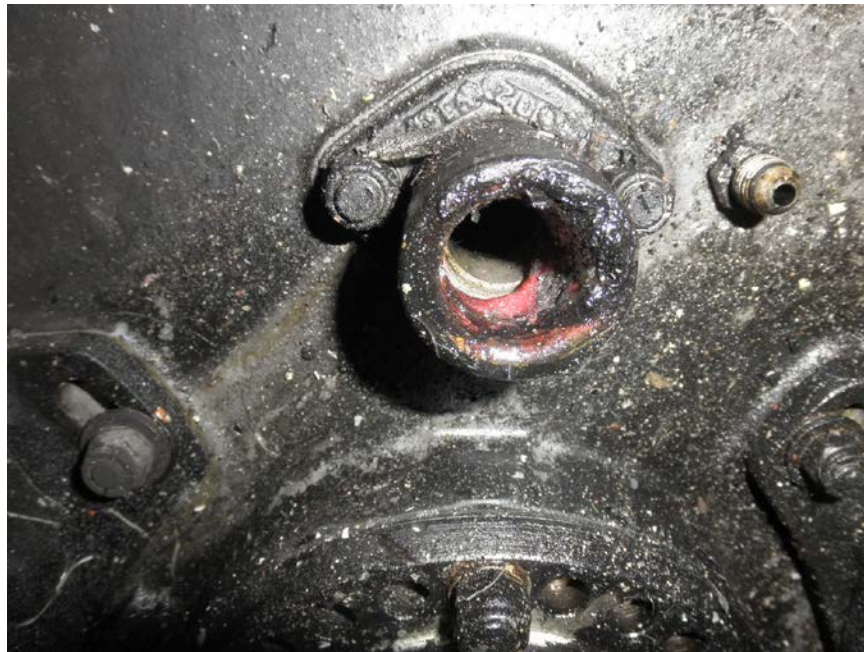
Photo No. 199: No. 4 engine's supercharger vent port with the remains of a plastic cap in the port.
