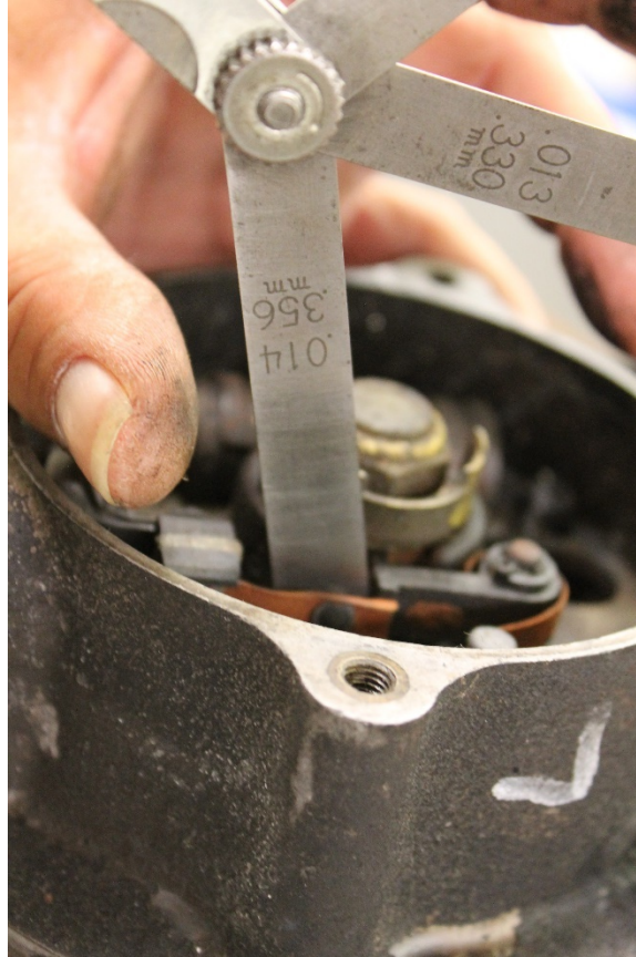
Photo No. 15: Close up view of left magneto's measured point gap of 0.014 inches. (S&T)
