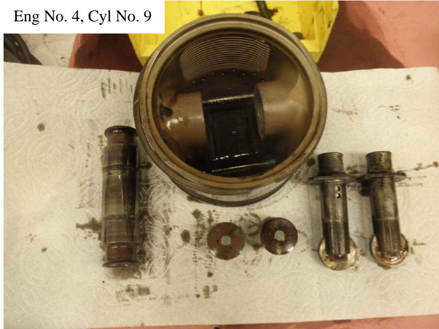
Photo No. 192: View of underside of No. 9 cylinder's piston along with the piston pin, piston pin buttons, and the cam followers showing all were intact and undamaged.
