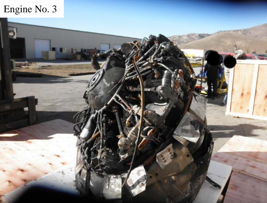
Photo No. 37: View of No. 3 engine after it was uncrated showing airframe structure still attached.
