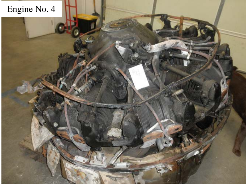
Photo No. 146: View of front of engine showing some airframe structure still attached.
