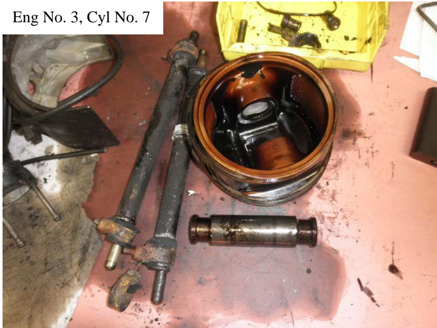
Photo No. 103: View of the underside of the No. 7 cylinder's piston, the piston ring, and push rod shrouds with push rods.
