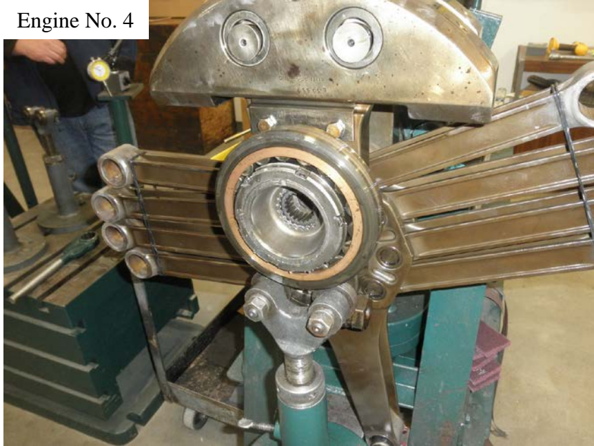
Photo No. 153: View of crank shaft rear bearing showing it was intact.
