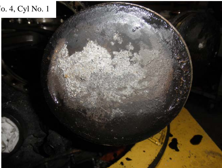
Photo No. 157: Close up view of the No. 1 cylinder's piston head showing the white-colored deposit.
