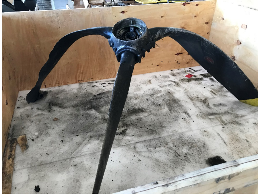
Photo No. 200: No. 3 propeller as received with all three blades in place, but with the dome separated from the spider hub.
