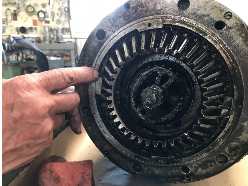
Photo No. 201: View of base of propeller dome showing gear was intact.
