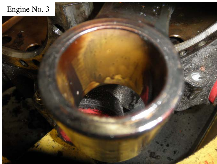
Photo No. 50: Close up of a typical articulating rod piston pin bearing surface showing that it was not damaged.
