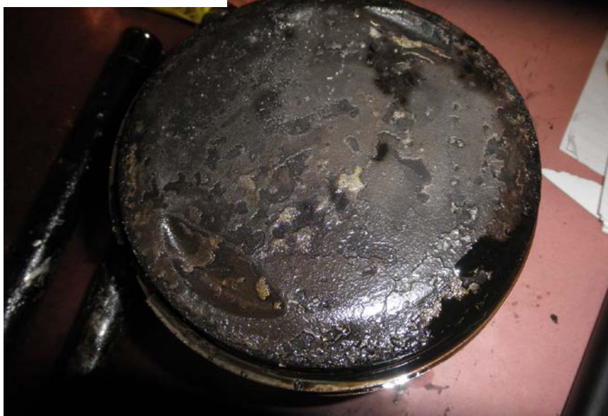
Photo No. 98: Close up view of the head of the No. 6 cylinder piston showing the dark gray color.
