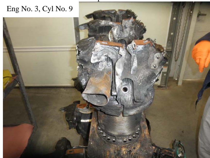
Photo No. 115: View of the rear of No. 9 cylinder showing that it was intact with the head in place. Also showing the broken exhaust rocker arm cover and the missing intake rocker arm cover.
