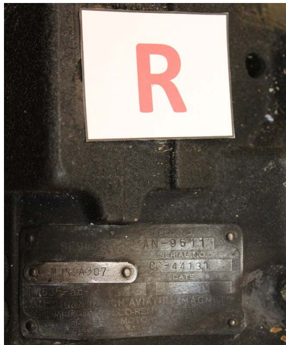
Photo No. 14: Right magneto's data plate. (S&T)
