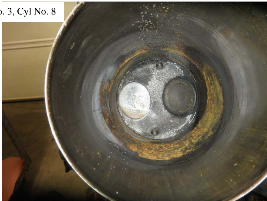
Photo No. 113: View inside of the No. 8 cylinder's barrel showing the metal fragments, but no damage to the barrel and that the two valves were in place in the closed position.
