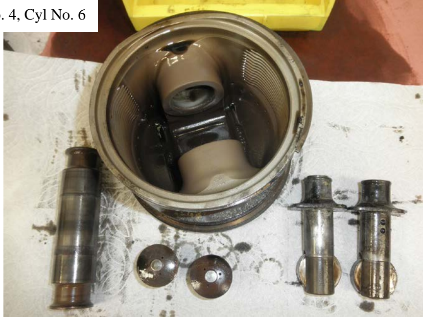
Photo No. 179: View of underside of No. 6 cylinder's piston along with the piston pin, piston pin buttons, and the cam followers showing all were intact and undamaged.
