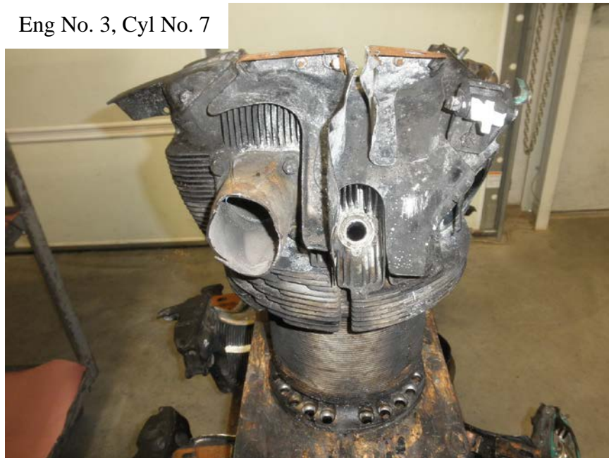
Photo No. 101: View of the rear of No. 7 cylinder showing that it was intact with the head in place.
