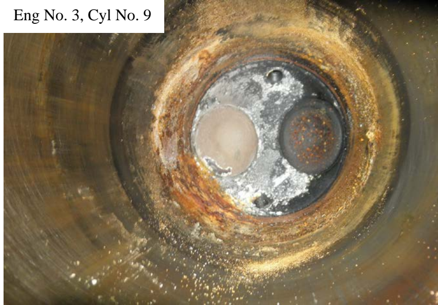
Photo No. 120: View inside of the No. 9 cylinder's barrel showing the corrosion and that the two valves were in place in the closed position.
