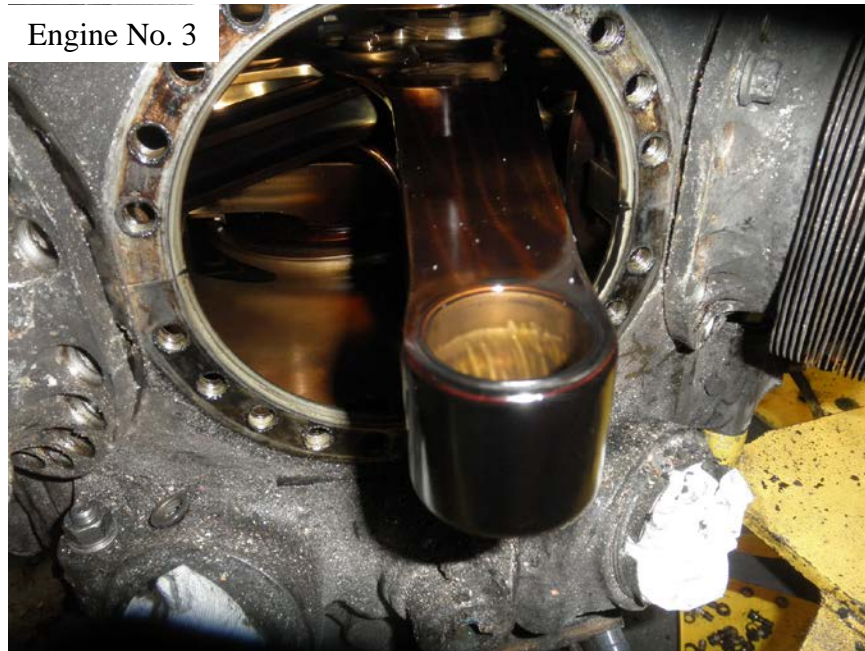
Photo No. 49: Close up view of the master rod piston pin bearing surface showing that it was not damaged.
