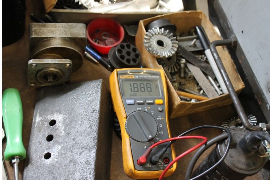
Photo No. 18: View of left magneto's multimeter reading of magnet's primary output of 1.888 amperes. (S&T)
