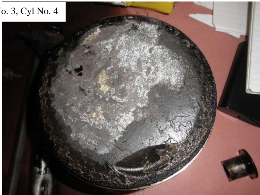
Photo No. 80: Close up view of the top of the No. 4 cylinder's piston showing areas of dark gray and white coloration that is indicative of detonation.
