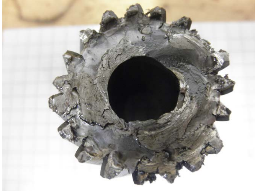
Photo No. 128: Close up view of fracture surface on aft end of accessory drive gear shaft.
