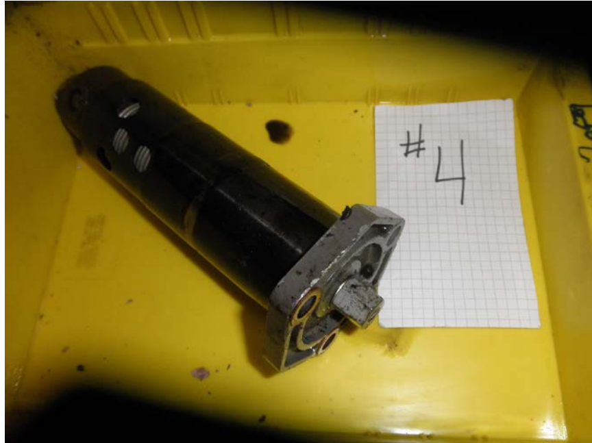
Photo No. 197: No. 4 engine's Cuno filter after it was removed from the engine.
