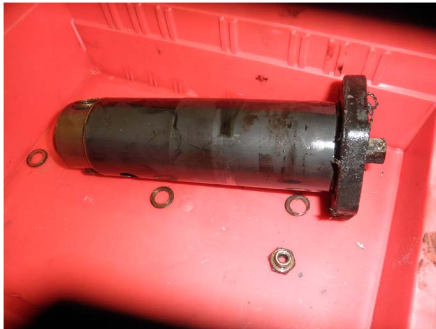
Photo No. 129: The No. 3 engine's Cuno oil filter after removal from the engine.
