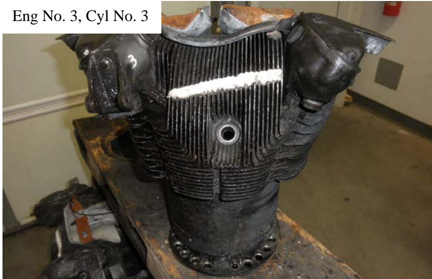
Photo No. 66: View of front of No. 3 cylinder showing it was intact with the head in place and intact, and the intake and exhaust rocker arm covers were in place.
