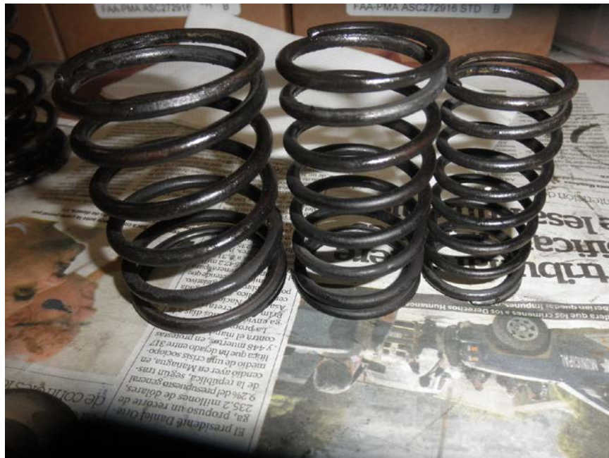
Photo No. 125: View of the three valve springs that should normally be installed in a R-1820 engine.
