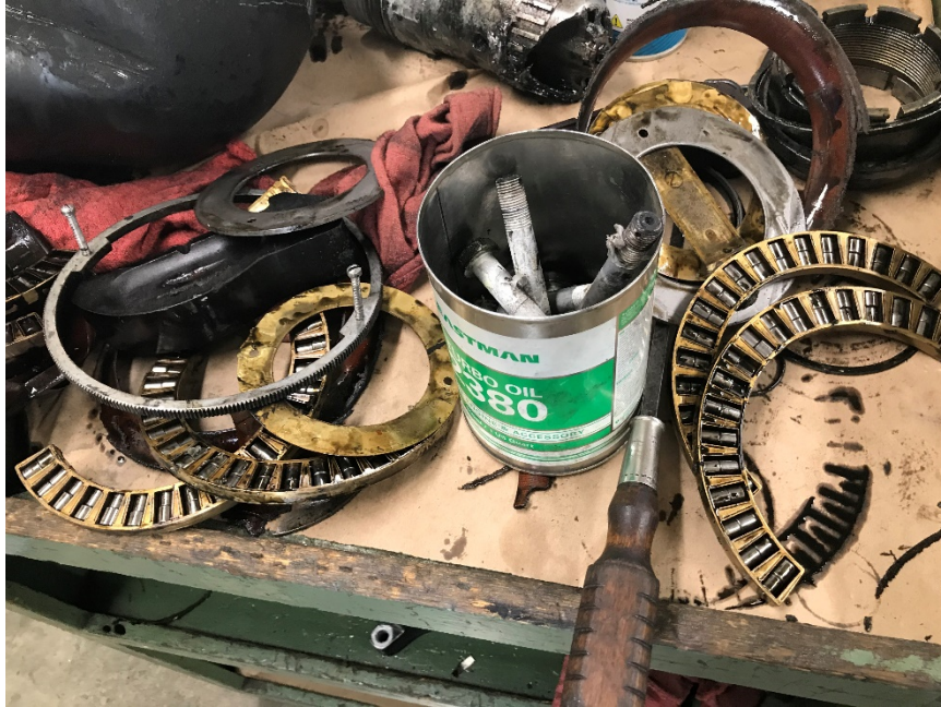
Photo No. 206: Picture of the propeller bearing segments showing they were intact with the rollers in place.
