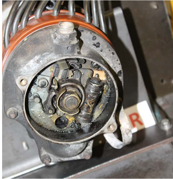
Photo No. 28: Right magneto installed on test bench. (S&T)
