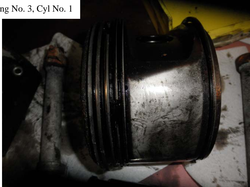
Photo No. 56: Close up view of side of No. 1 cylinder's piston showing the rings were in place.
