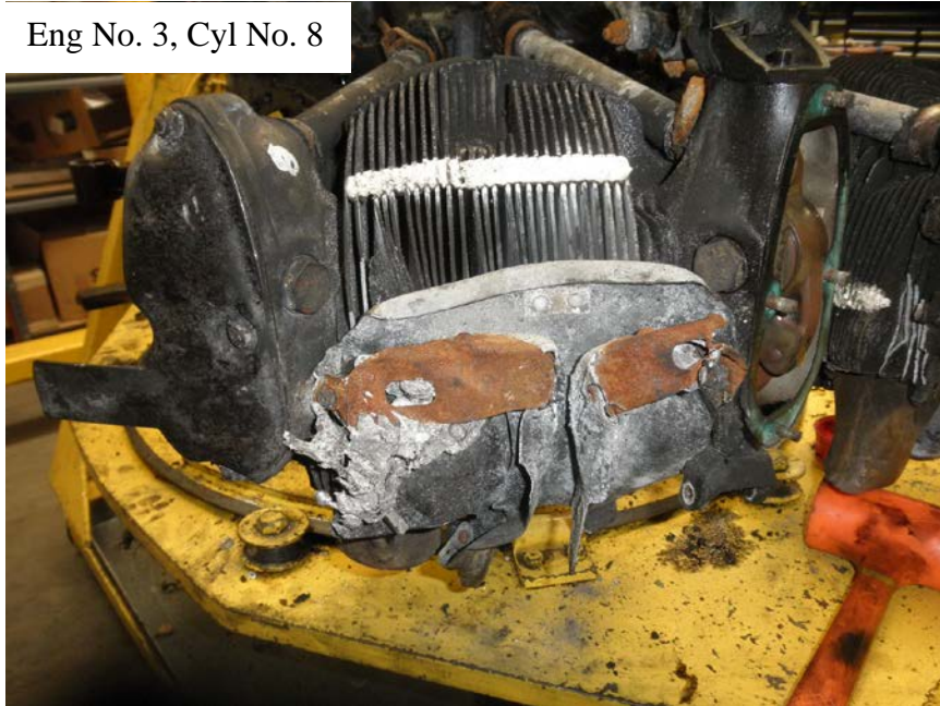
Photo No. 108: View of the No. 8 cylinder head showing the metal slag.
