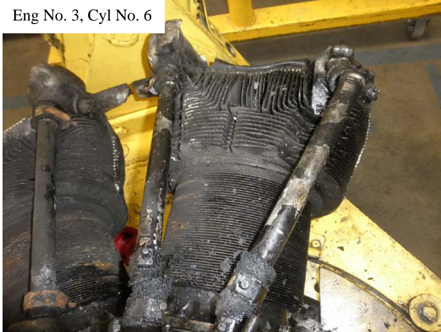
Photo No. 93: View of the front of No. 6 cylinder showing that it was in place on the crankcase and that it was intact with the head in place.
