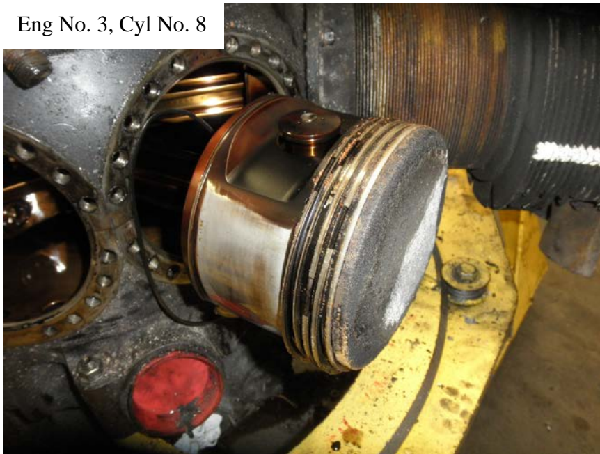
Photo No. 109: View of No. 8 cylinder's piston showing that it was intact.
