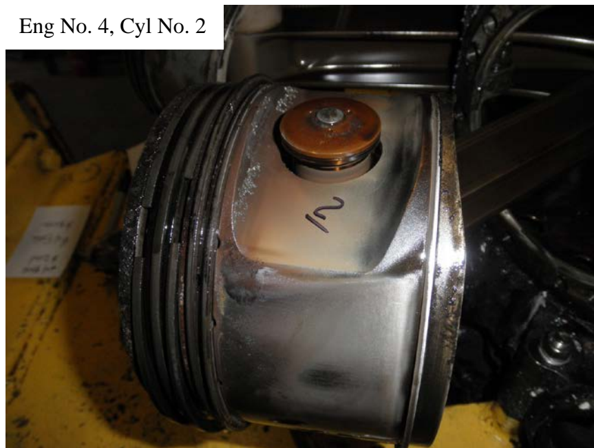
Photo No. 160: View of No. 2 cylinder's piston in place on the articulating rod showing that the piston was intact and that all of the piston rings were in place.
