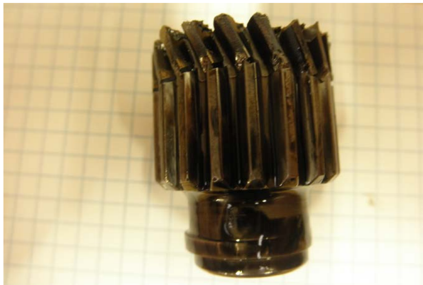
Photo No. 127: View of side of aft end of accessory drive gear shaft showing splines at fractured end twisted slightly.
