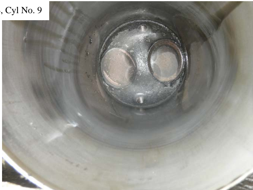
Photo No. 193: View of the inside of the No. 9 cylinder showing no damage to the barrel and the two valves centered in place in the closed position.
