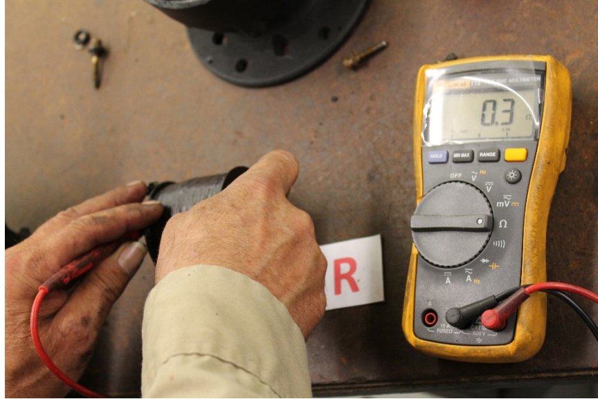
Photo No. 30: Right magneto coil assembly's primary coil resistance was 0.3 ohms. (S&T)
