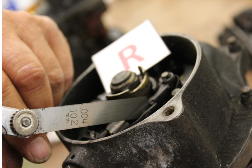
Photo No. 26: Close up view of right magneto's measured point gap of 0.004 inches. (S&T)
