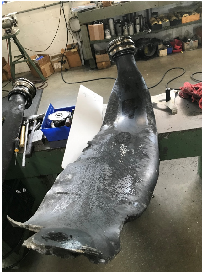
Photo No. 209: View of blade No. 3 showing the missing piece of the tip and the bend to the camber side as well as the thermal damage.
