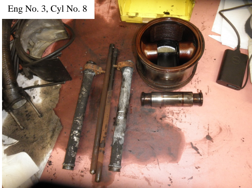
Photo No. 110: View of the underside of the No. 8 cylinder's piston, the piston pin, push rod shrouds, and the push rods.
