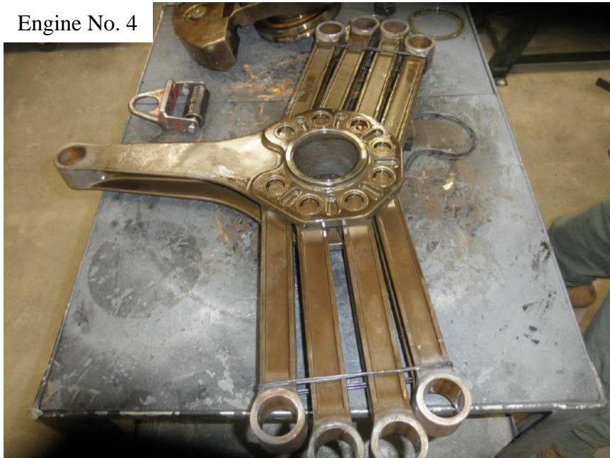
Photo No. 154: View of the master rod and all of the articulating rods showing all were intact and undamaged.
