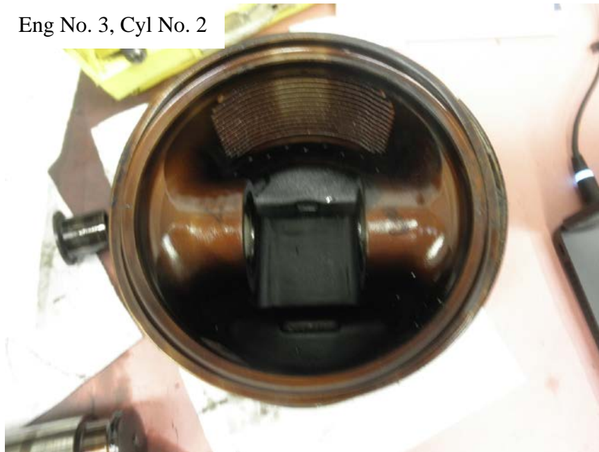
Photo No. 63: Close up of underside of No. 2 cylinder's piston showing no damage.
