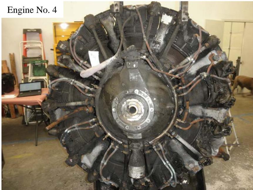
Photo No. 151: View of the front of the No. 4 engine showing all nine cylinders in place on the crank case.
