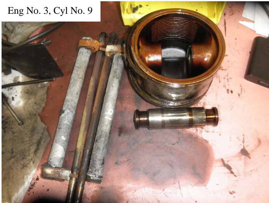
Photo No. 117: View of the underside of the No. 9 cylinder's piston, the piston pin, push rod shrouds, and the push rods.
