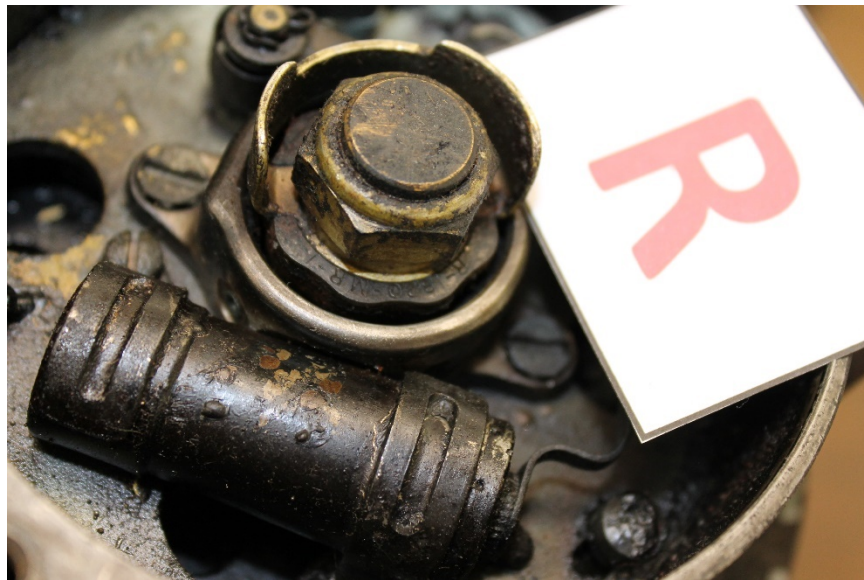
Photo No. 27: Close up view of right magneto's compensating cam showing it is marked R-1820 MR-1. (S&T)
