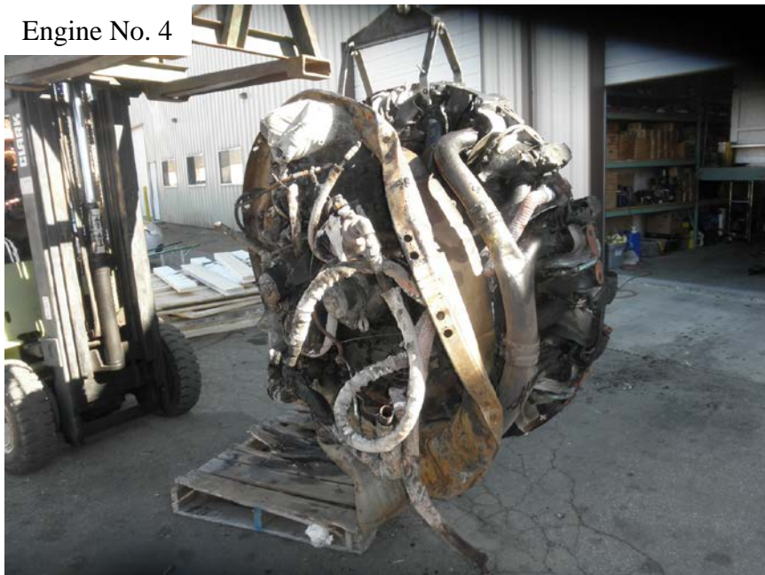
Photo No. 147: View of rear of No. 4 engine showing fire damage and some airframe structure still attached.
