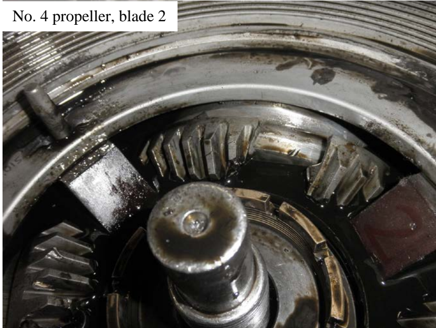
Photo No. 216: Close up view of No. 4 propeller, No. 2 blade's gear ring showing it was fractured.
