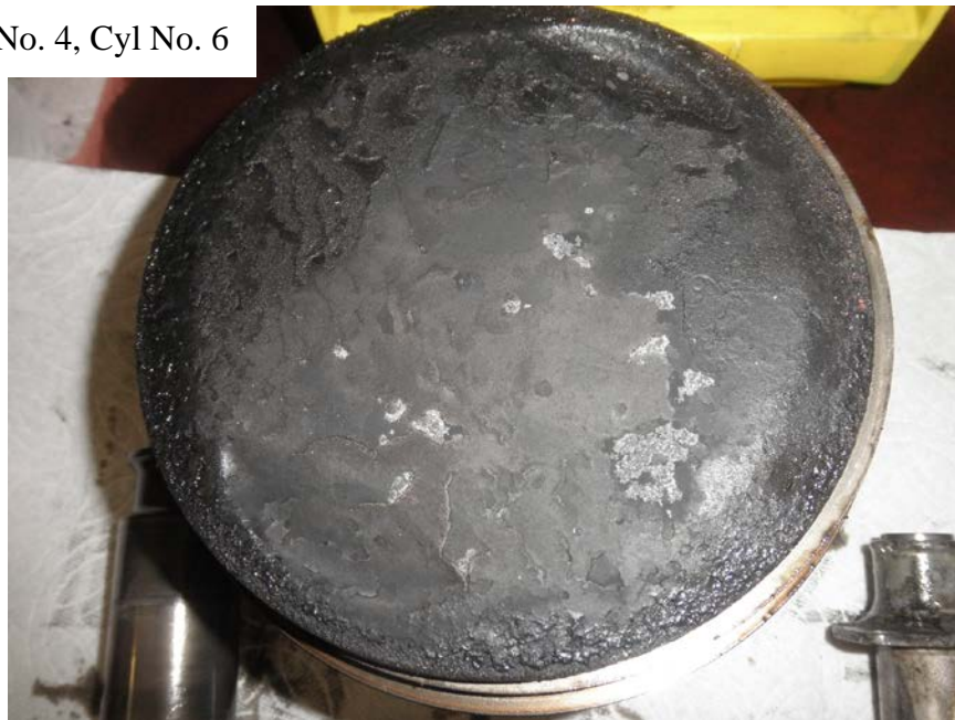
Photo No. 178: Close up view of the No. 6 piston's head showing the gray color.
