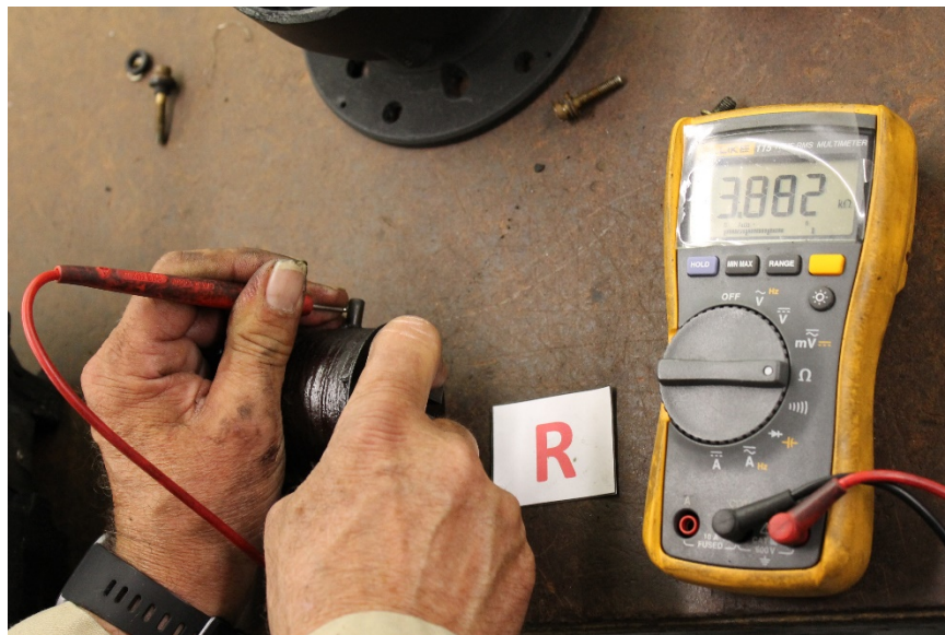
Photo No. 31: Right magneto coil assembly's secondary coil resistance was 3,882 ohms. (S&T)
