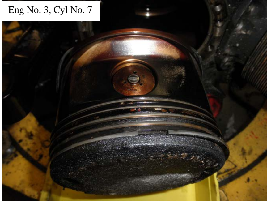
Photo No. 104: Close up view of side of No. 7 cylinder's piston showing all of the rings were in place.
