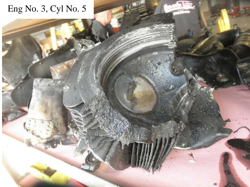
Photo No. 92: View of piece of No. 5 cylinder head with exhaust valve in place.
