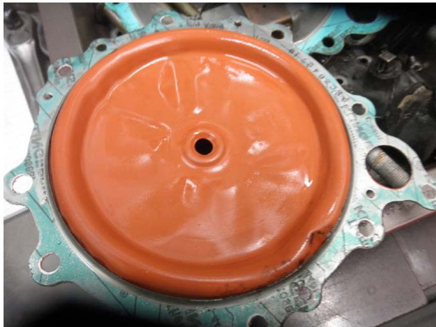
Photo No. 144: View of typical diaphragm showing it was intact.
