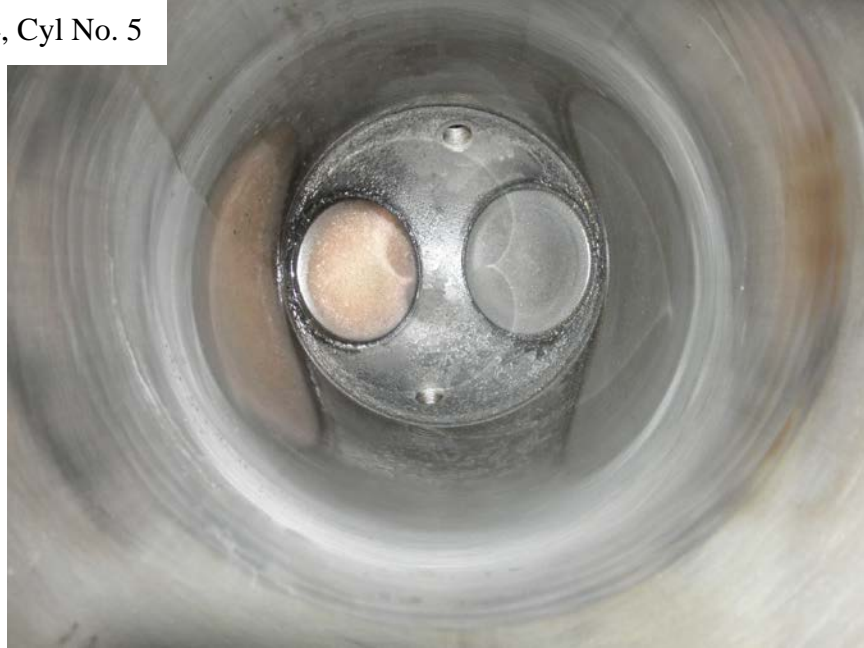
Photo No. 176: View of the inside of the No. 5 cylinder showing no damage to the barrel and the two valves were centered in place in the closed position.
