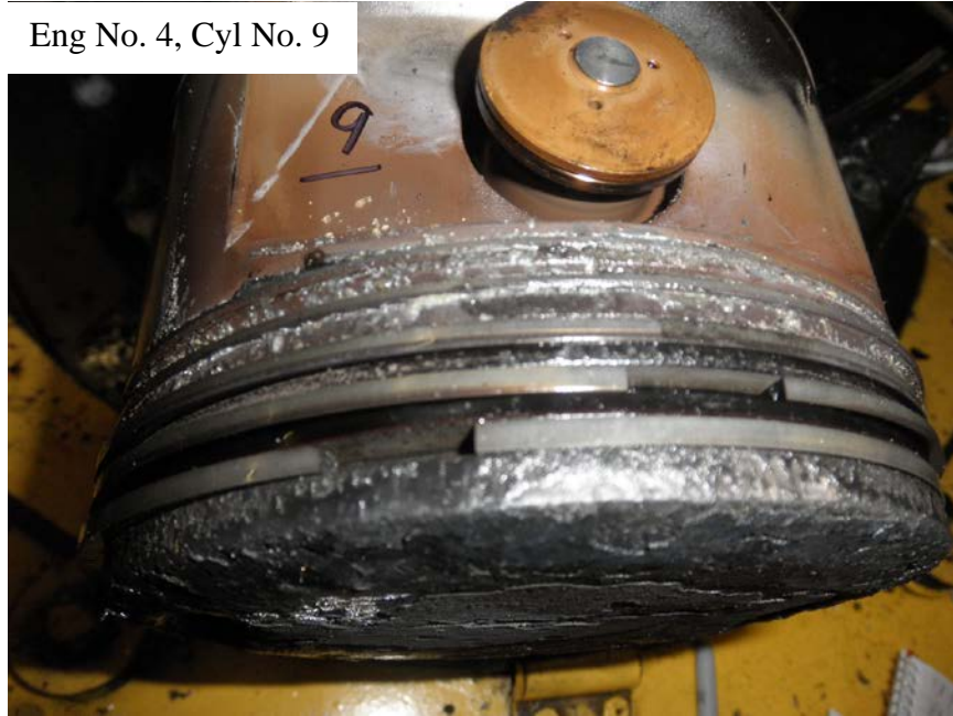
Photo No. 190: View of No. 9 cylinder's piston in place on the articulating rod showing that the piston was intact and that all of the piston rings were in place. Also shown are small metal particles in the piston rings.
