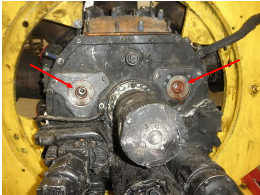
Photo No. 138: View of the left and right magneto drives showing a red material on the drives with more being on the right than on the left.
