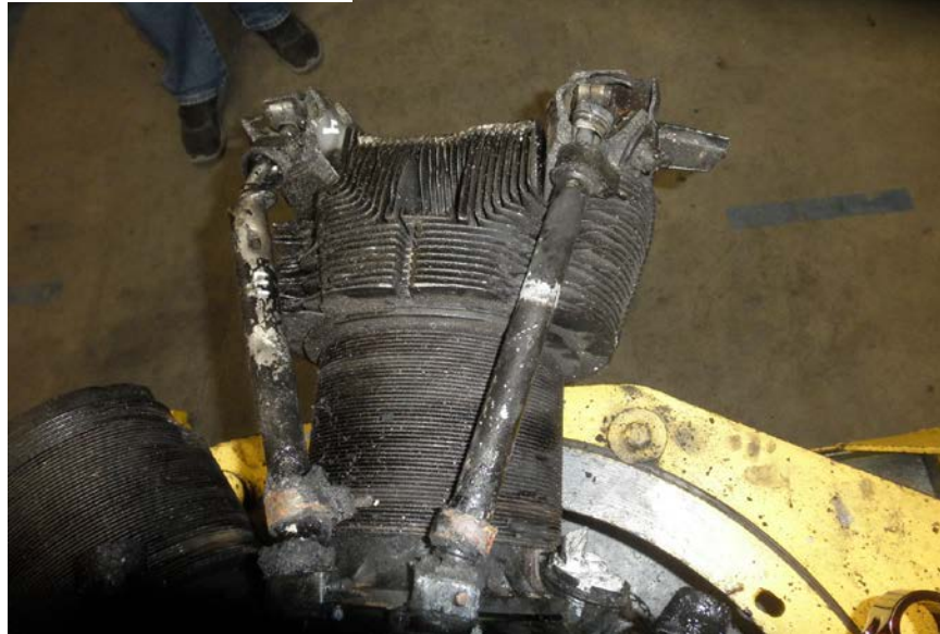
Photo No. 73: View of front of No. 4 cylinder showing it was intact with the head in place and intact except for the rocker arm assemblies and covers that were broken.
