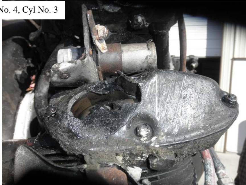
Photo No. 164: Close up view of the No. 3 cylinder's exhaust rocker arm cover showing the hole in the cover.
