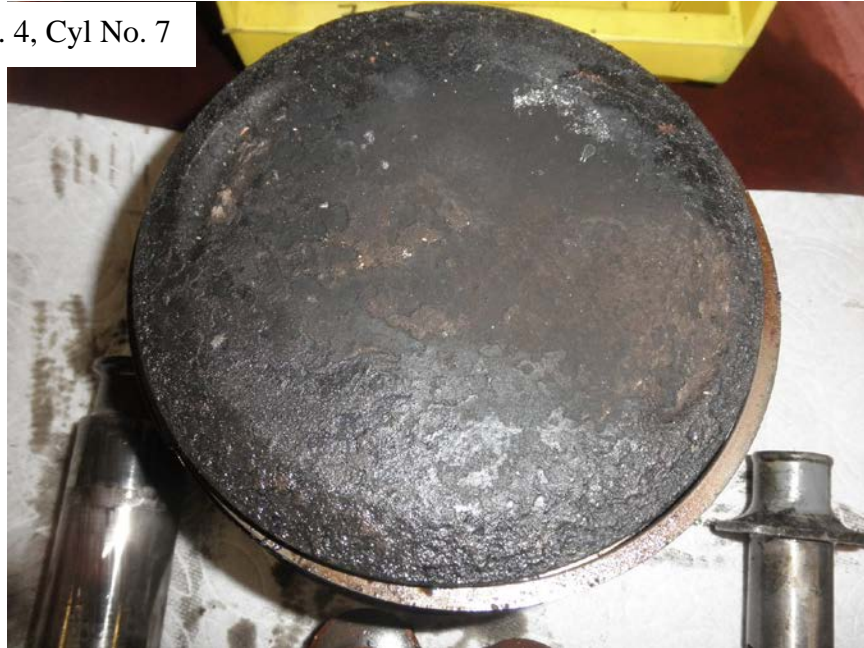
Photo No. 182: Close up view of the No. 7 piston's head showing the dark gray color.
