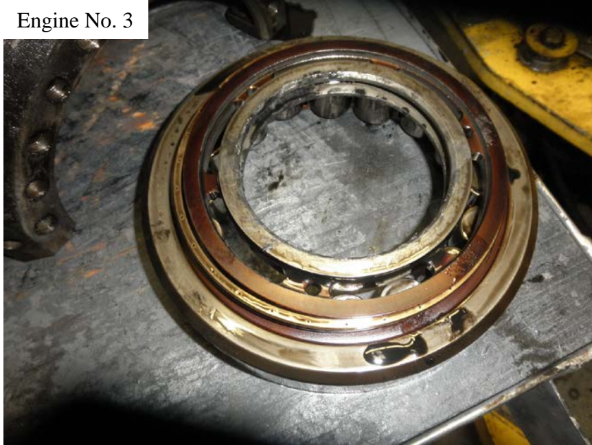
Photo No. 47: View of front crank shaft bearing showing that it was intact and the rollers were in place.
