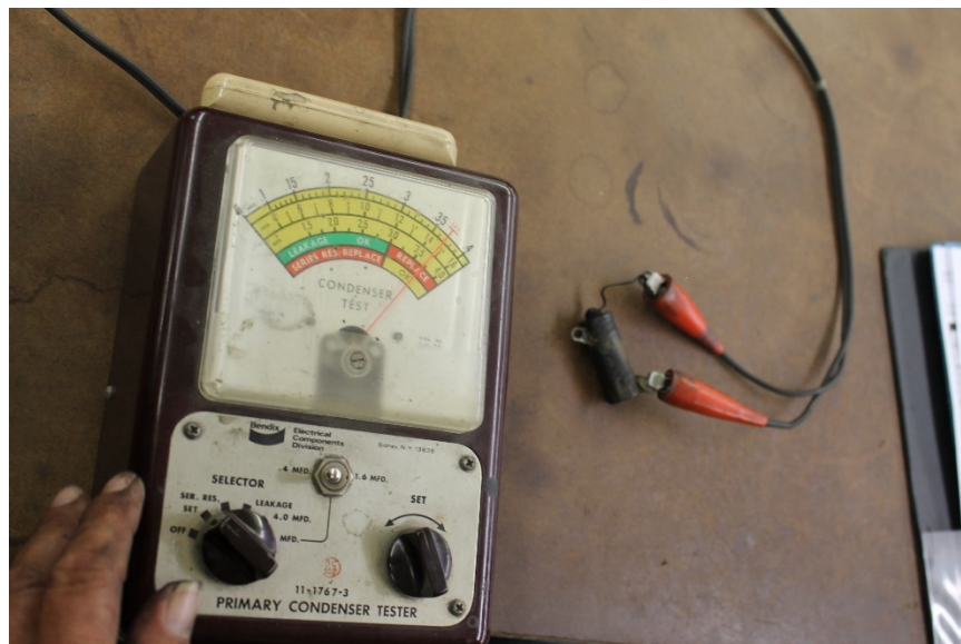
Photo No. 21: View of primary condenser tester. (S&T)
