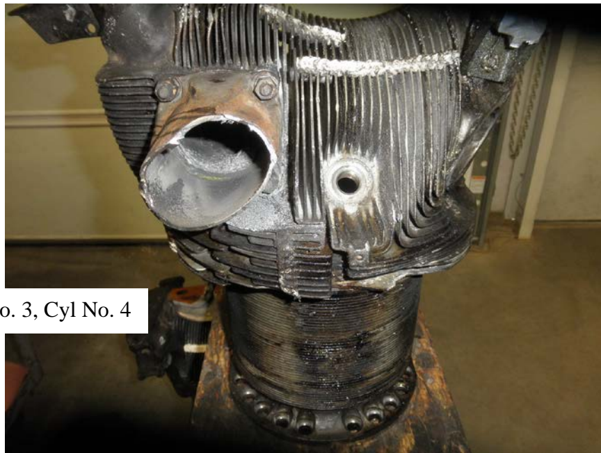
Photo No. 74: View of rear of No. 4 cylinder showing it was intact with the head in place and intact.
