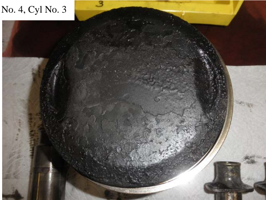
Photo No. 166: Close up view of the No. 3 piston's head showing the dark gray color.
