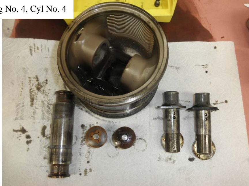
Photo No. 171: View of underside of No. 4 cylinder's piston along with the piston pin, piston pin buttons, and the cam followers showing all were intact and undamaged.
