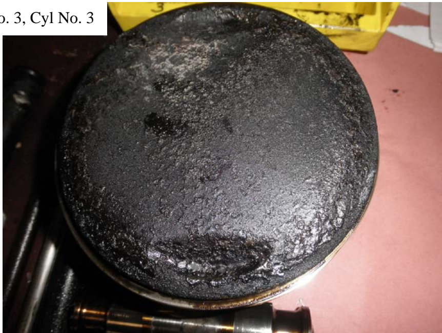
Photo No. 69: Close up view of No. 3 cylinder's piston head showing that it was intact and had a dark color.
