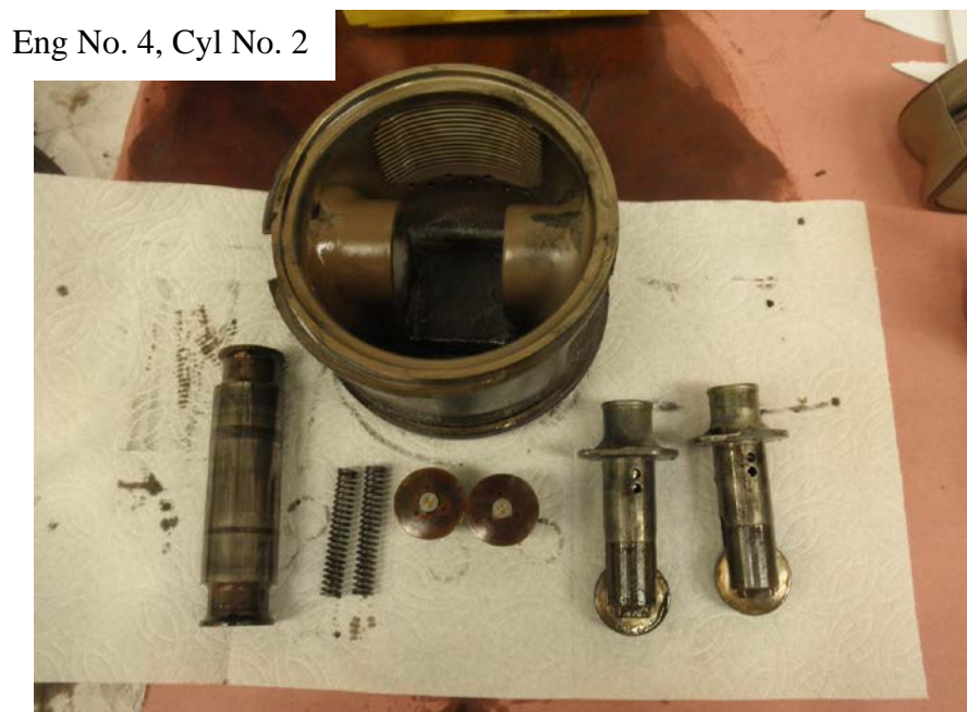
Photo No. 162: View of underside of No. 2 cylinder's piston along with the piston pin, piston pin buttons, and the cam followers showing all were intact and undamaged.
