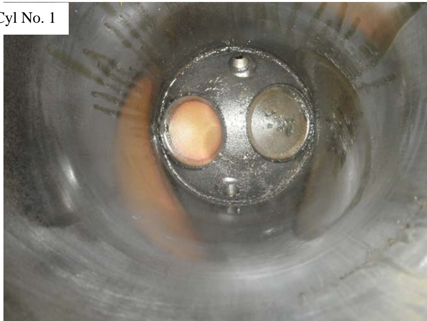
Photo No. 159: View of the inside of the No. 1 cylinder showing no damage to the barrel and the two valves were centered in place in the closed position.
