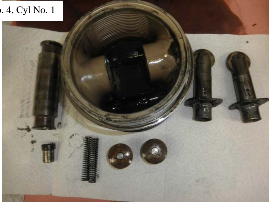
Photo No. 158: View of underside of No. 1 cylinder's piston along with the piston pin, piston pin buttons, and the cam followers showing all were intact and undamaged.
