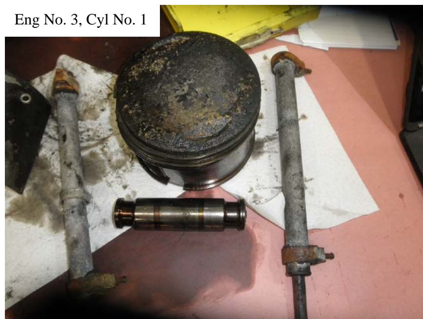
Photo No. 53: View of No. 1 cylinder's piston, piston pin, and push rod shrouds.
