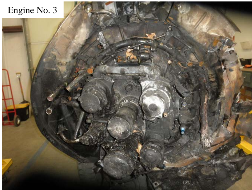
Photo No. 39: View of rear of No. 3 engine showing sooting, hose with charred and burned heat resistant covering, and accessories bent to the left.
