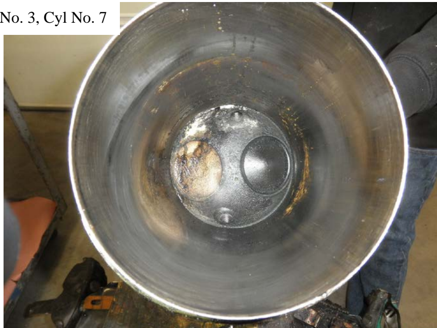
Photo No. 105: View inside of the No. 7 cylinder's barrel showing the dark color of the barrel and head and that the two valves were in place in the closed position.
