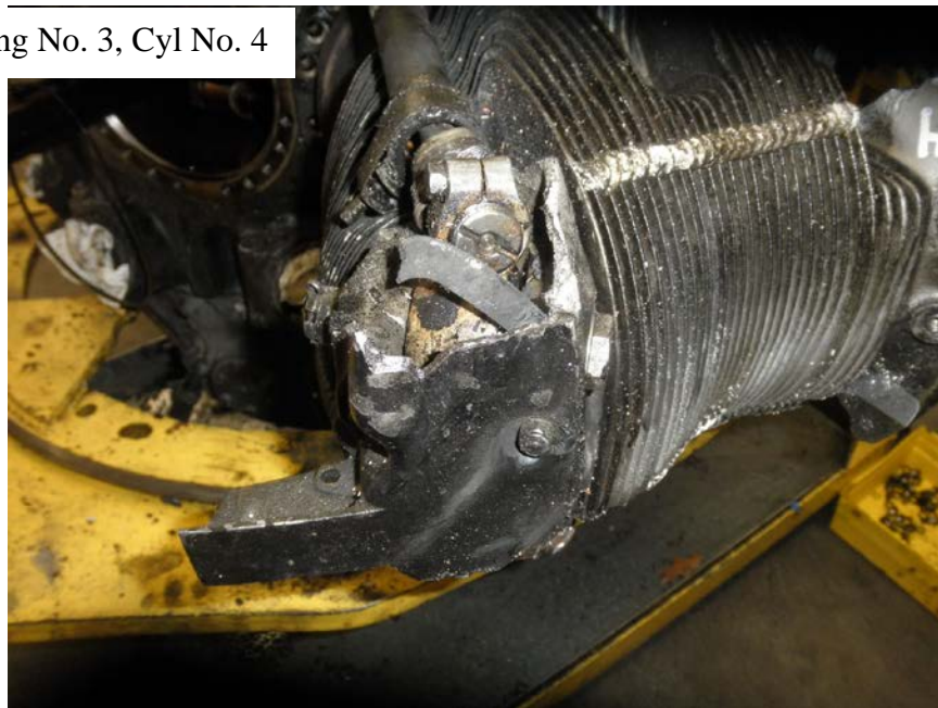
Photo No. 76: Close up view of broken exhaust rocker arm assembly and cover showing rocker arm intact.
