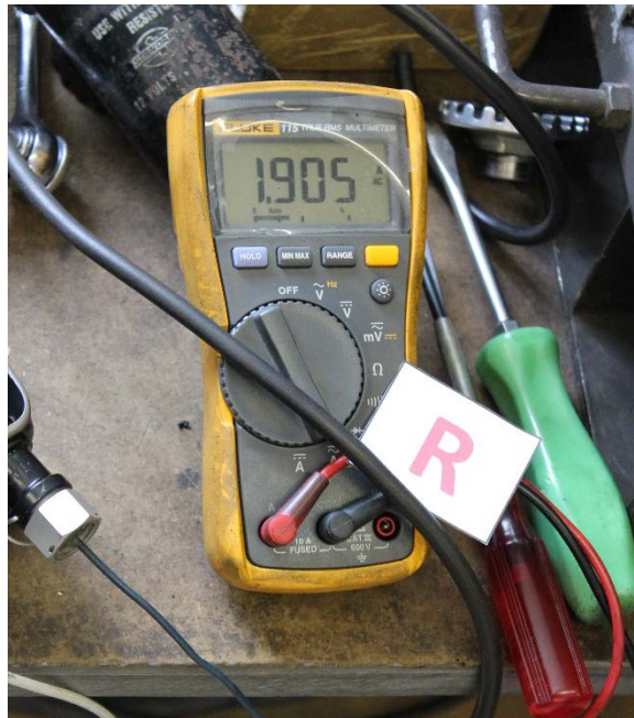
Photo No. 29: View of right magneto's multimeter reading of magnet's primary output of 1.905 amperes. (S&T)
