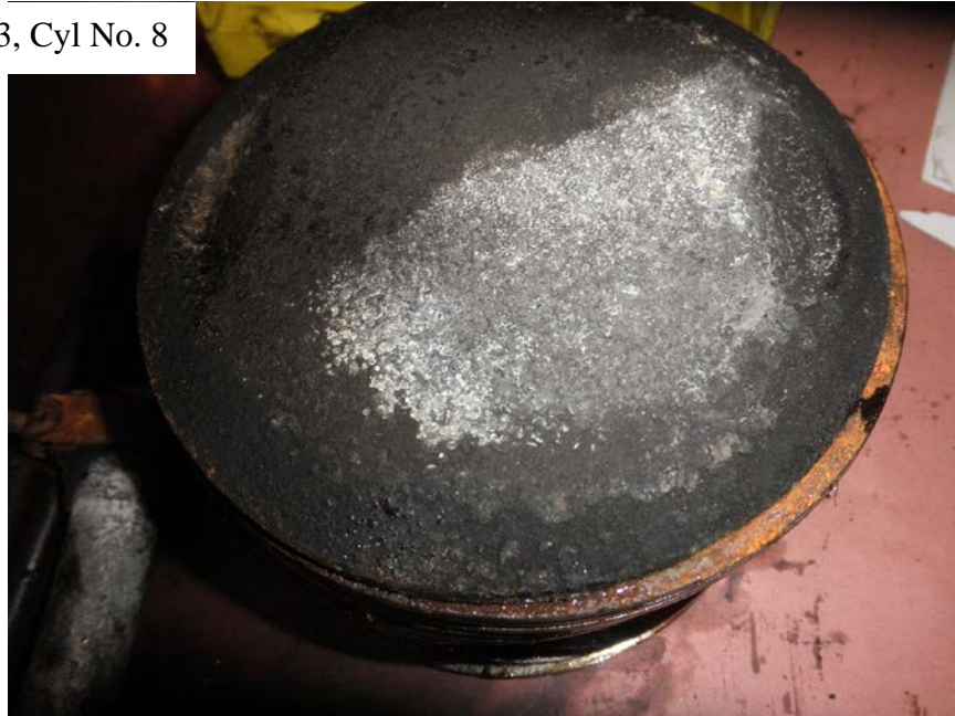
Photo No. 112: Close up view of the head of the No. 8 cylinder's piston showing it to be mostly a dark color with a light colored area.
