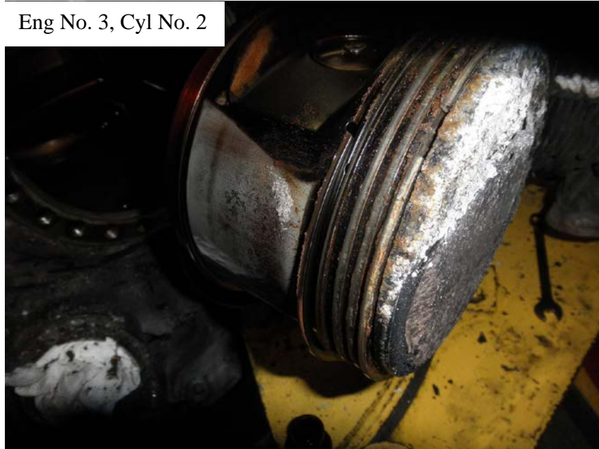
Photo No. 64: Close up view of side of No. 2 cylinder's piston showing the rings were in place.
