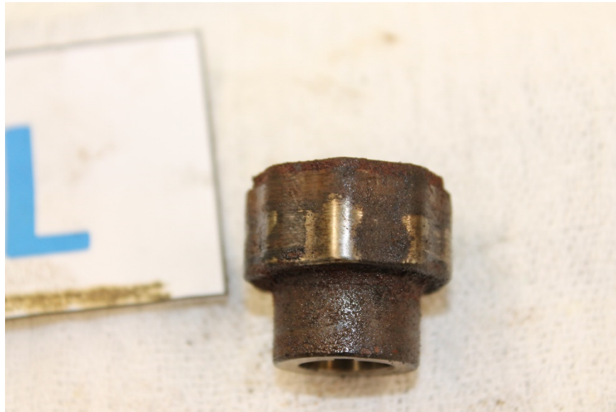
Photo No. 25: Close-up view of left magneto's cam compensator showing smooth wear surface. (S&T)
