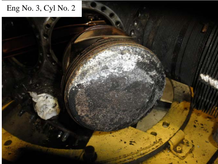
Photo No. 62: Close up of No. 2 cylinder's piston head showing that it was intact and had a dark color with small gray- and white-colored areas.
