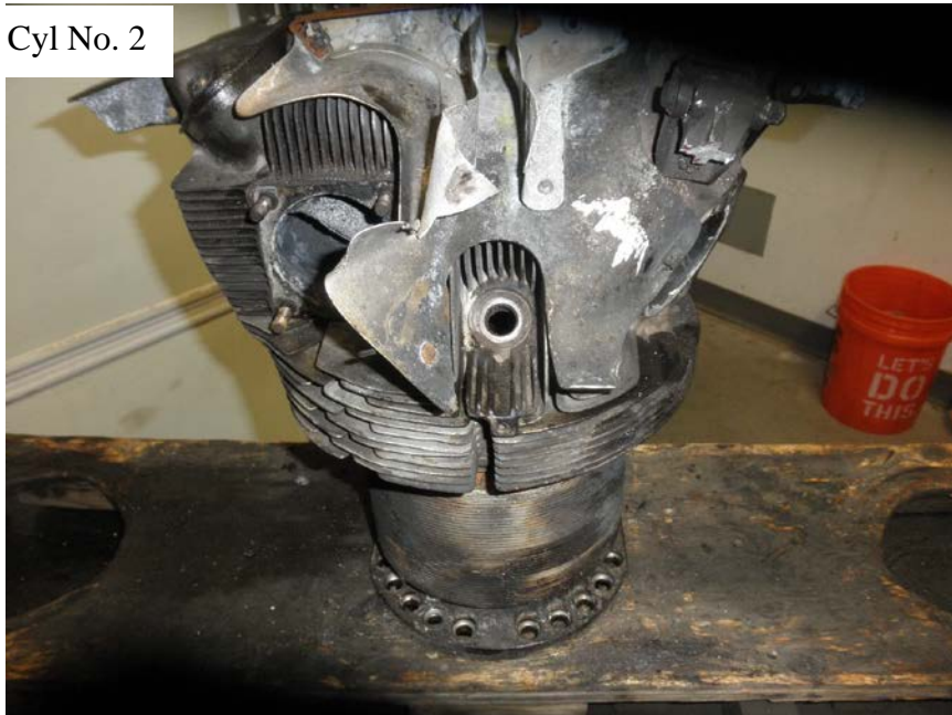
Photo No. 59: View of rear of No. 2 cylinder showing it was intact with the head in place and intact, and the intake and exhaust rocker arm covers were in place.
