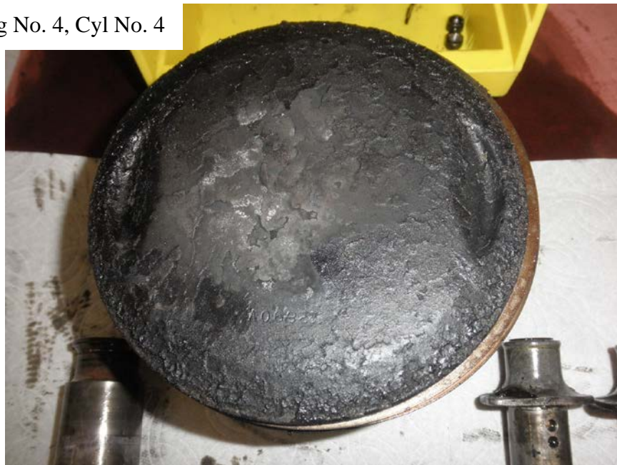
Photo No. 170: Close up view of the No. 4 piston's head showing the dark gray color.
