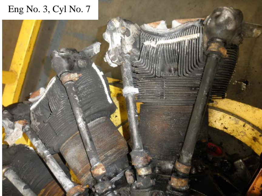
Photo No. 100: View of the front of No. 7 cylinder showing that it was in place on the crankcase and that it was intact with the head in place.
