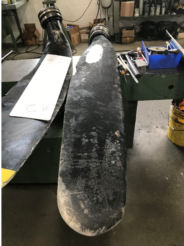
Photo No. 204: View of blade No. 1 showing it was full length and essentially straight with the thermal damage along the camber side.
