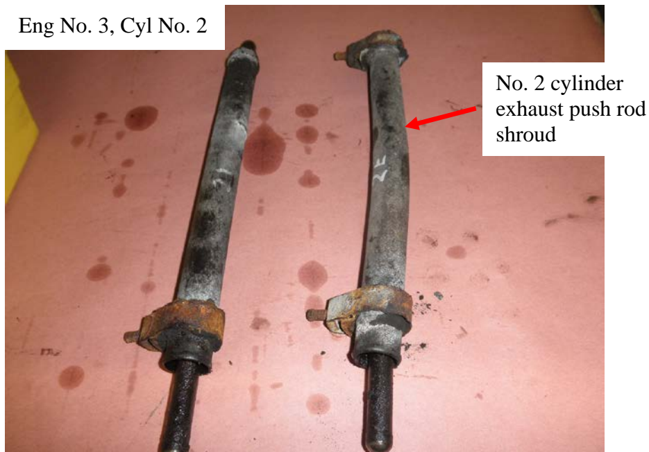
Photo No. 61: View of the two push rod shrouds and push rods showing the exhaust push rod shroud was bent slightly.
