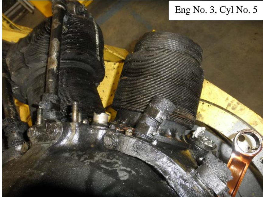
Photo No. 82: View of No.5 cylinder barrel in place on the crankcase.
