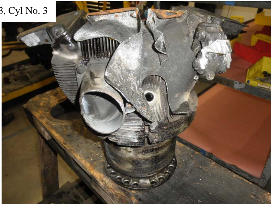
Photo No. 67: View of rear of No. 3 cylinder showing it was intact with the head in place and intact, and the intake and exhaust rocker arm covers were in place.
