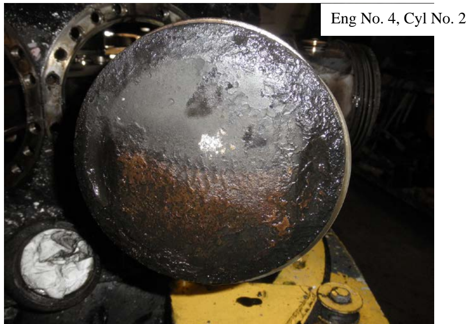
Photo No. 161: Close up view of the No. 2 piston's head showing the dark- and bronze-colored areas.
