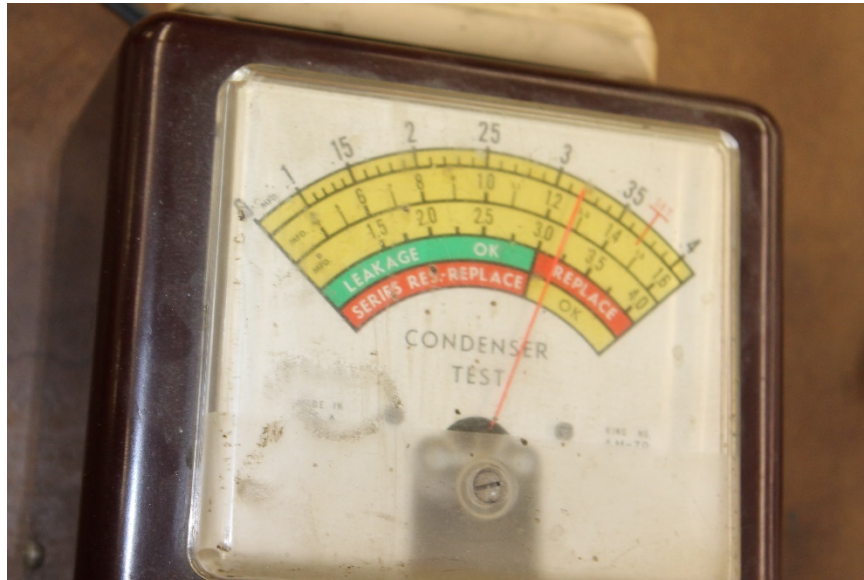
Photo No. 22: View of left magneto's condenser test showing the resistance was good. (S&T)
