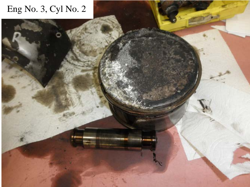
Photo No. 60: View of the No. 2 cylinder's piston and wrist pin showing that they were undamaged.
