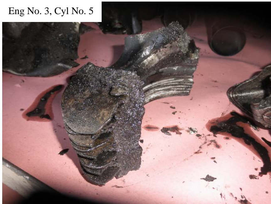
Photo No. 85: Broken piece of No. 5 cylinder head.
