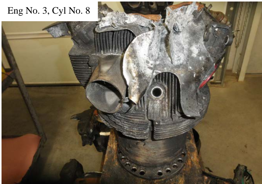
Photo No. 107: View of the rear of No. 8 cylinder showing that it was intact with the head in place.
