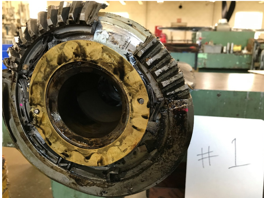
Photo No. 205: Close up view of blade No. 1's gear segment broken at the low pitch position.
