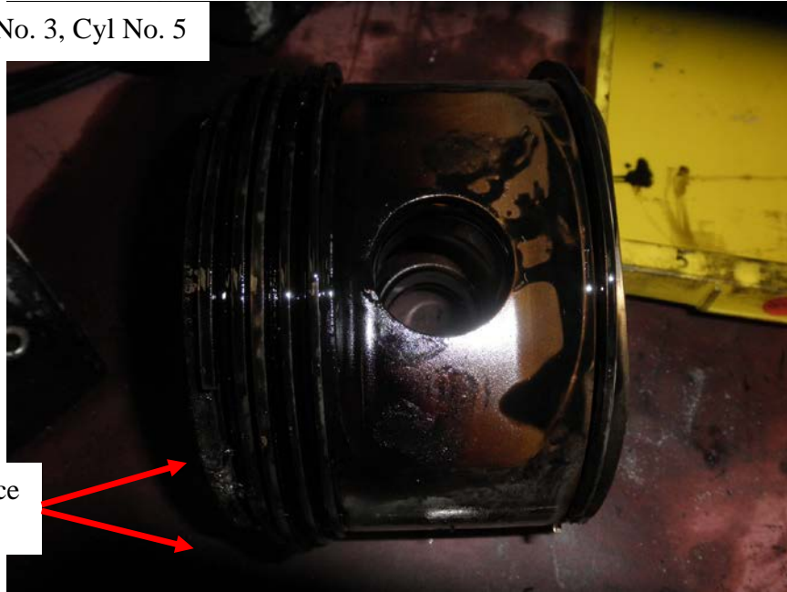
Photo No. 88: Close up of No. 5 cylinder's piston rings showing all were in place.
