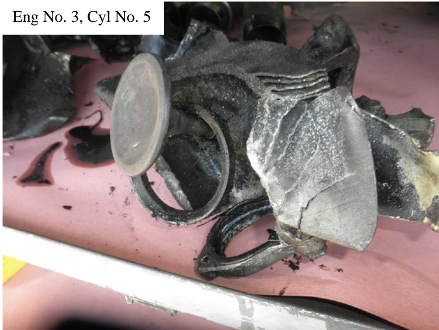
Photo No. 91: View of piece of No. 5 cylinder head with bent intake valve.
