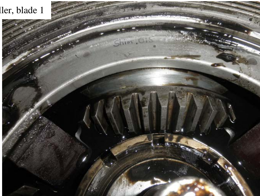
Photo No. 215: Close up view of No. 4 propeller, No. 1 blade's gear ring showing it was intact.
