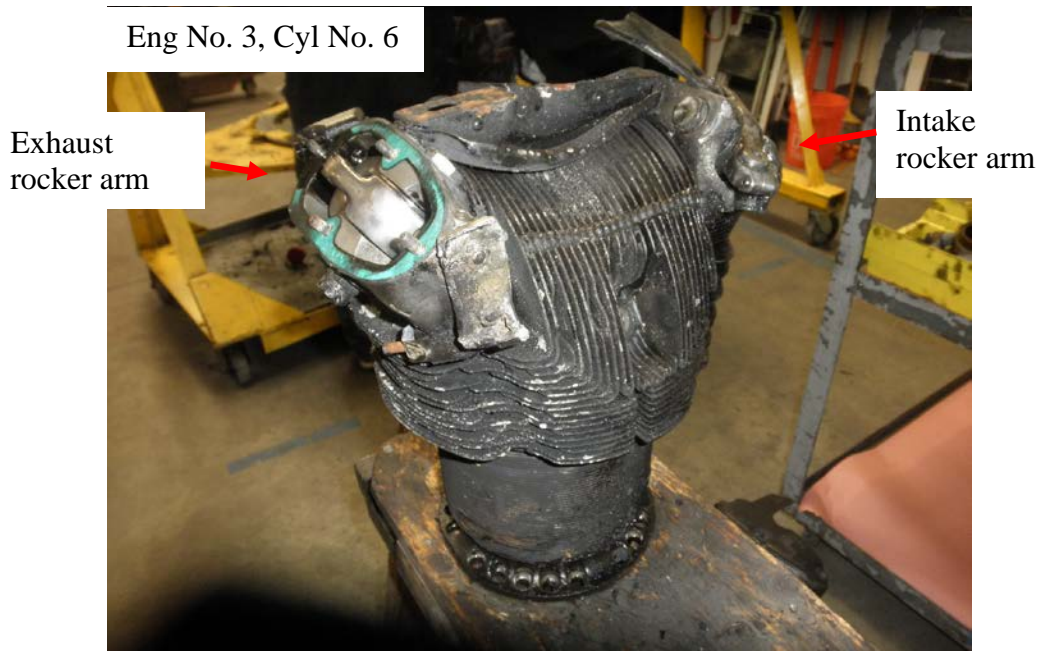
Photo No. 95: View of head of the No. 6 cylinder showing the intake and exhaust rocker arm assemblies were broken open exposing the rocker arms.
