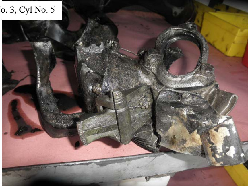
Photo No. 84: Broken piece of No. 5 cylinder head.
