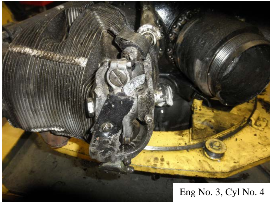
Photo No. 75: Close up view of broken intake rocker arm assembly and cover showing rocker arm intact.
