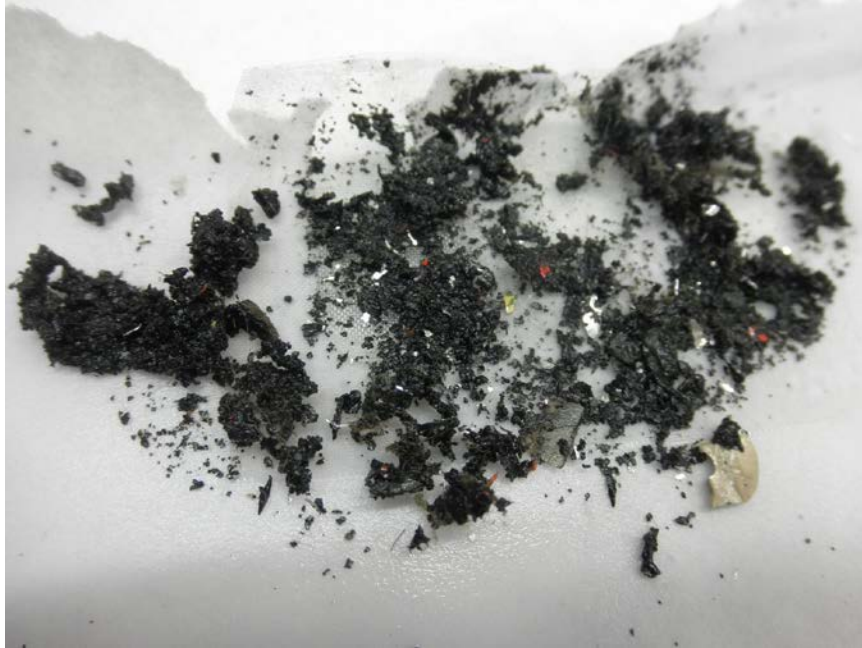
Photo No. 132: Debris that was flushed from the No. 3 engine's Cuno oil filter.
