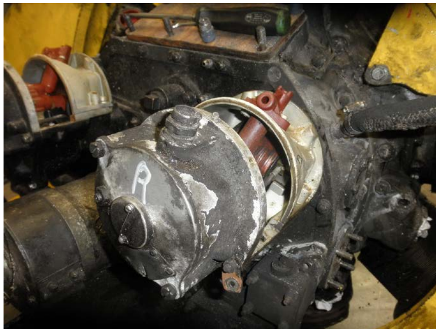
Photo No. 135: Close up view of right magneto housing showing it was intact, but the paint was blistered and partially burned away.
