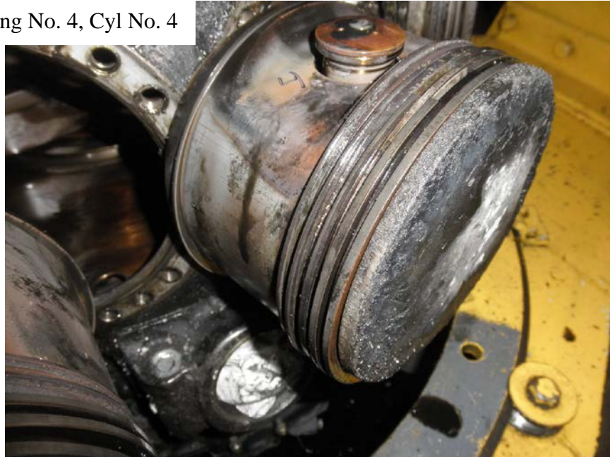
Photo No. 169: View of No. 4 cylinder's piston in place on the articulating rod showing that the piston was intact and that all of the piston rings were in place.
