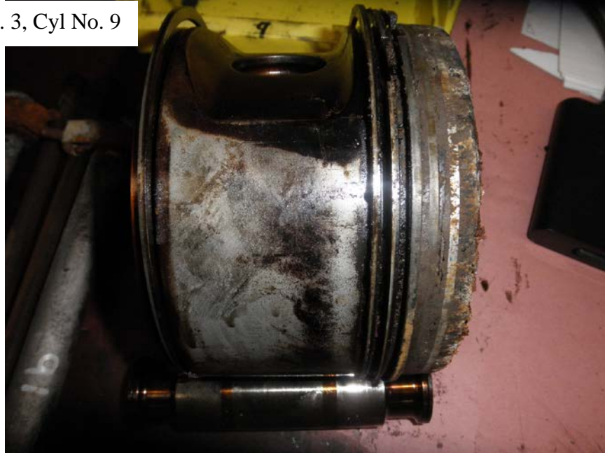
Photo No. 118: Close up view of the side of the No. 9 cylinder's piston showing the rings were in place.
