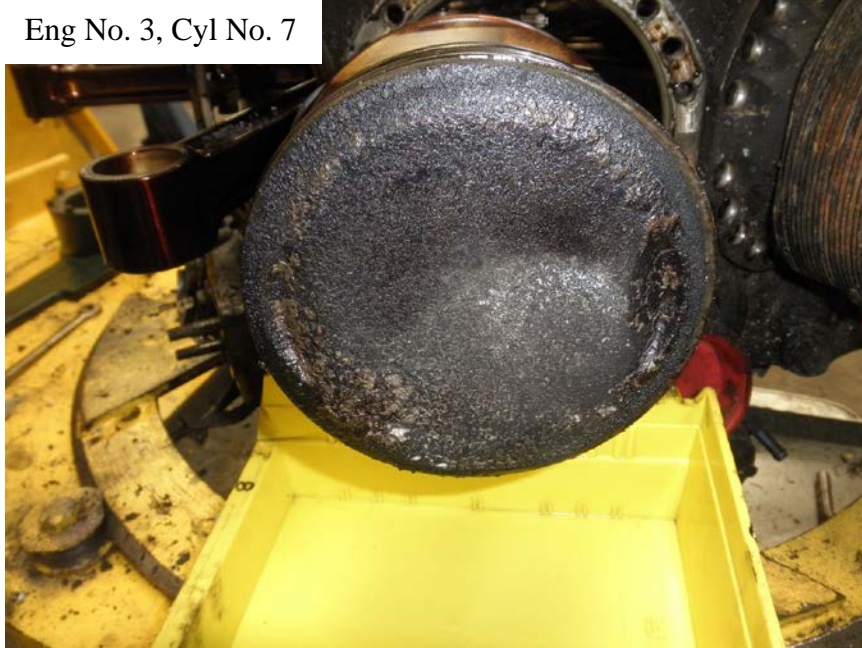
Photo No. 102: View of the head of the No. 7 cylinder's piston showing that it was intact.
