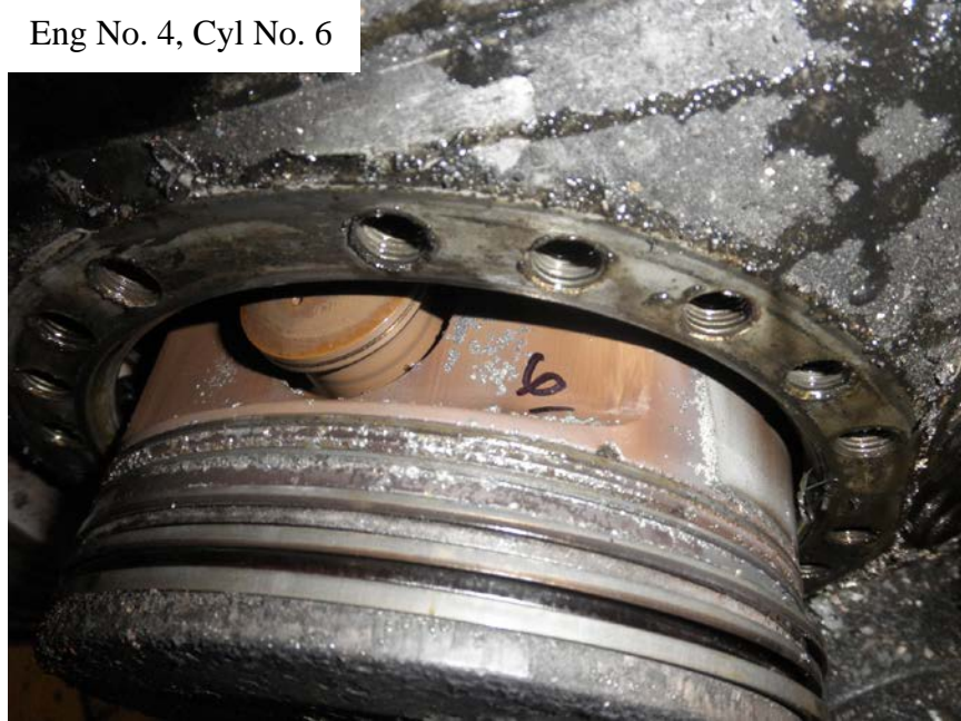
Photo No. 177 View of No. 6 cylinder's piston in place on the articulating rod showing that the piston was intact and that all of the piston rings were in place.
