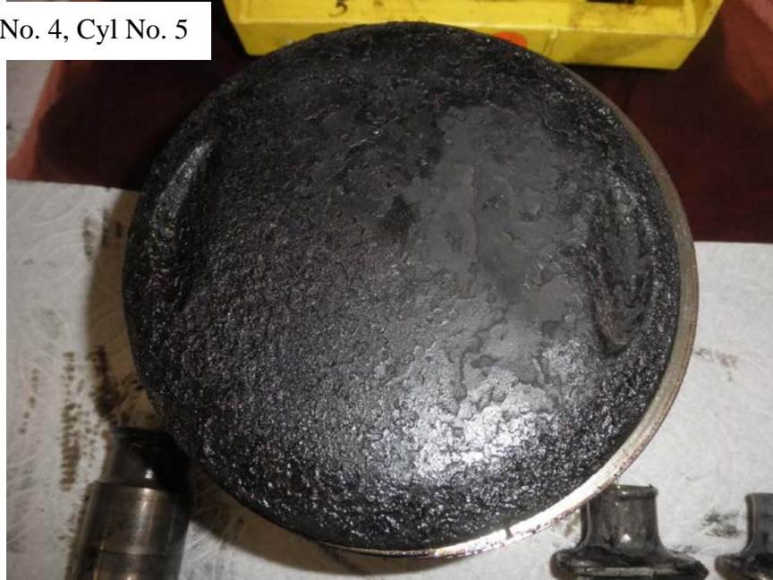
Photo No.174: Close up view of the No. 5 piston's head showing the dark gray color.
