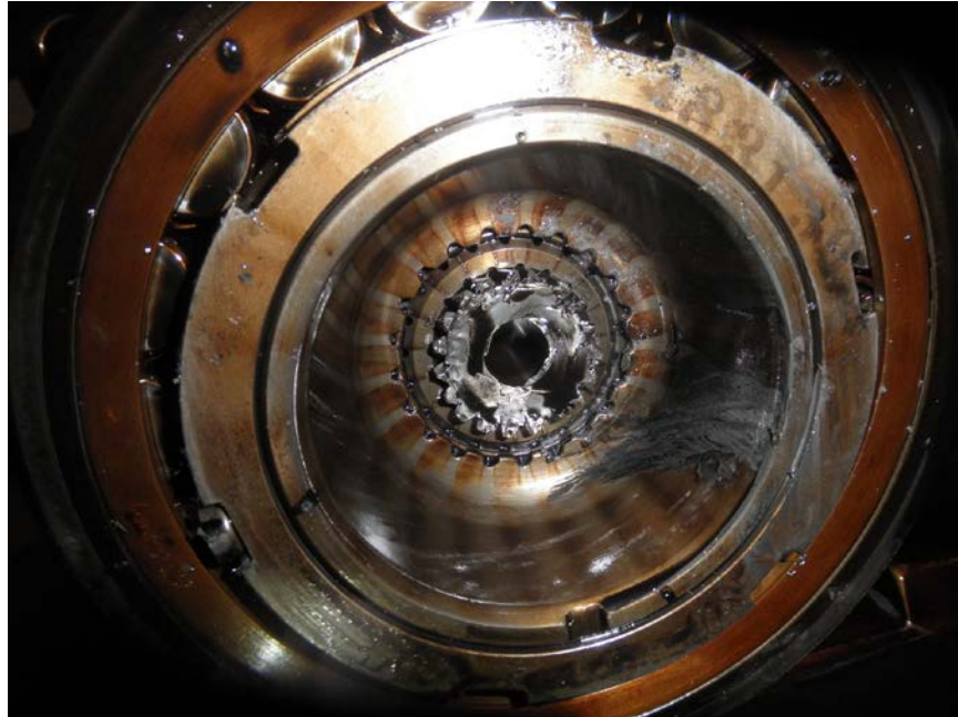
Photo No. 126: View of fractured forward end of accessory drive gear shaft in end of crankshaft.
