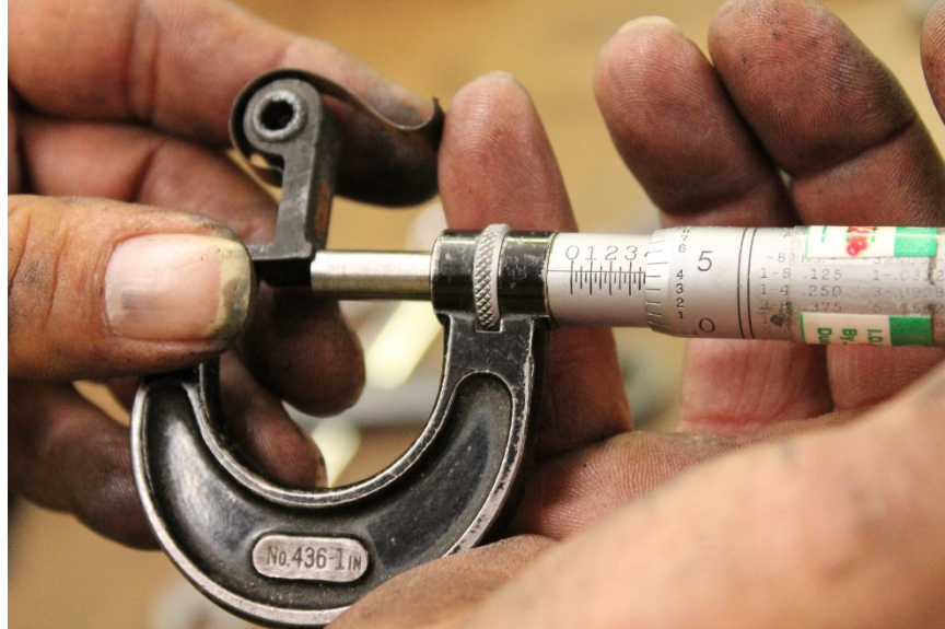
Photo No. 24: View showing the measurement of the left magneto's cam follower at 0.379 inches. (S&T)
