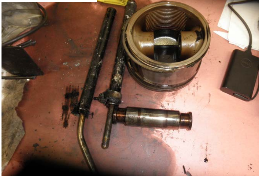
Photo No. 97: View of the underside of the No. 6 cylinder piston and the piston pin.
