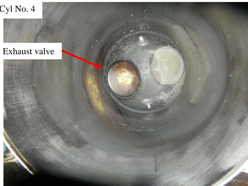
Photo No. 172: View of the inside of the No. 4 cylinder showing no damage to the barrel and the two valves were centered in place in the closed position. Also shown is what appeared to be yellow paint on the exhaust valve.
