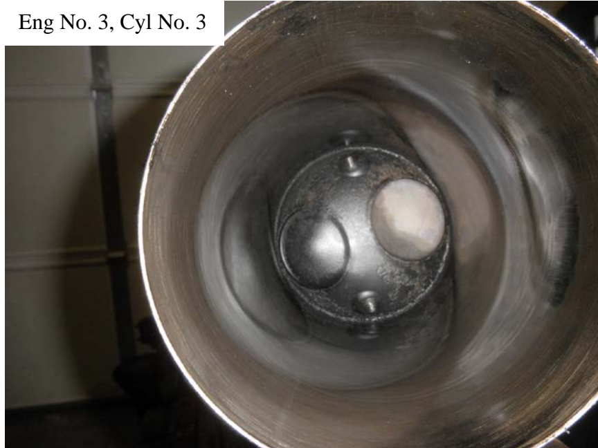
Photo No. 72: View of the inside of the No. 3 cylinder showing no damage to the barrel and the valves centered in the closed position.
