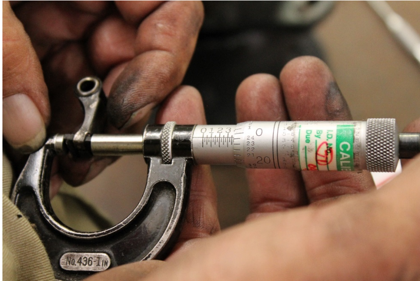
Photo No. 34: View showing the measurement of the left magneto's cam follower at 0.374 inches. (S&T)
