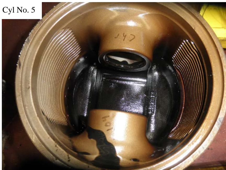
Photo No. 87: View of underside of No. 5 cylinder's piston.
