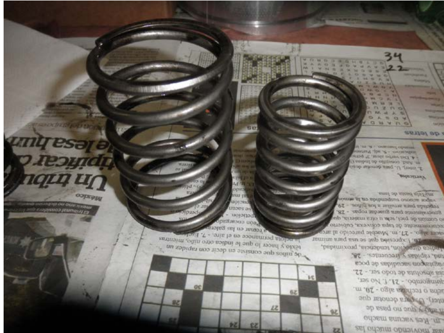
Photo No. 124: View of two valve springs that were found in the No. 3 engine's cylinders.
