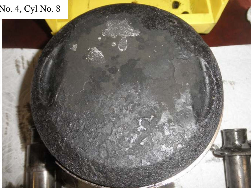
Photo No. 187: Close up view of the No. 8 piston's head showing the dark gray color with the white-colored patches.
