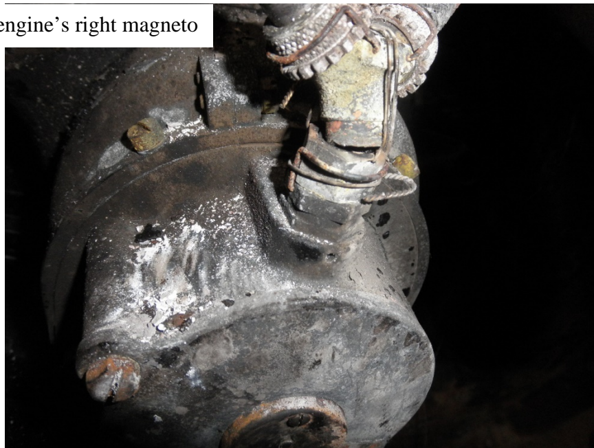
Photo No. 3: Close up of No. 4 engine's right magneto showing P-lead partially pulled out of the fitting and the single strand of safety wire wrapped around the lead.
