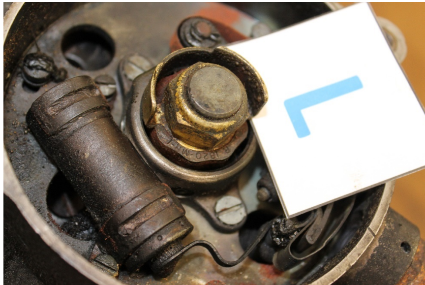
Photo No. 16: Close up view of left magneto's compensating cam showing it is marked R-1820 MR-1. (S&T)
