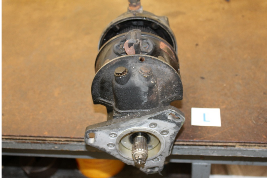
Photo No. 11: Left magneto as removed from the box. (S&T)
