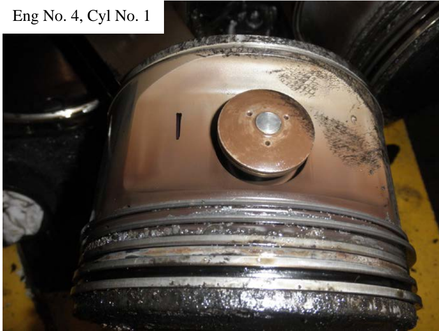
Photo No. 156: View of No. 1 cylinder's piston in place on the master rod showing that the piston was intact and that all of the piston rings were in place.
