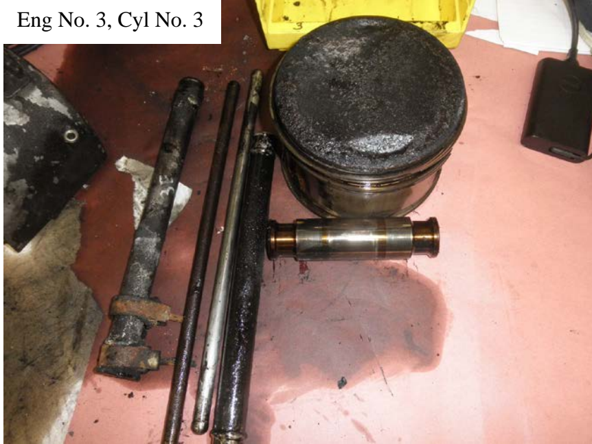
Photo No. 68: View of No. 3 cylinder's piston, wrist pin, push rods, and push rod shrouds.
