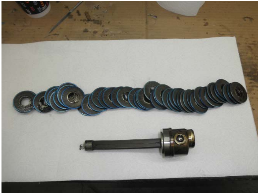
Photo No. 131: The No. 3 engine's Cuno oil filter elements after they were unstacked.
