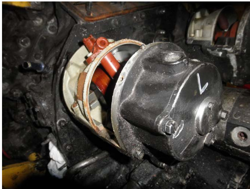
Photo No. 134: Close up view of left magneto housing showing it was intact.
