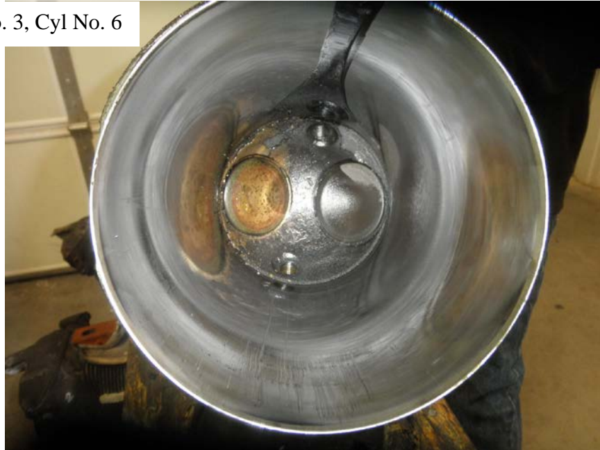
Photo No. 99: View of the inside of the No. 6 cylinder showing no damage to the barrel and the two valves centered in place in the closed position.
