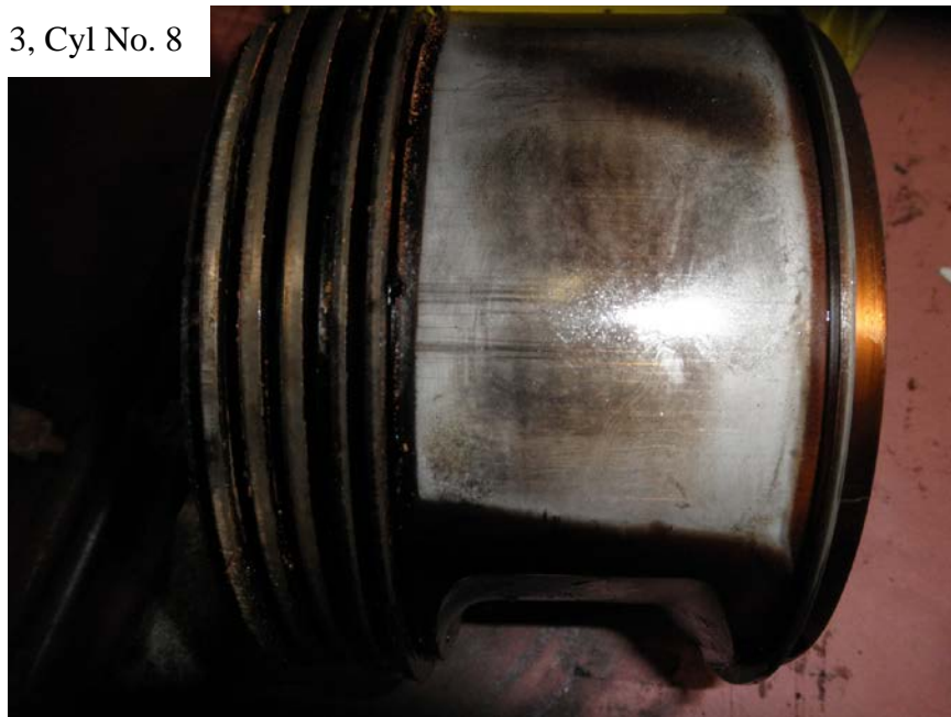
Photo No. 111: Close up view of the side of the No. 8 cylinder's piston showing the rings were in place.
