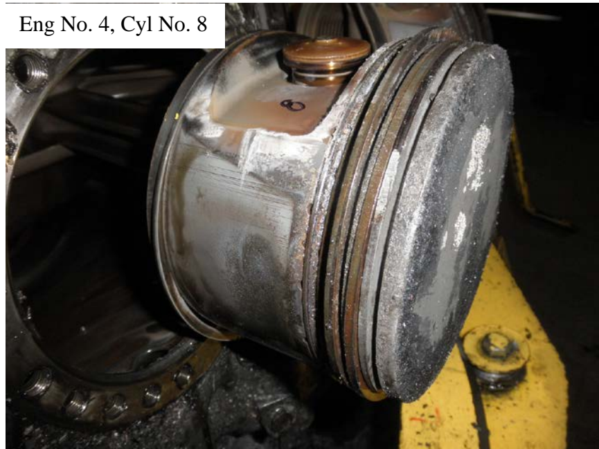
Photo No. 185: View of No. 8 cylinder's piston in place on the articulating rod showing that the piston was intact and that all of the piston rings were in place. Also shown are small metal particles in the piston rings.
