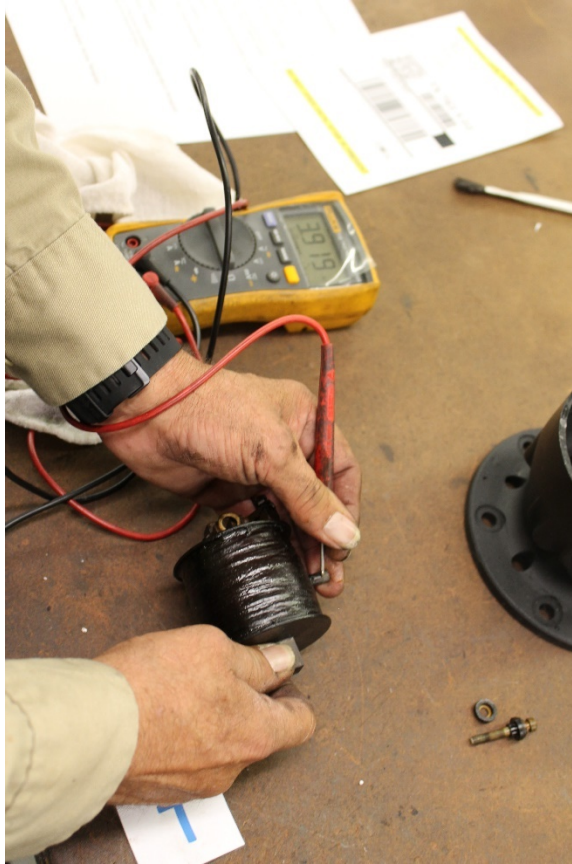
Photo No. 20: Left magneto coil assembly's secondary coil resistance was 3,919 ohms. (S&T)
