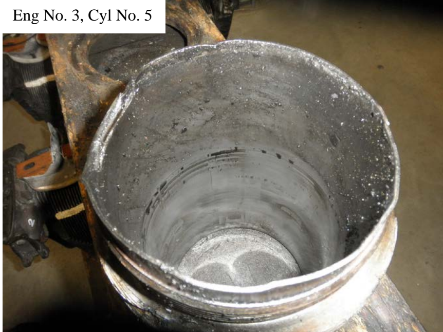
Photo No. 90: View of top of No. 5 cylinder barrel showing metal fragments.
