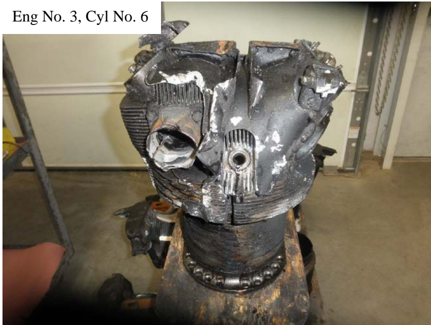
Photo No. 94: View of the rear of No. 6 cylinder showing that it was intact with the head in place.
