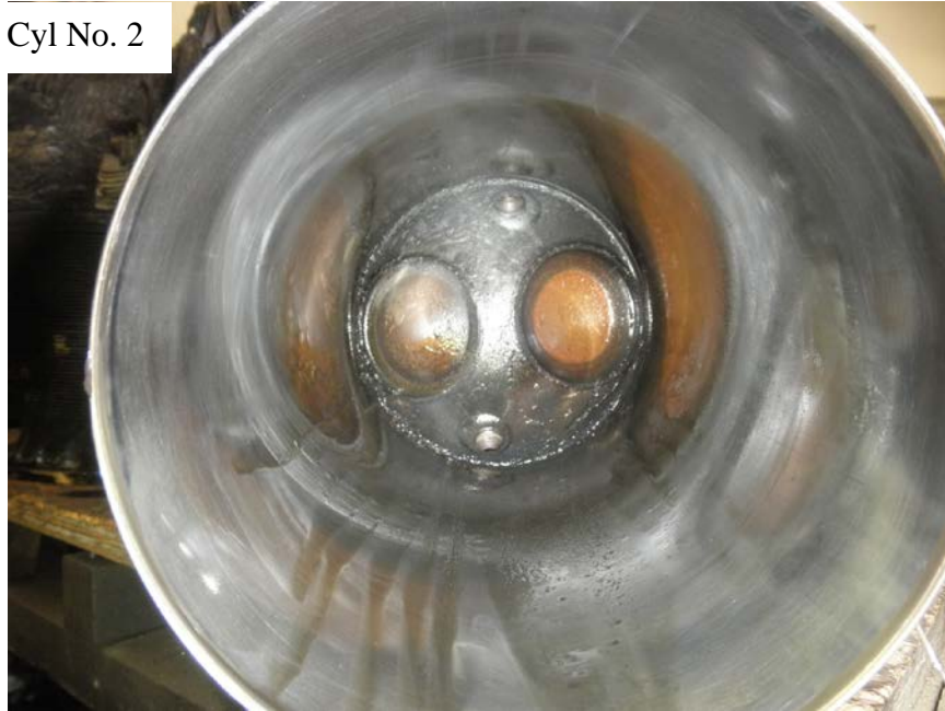
Photo No. 163: View of the inside of the No. 2 cylinder showing no damage to the barrel and the two valves were centered in place in the closed position.
