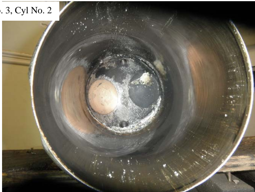
Photo No. 65: View of the inside of the No. 2 cylinder showing no damage to the barrel and the two valves centered in place in the closed position.
