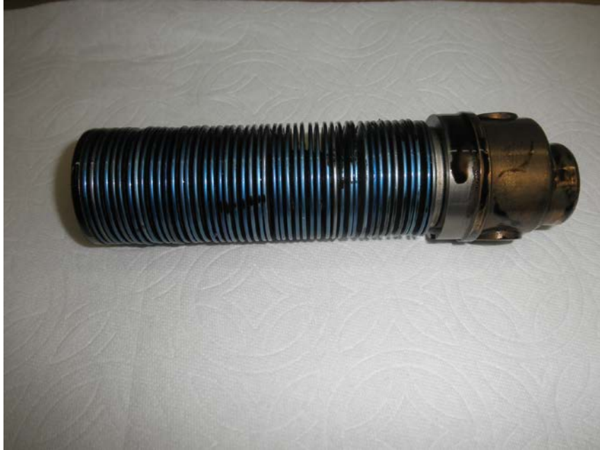
Photo No. 130: The No. 3 engine's Cuno oil filter after the filter housing was removed.
