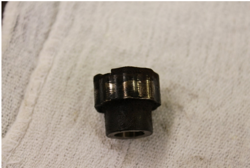
Photo No. 35: Close up of right magneto's compensator cam showing wear and scoring on the cam lobes. (S&T)
