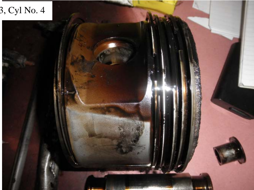
Photo No. 79: Close up view of the side of No. 4 cylinder's piston showing all of the rings were in place and intact.
