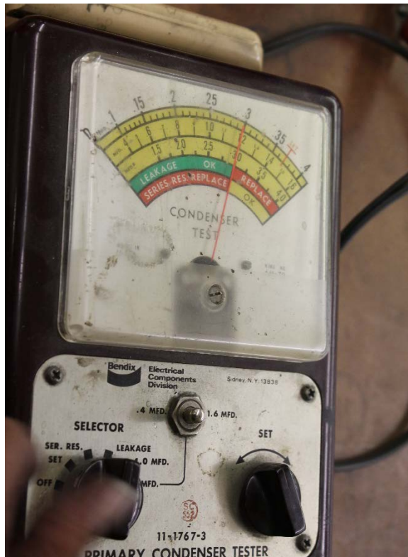
Photo No. 33: View of left magneto's condenser test showing the leakage was not acceptable. (S&T)
