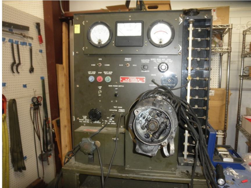
Photo No. 8: Magneto test unit with a magneto installed.
