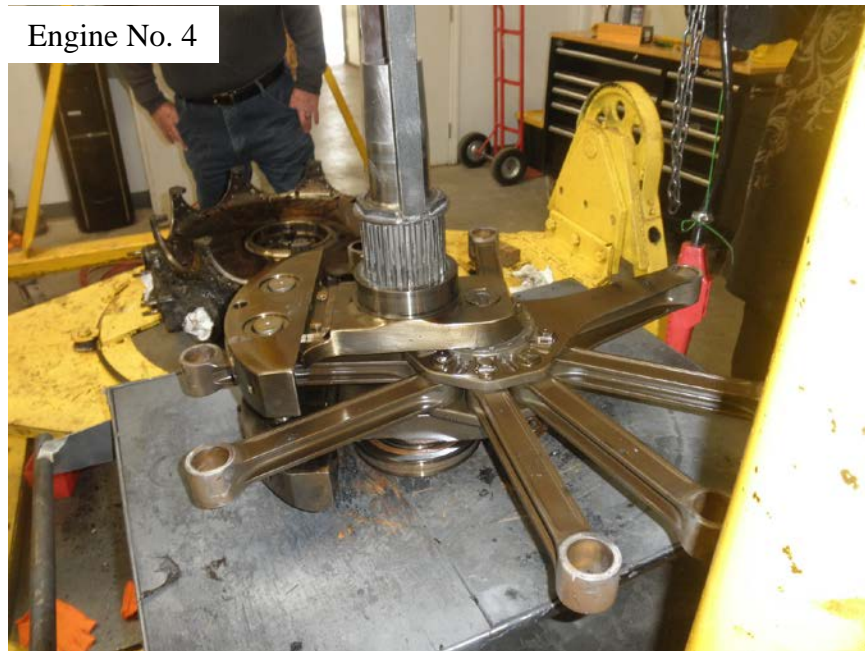
Photo No. 152: View of crank shaft showing it is intact with the two counterweights in place.
