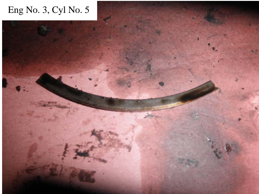
Photo No. 89: Broken piece of piston from No. 5 cylinder's piston.
