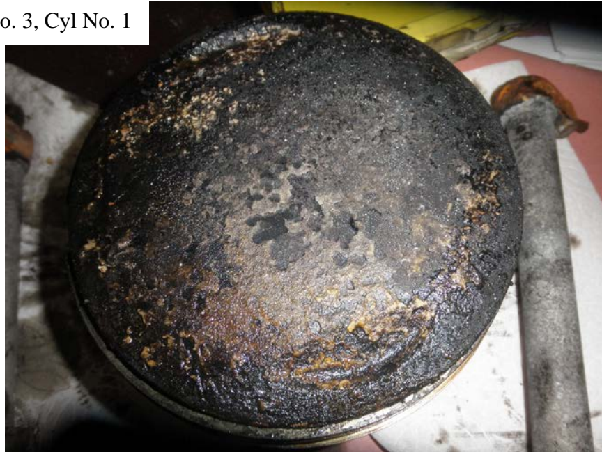
Photo No. 54: Close up view of No. 1 cylinder's piston head showing that it was intact and had a dark color.
