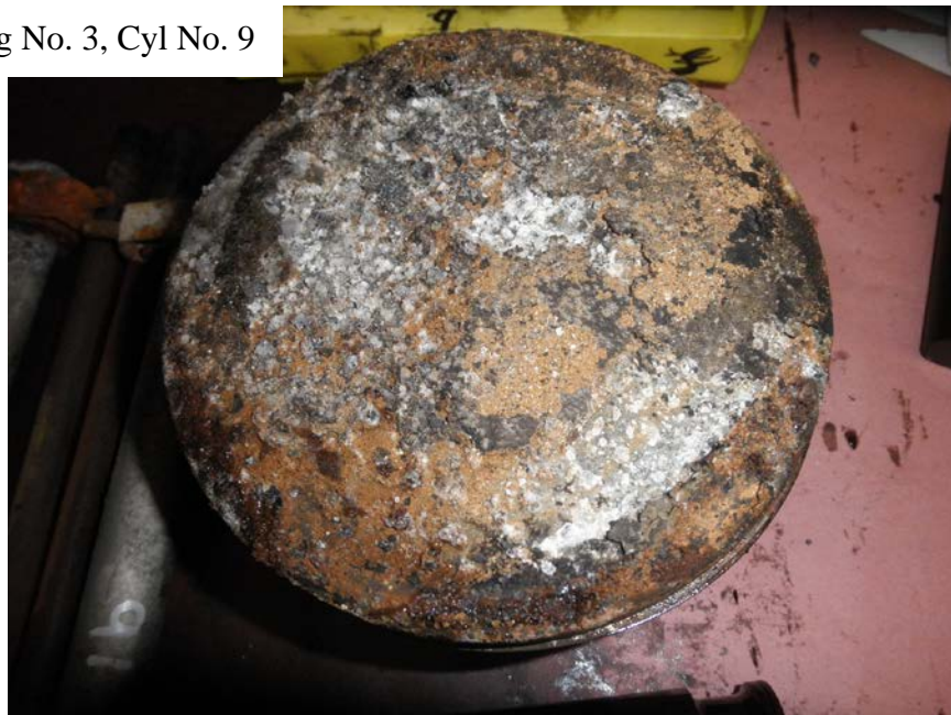
Photo No. 119: Close up view of the head of the No. 9 cylinder's piston showing the brown color with the white crystals consistent with corrosion.
