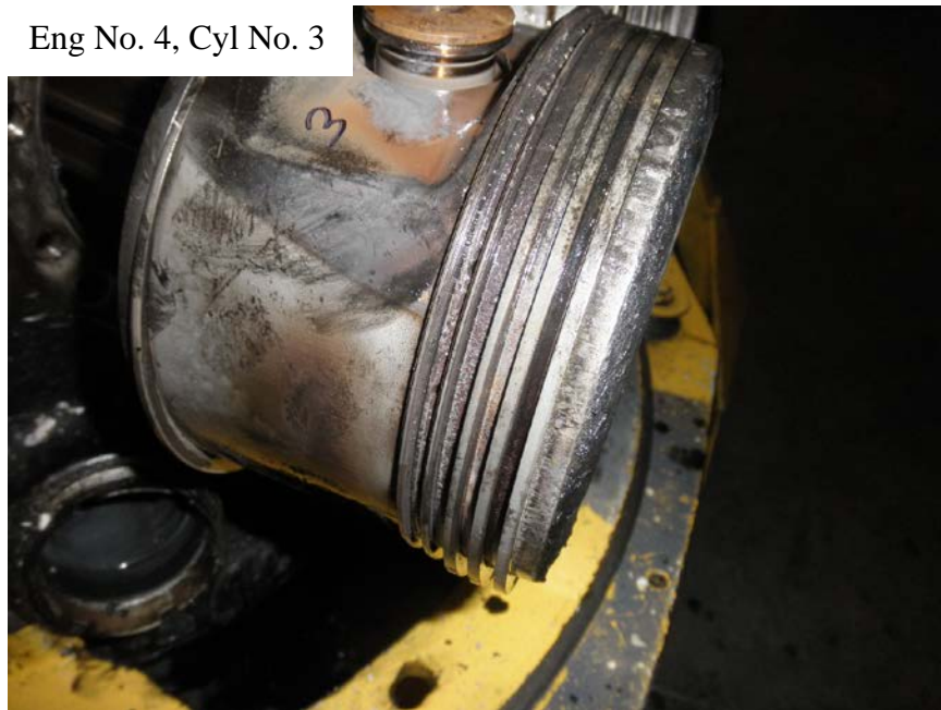
Photo No. 165: View of No. 3 cylinder's piston in place on the articulating rod showing that the piston was intact and that all of the piston rings were in place.
