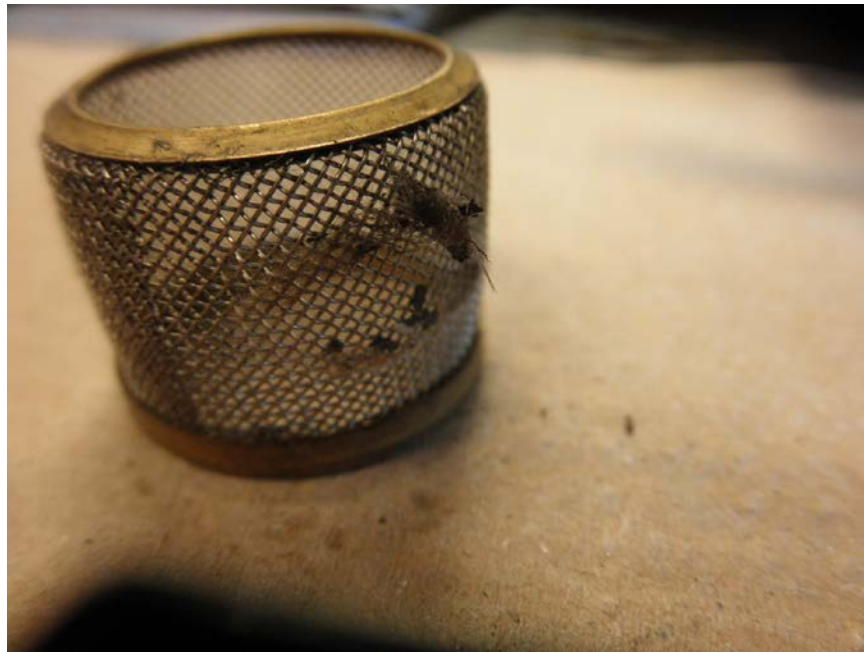
Photo No. 143: Close up view of strainer showing debris.
