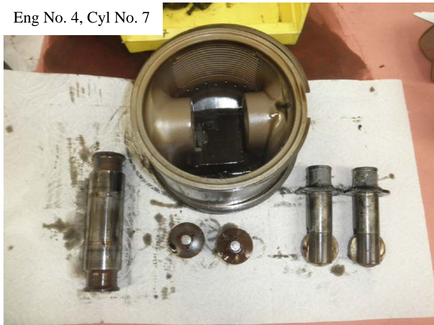
Photo No. 183: View of underside of No. 7 cylinder's piston along with the piston pin, piston pin buttons, and the cam followers showing all were intact and undamaged.
