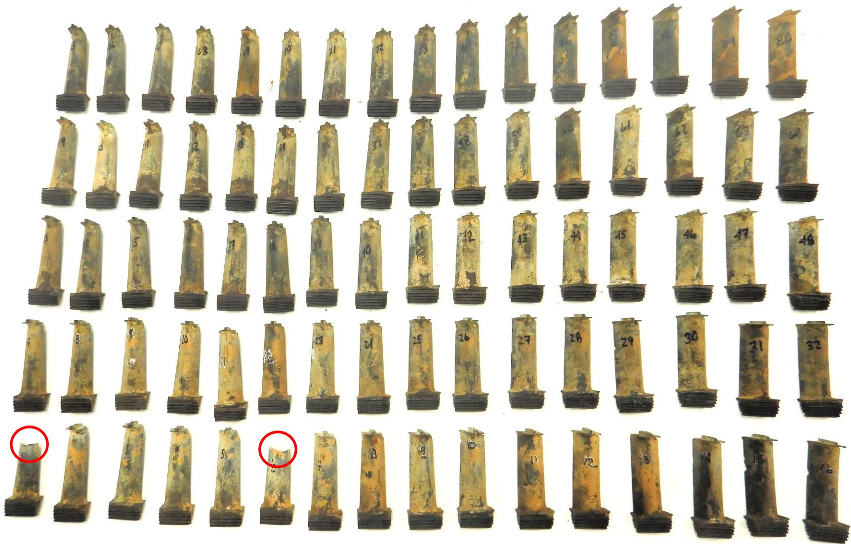
Figure 1: Blade set viewed from convex (suction) side of airfoils. The two indicated blades, #1 and #6, were fractured between 65 and 75 percent span.
