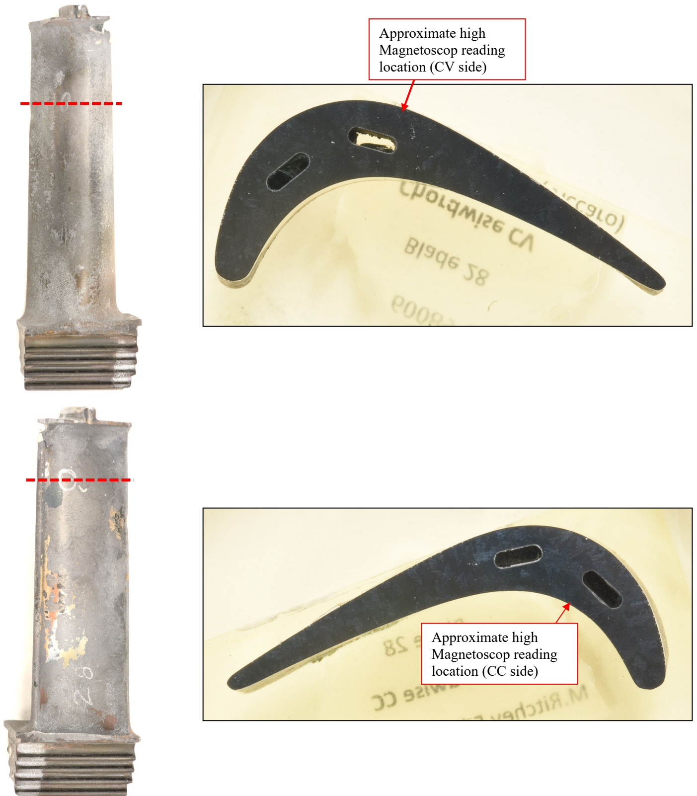
Figure 17: Images showing the locations of the metallographic sections prepared through the highest Magnetoscopy readings on the concave and convex sides of blade 28.
