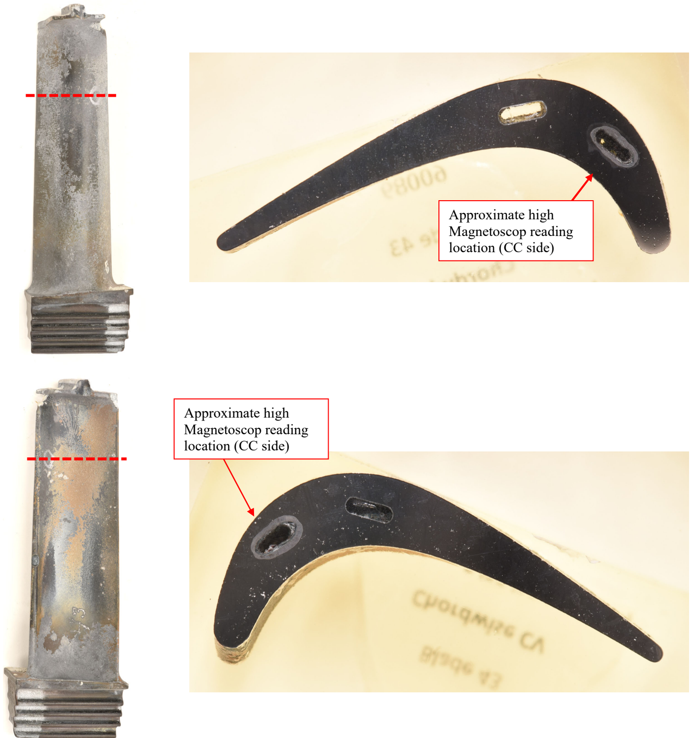
Figure 34: Images showing the locations of the metallographic sections prepared through the highest Magnetoscop readings on blade 43.
