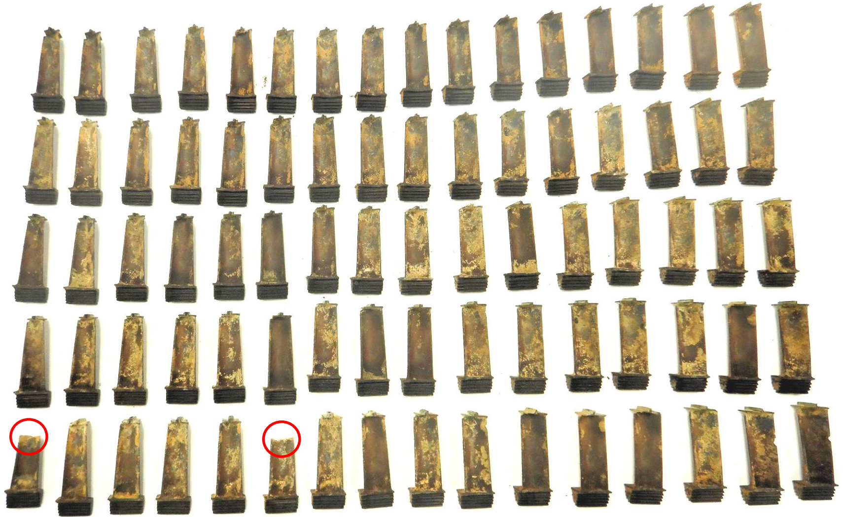
Figure 2: Blade set viewed from concave (pressure) side of airfoils. Two blades, #1 and #6, were fractured.
