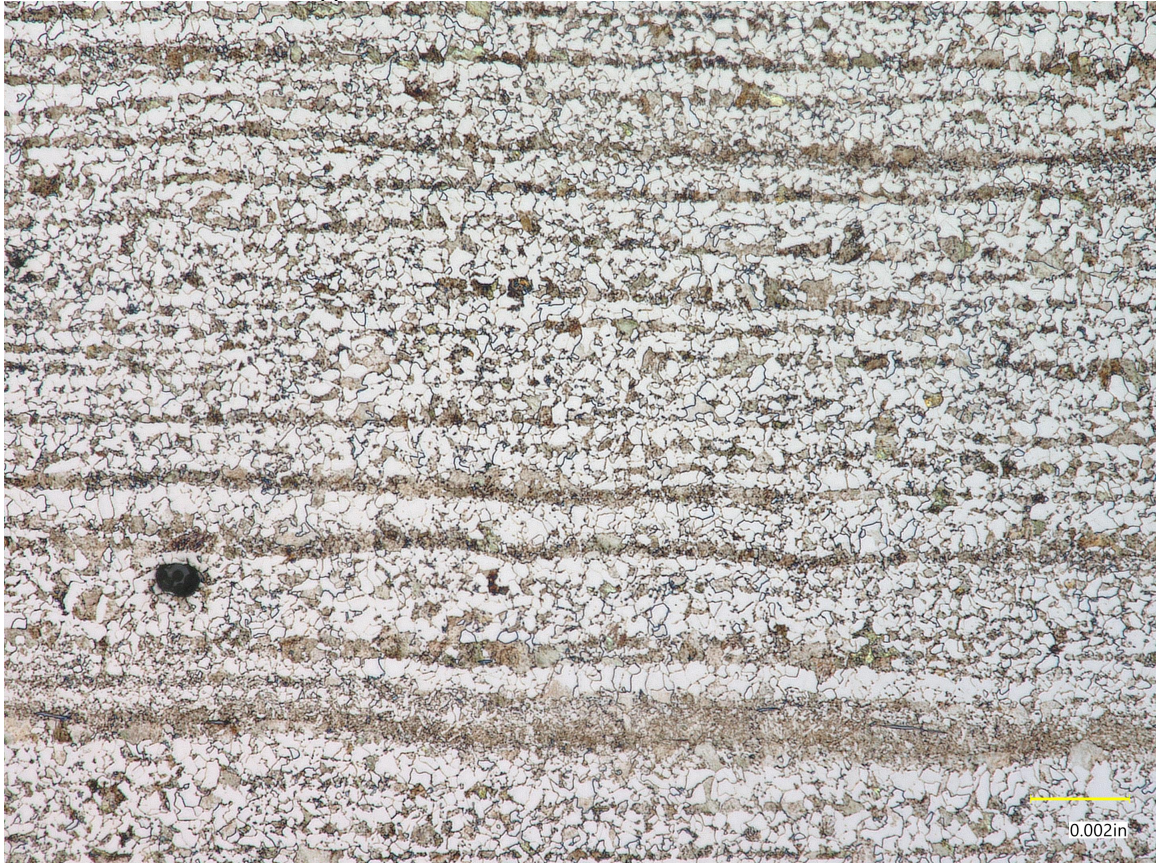
Figure 4 - NATX 400688 Microstructure, Longitudinal Direction, Centerline, 500X Magnification
