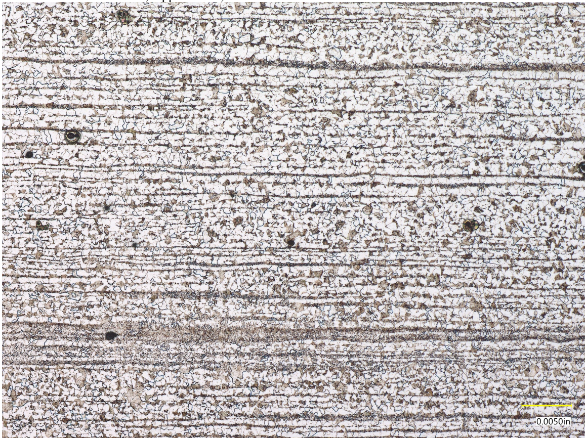
Figure 7 - UTLX 954193 Microstructure, Longitudinal Direction, Centerline, 200X Magnification
