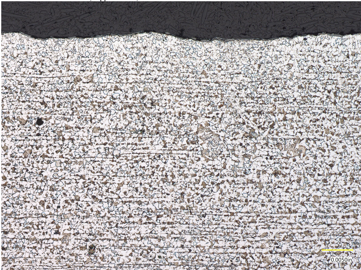
Figure 5 - UTLX 954193 Microstructure, Longitudinal Direction, Surface, 200X Magnification
