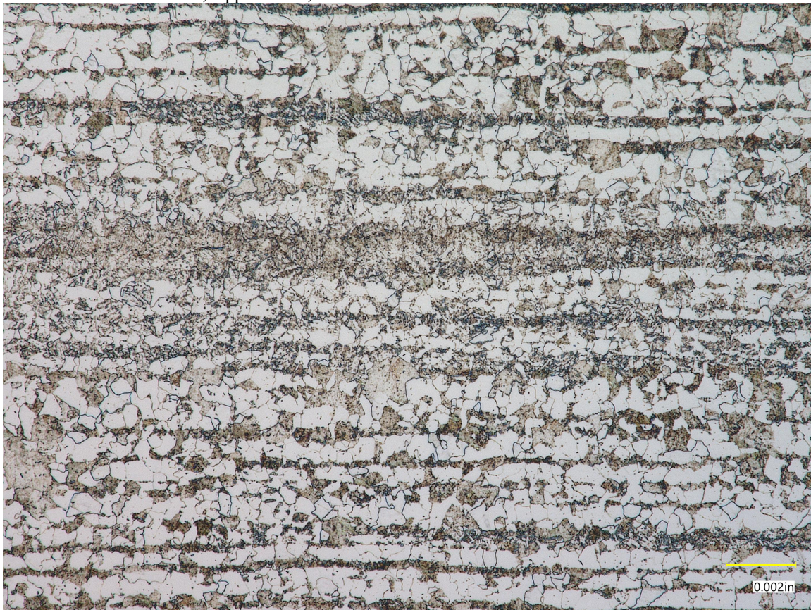
Figure 8 - UTLX 954193 Microstructure, Longitudinal Direction, Centerline, 500X Magnification
