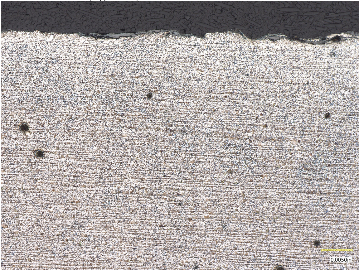
Figure 1 - NATX 400688 Microstructure, Surface, Longitudinal Direction, 200X Magnification
