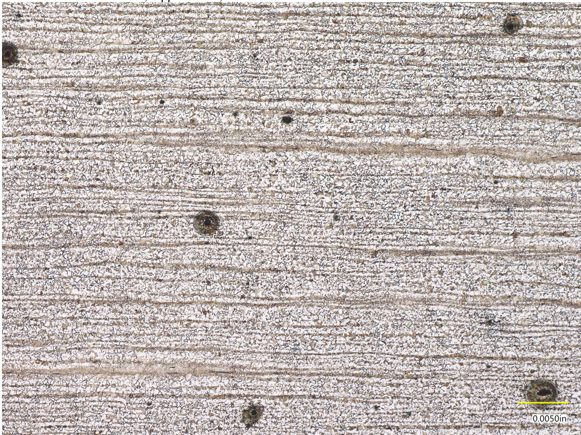
Figure 3 - NATX 400688 Microstructure, Longitudinal Direction, Centerline, 200X Magnification
