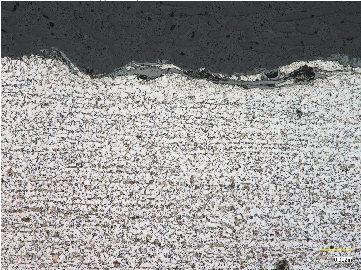
Figure 2 - NATX 400688 Microstructure, Surface, Longitudinal Direction, 500X Magnification
