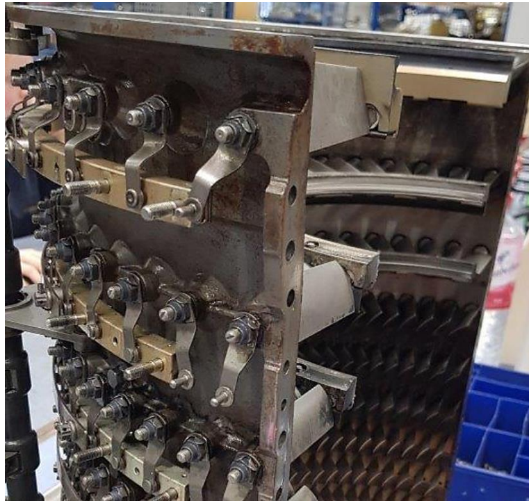
HPC case with corrosion
