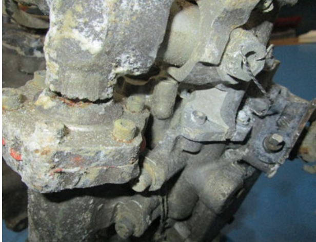
Figure 7 Fractured CDP limiter housing
