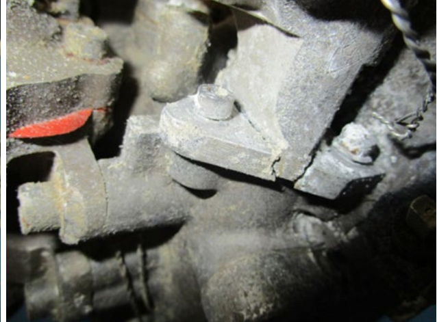
Figure 8 Motor bellows cover flange fractures
