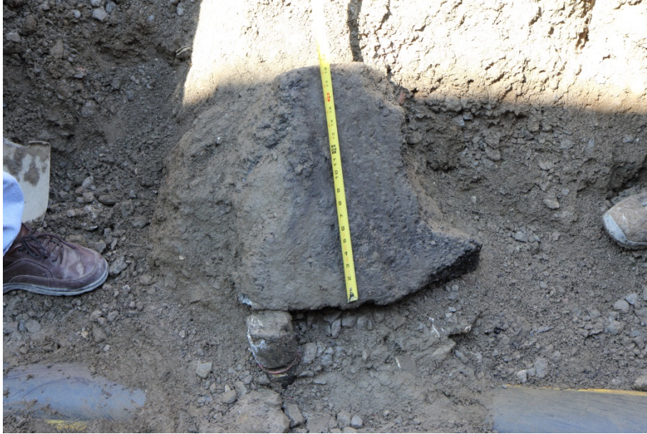
Figure 7: Re-excavation at 1642 Park Avenue shows asphalt piece on top of service saddle tee cap that measured about 19 inches high during field investigation. Source: NYPSC.
