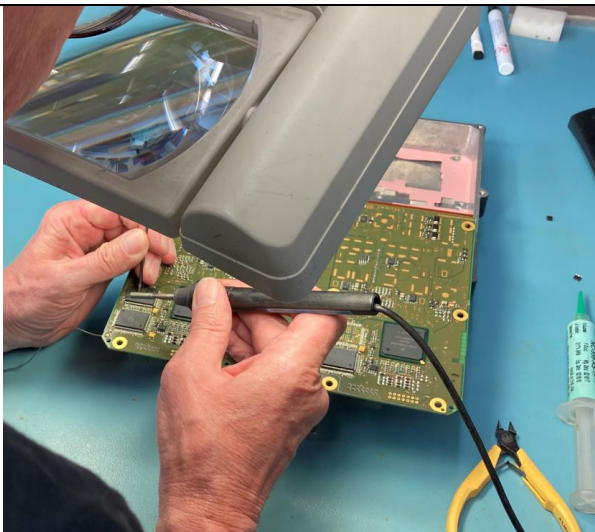
Figure 20 - EECU s/n 1657 MB memory installation
