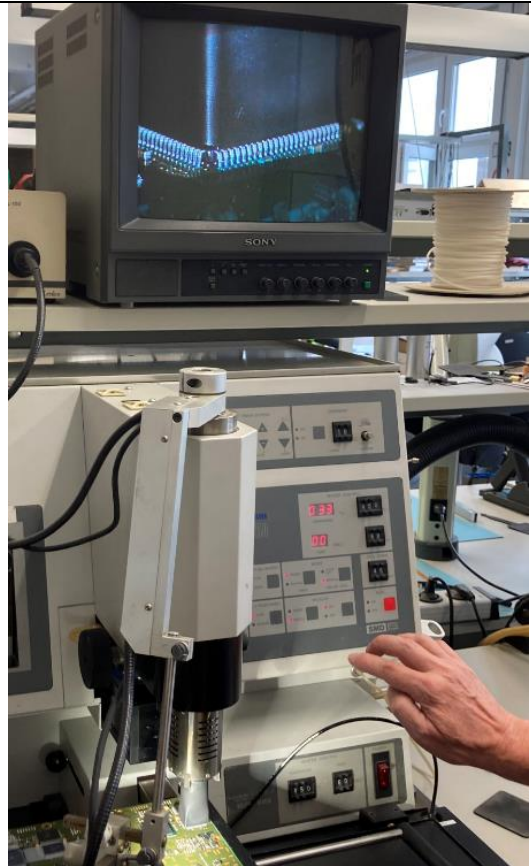
Figure 19 - EECU s/n 2786 MB memory removal
