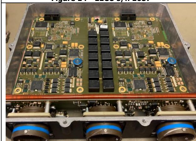
Figure 16 - EECU s/n 1657 MB upper side
