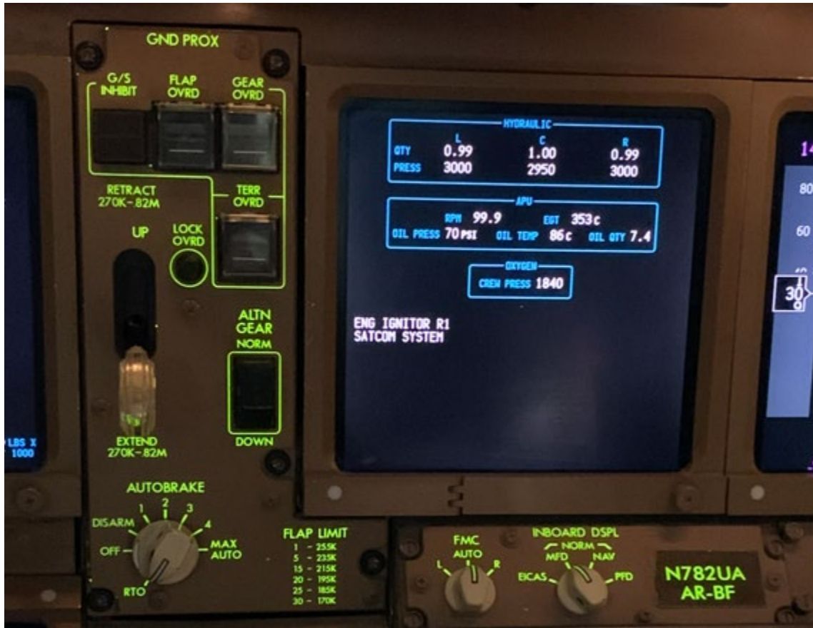
Photo #4; Status page showing a fault with the Right Engine #1 igniter.
