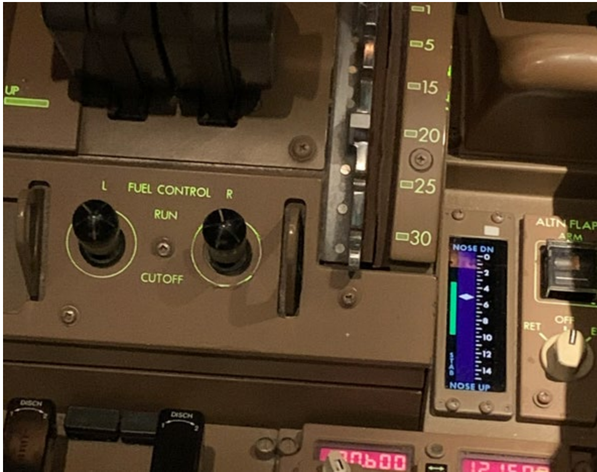
Photo #2. Left and Right Fuel Control switches in the Run, Run position
