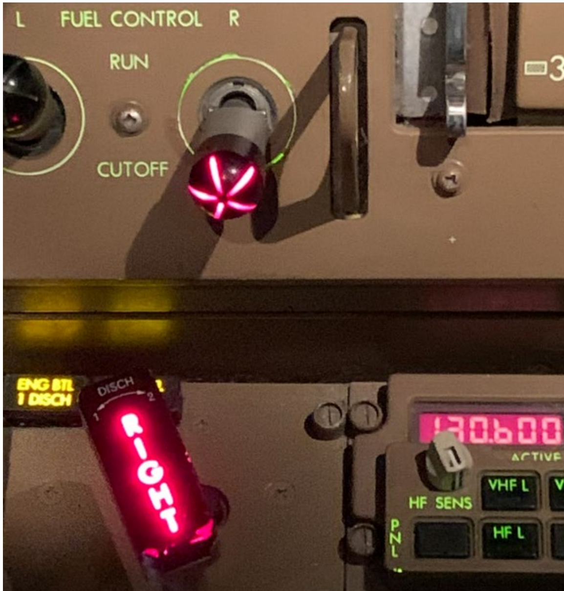
Photo # 7: Right engine fire with the R Fuel Controller shutoff and both fire bottles discharged.
