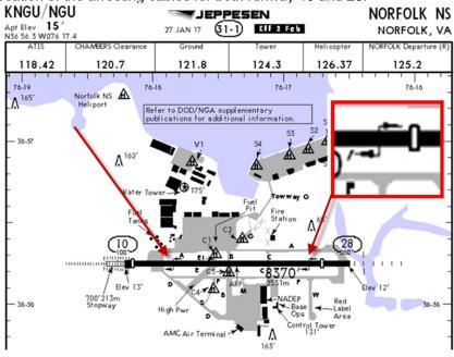
The location of the arresting cables is marked on the runway by yellow, reflective discs, 10 feet in diameter that span the width of the runway.
