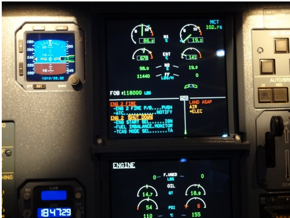
Photo 8: ENG 2 FIRE message and Additional Prioritized messages
