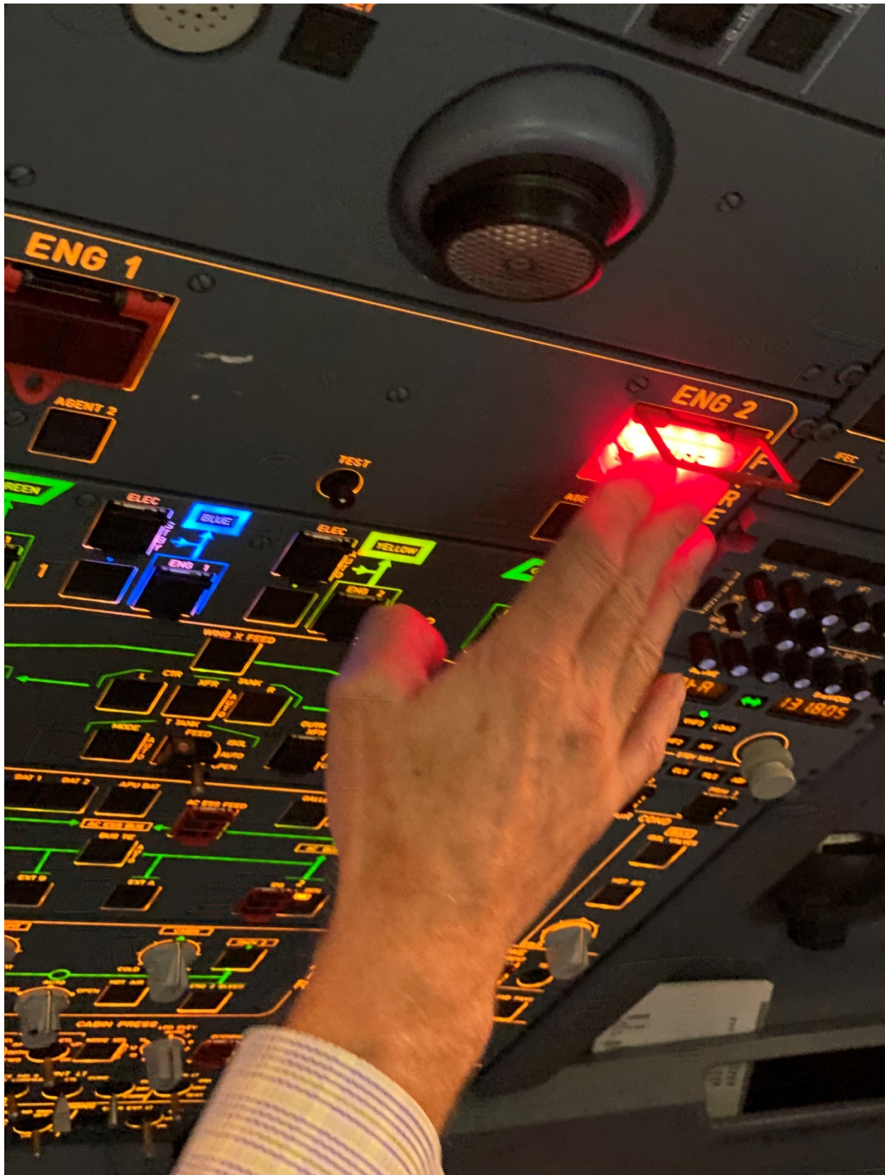
Photo 10: ENG 2 FIRE P/B on Upper Center Panel
