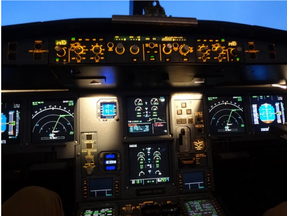
Photo 7: Liftoff + 15 seconds ENG 2 FIRE message 7
