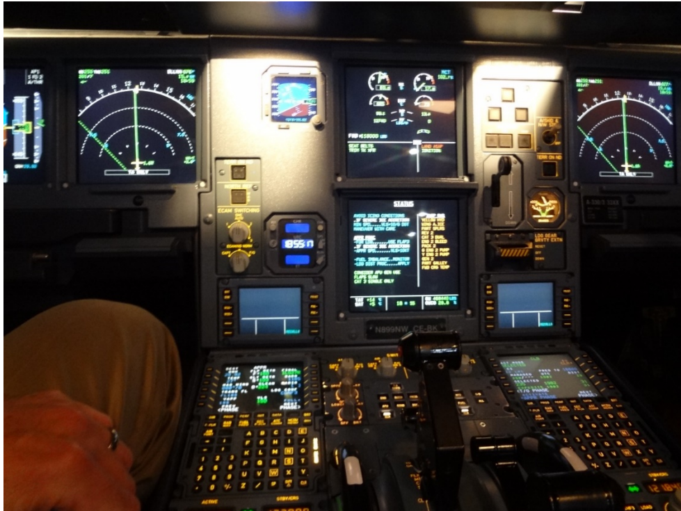
Photo 16: Status Messages on ECAM
