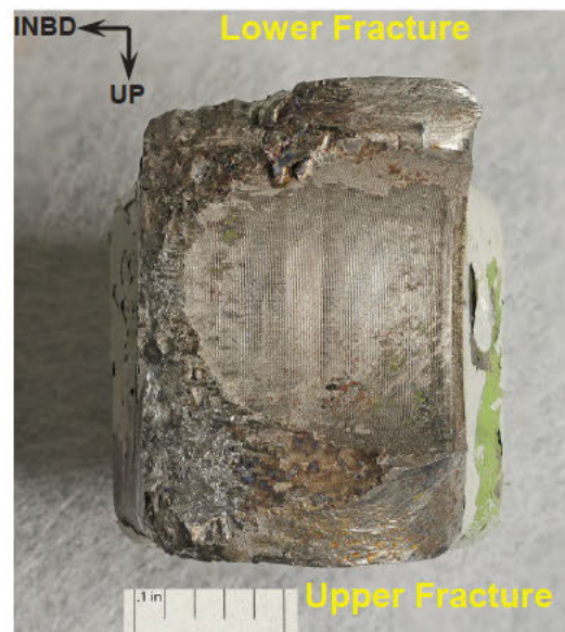
Figure 7. Close-up of mating fracture surfaces of Lower Torque Arm
