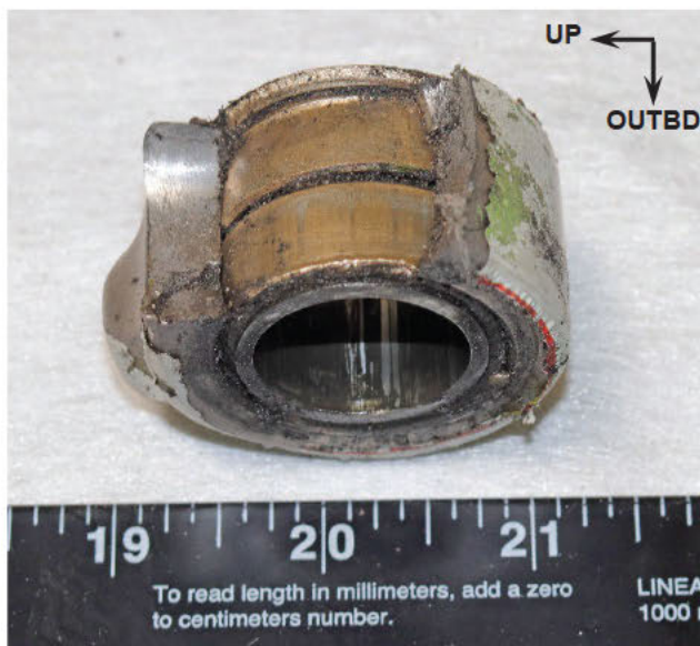
Figure 6. Close-up of fracture surfaces of Lower Torque Arm
