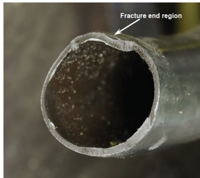
Figure 65. Close-up of fracture surface [Retract Rod]
