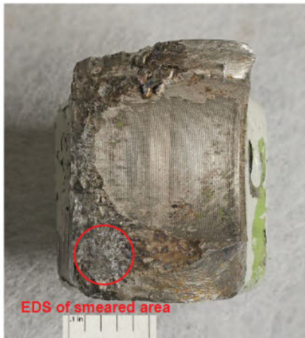
Figure 24. Close-up of mating fracture surface [Lower Torque Arm]
