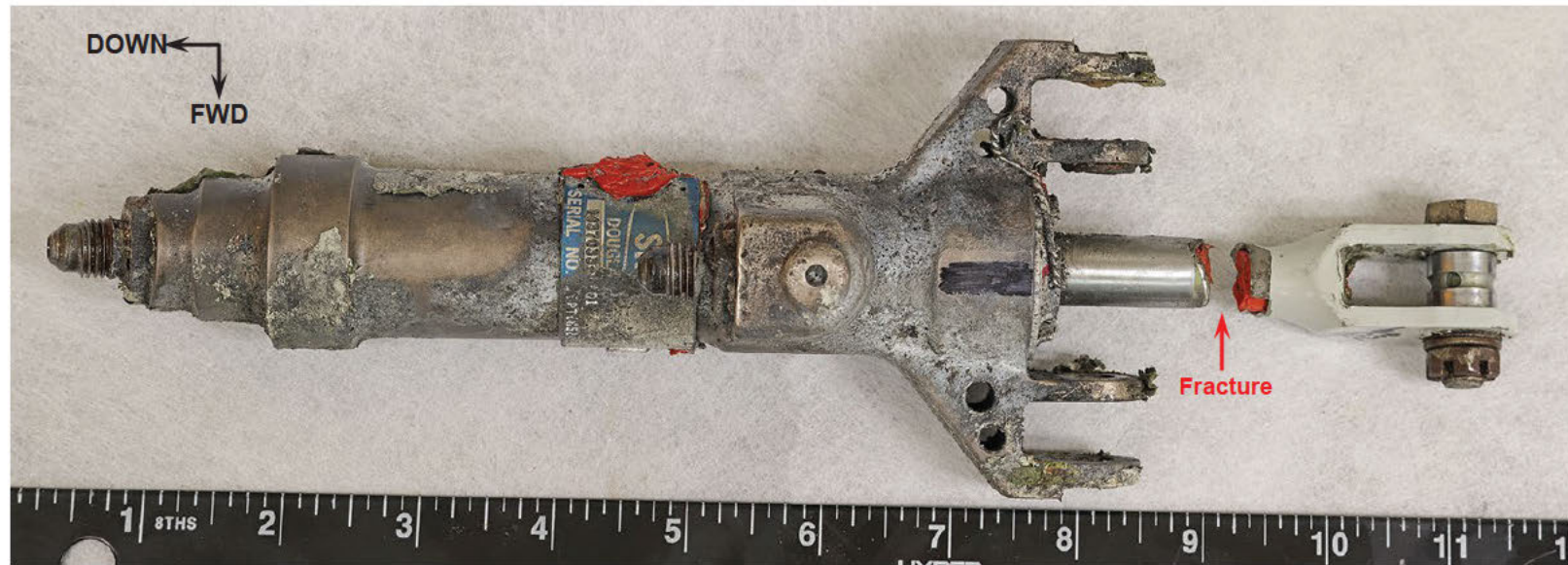
Figure 94. Close-up of fractured Bungee Piston after removal
