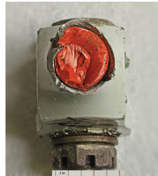
Figure 96. Close-up of fracture surface at clevis lug end
