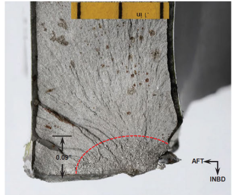
Figure 37. Close-up of secondary origin area.
