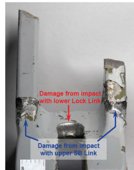
Figures 29 and 30. Close-up of witness marks in Links from contact during hyper-extension
