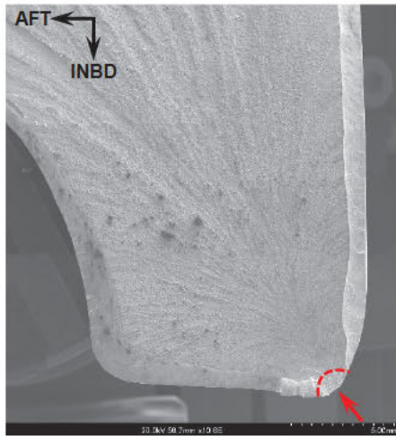
Figure 58. Close-up of origin area [Lower Side Brace]
