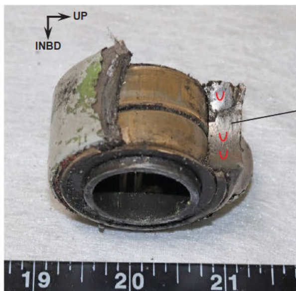
Figure 11. Close-up of fracture surfaces Red ellipses indicate direction of open-ended dimple formations. [Lower Torque Arm]
