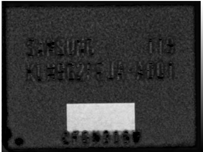
Second chip with shadow of the top chip and wirebonds
