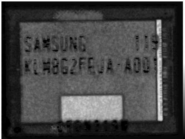
Chip carrier with shadow of the chips and wirebonds
