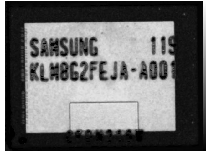
Second chip with shadow of the top chip and wirebonds
