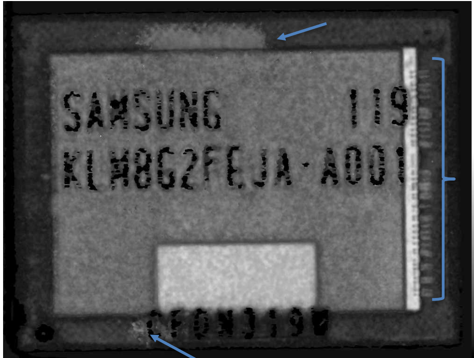
Chip carrier damaged area
