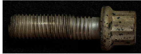
FIGURE 19: PN 5318316-01 TMS LOWER AFT CASE MOUNT; CLOSE-UP VIEWS OF CRACKED BOLT
