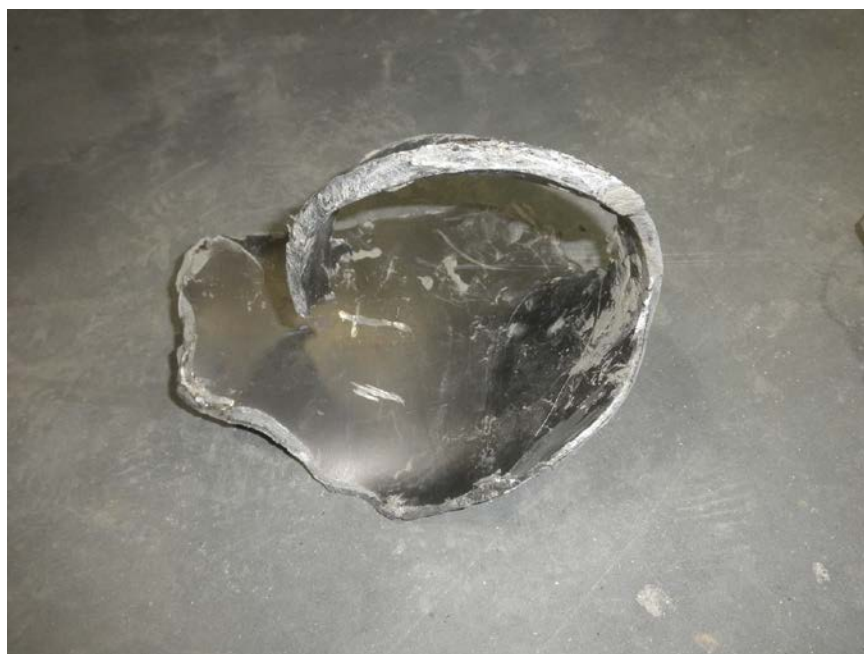
Photo No. 39: Close up view of a piece of stub shaft that is twisted back onto itself.
