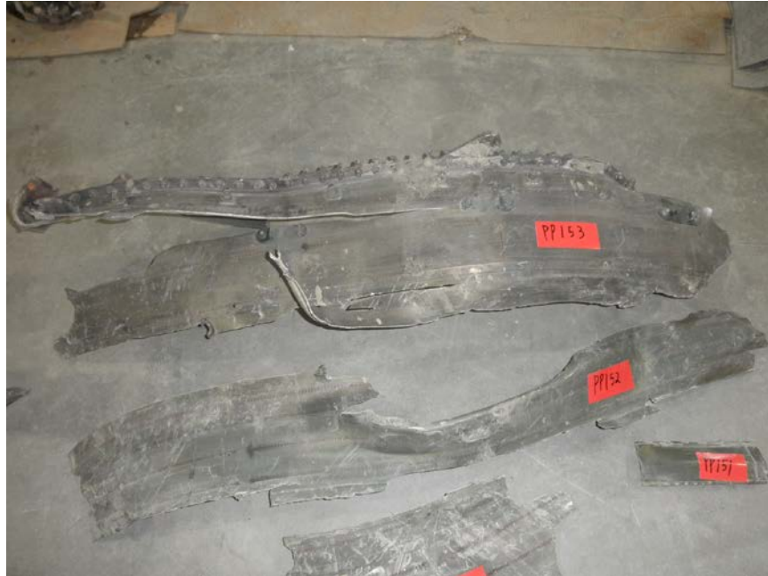
Photo No. 42: Broken pieces of LPT case.
