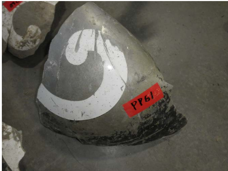
Photo No. 35: Broken piece of spinner cap.
