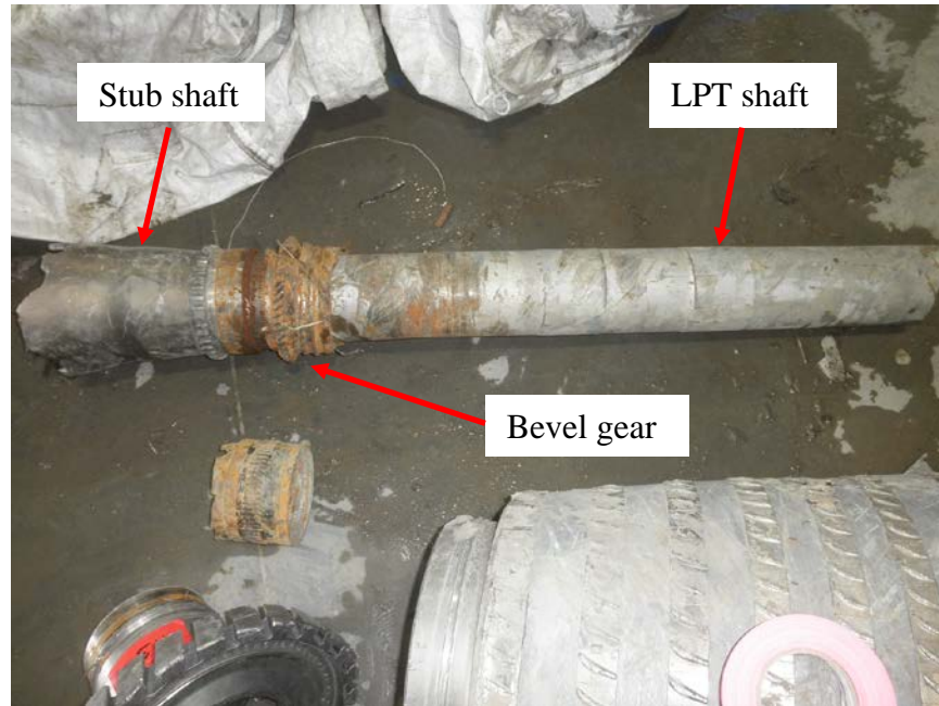
Photo No. 16: The No. 1 engine's stub shaft and LPT shaft.
