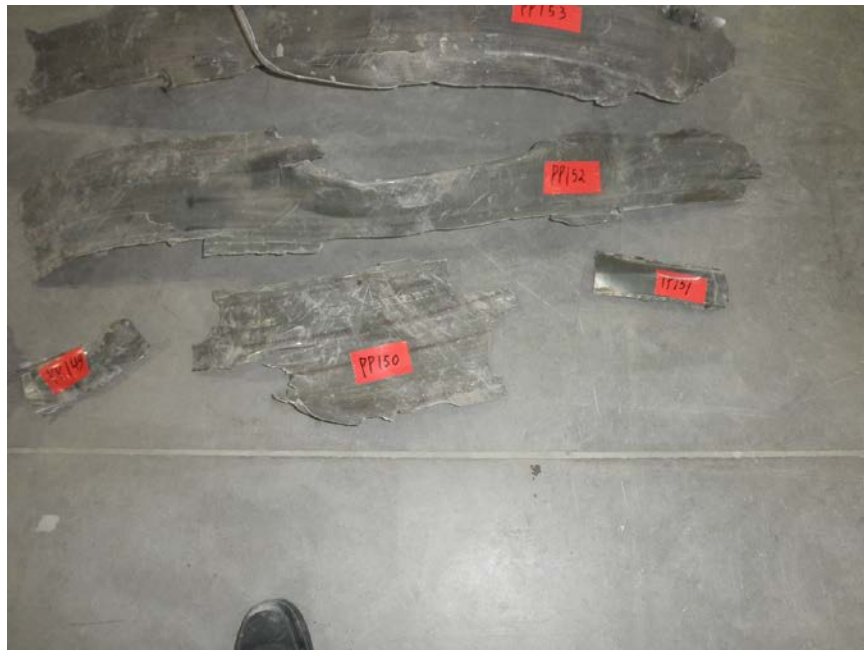
Photo No. 43: Broken pieces of LPT case.
