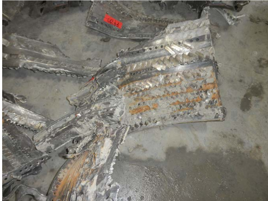
Photo No. 41: View of several broken pieces of HPC case.
