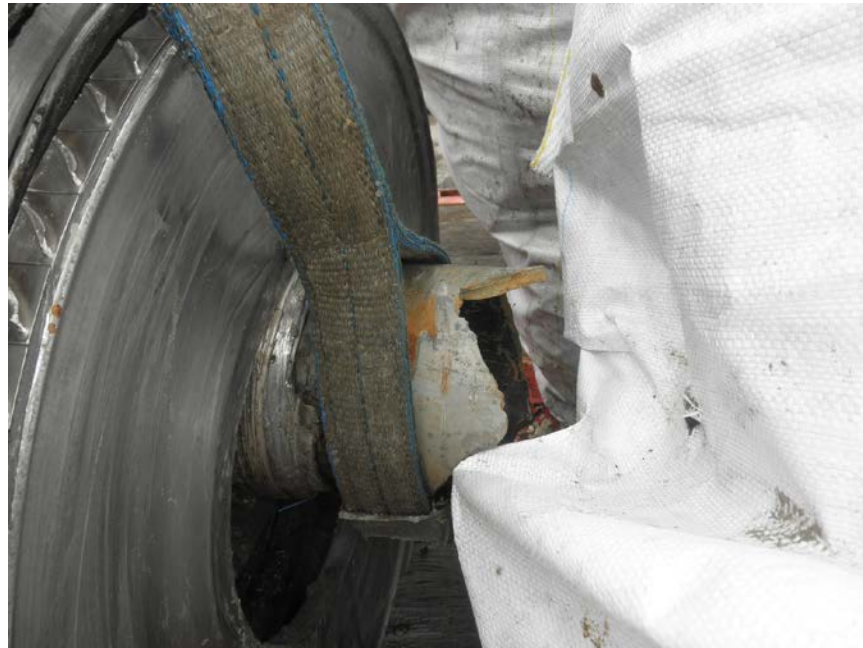
Photo No. 17: The broken aft end of the No. 1 engine's LPT shaft.
