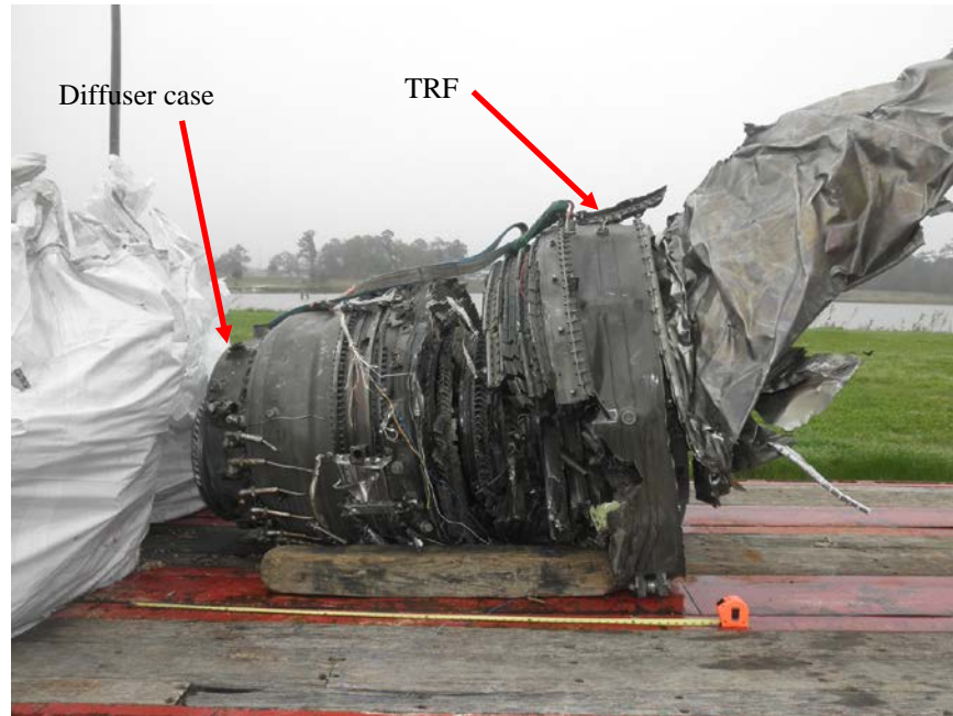
Photo No. 1: Largest piece of No. 1 (left) engine recovered that extended from front of diffuser on left to turbine rear frame on the right. To the right of the turbine rear frame is the crushed exhaust duct.
