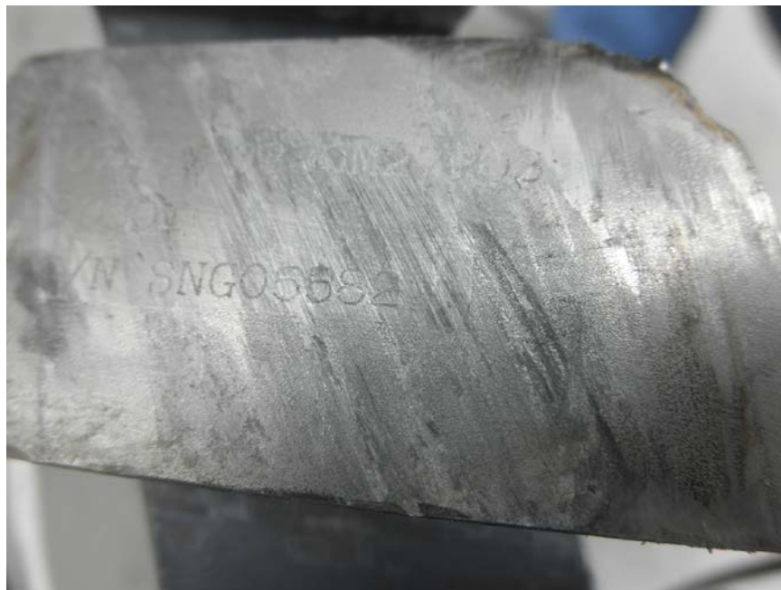
Photo No. 9: Serial number of No. 1 engine's HPC stage 2 disk.
