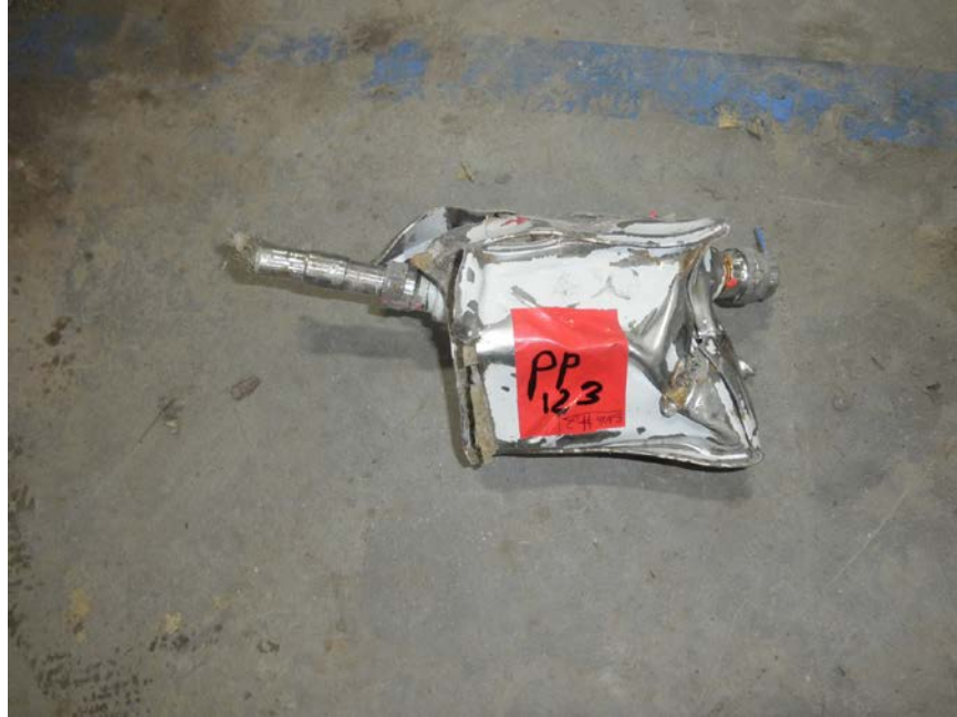
Photo No. 47: Ignition exciter box.
