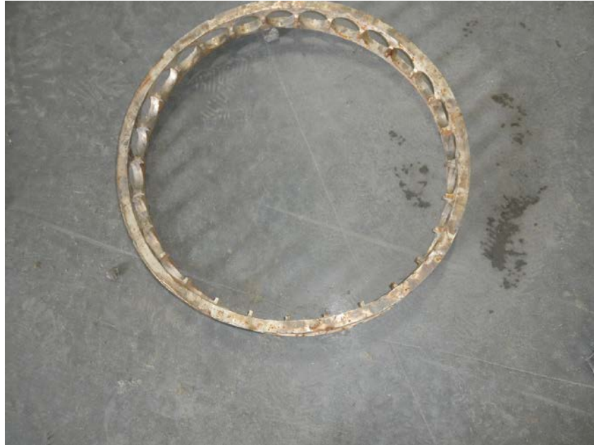
Photo No. 33: Close of the No. 2 engine's No. 1 bearing cage.
