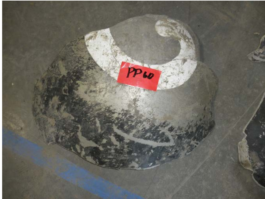
Photo No. 34: Broken piece of spinner cap.
