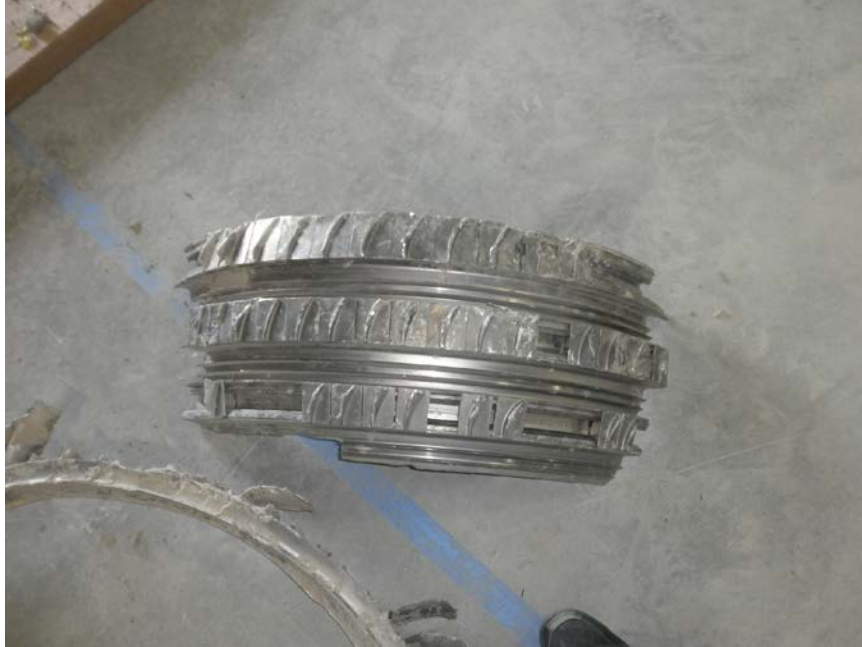
Photo No. 6: Piece of No. 1 engine's booster spool, stages 1 through 3.
