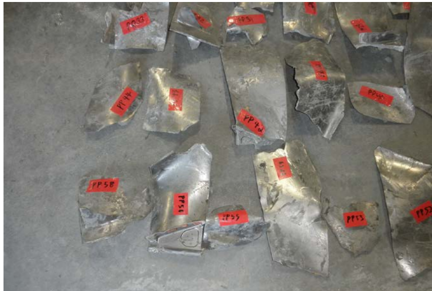
Photo No. 37: Broken pieces of fan blade.
