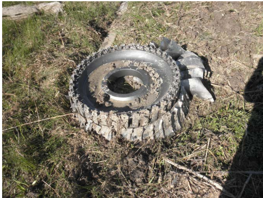
Photo No. 22: The No. 2 engine's fan disk laying face up on marshy ground at the crash site.
