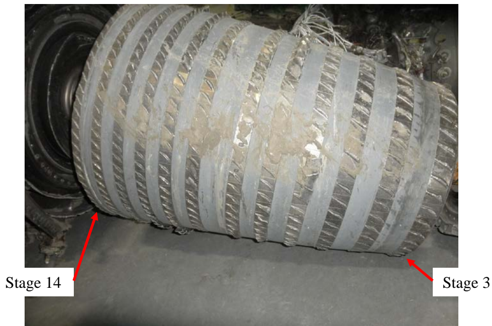
Photo No. 27: The No. 2 engine's HPC between stages 3 and 14.
