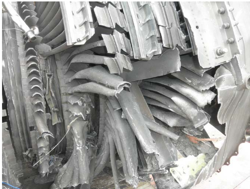
Photo No. 20: Close up view of the No. 1 engine's LPT blades that are bent and broken.
