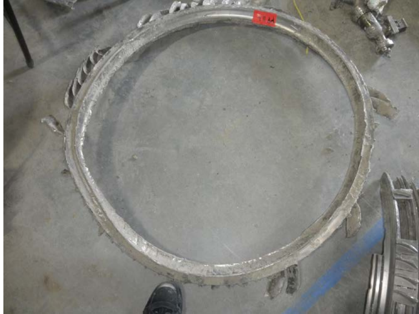
Photo No. 7: The No. 1 engine's booster stage 4 disk rim.
