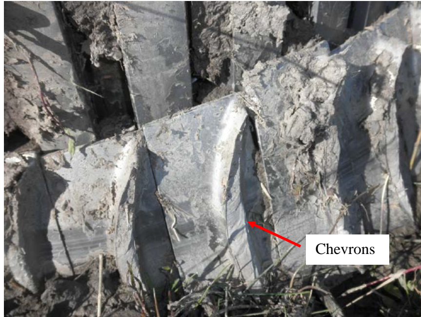
Photo No. 23: Close up of the No. 2 engine's fan blade fracture surfaces showing the chevrons pointing forward.
