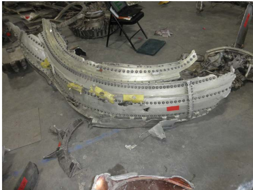
Photo No. 40: Large piece of spool case.
