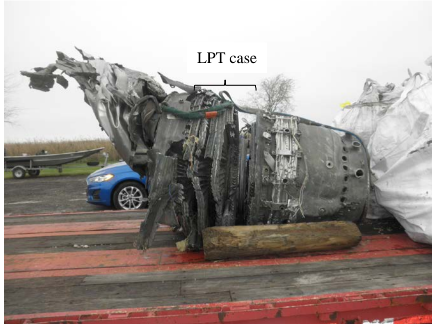
Photo No. 19: The right side of No.1 engine showing the LPT case between the diffuser case and turbine rear frame on a truck bed.
