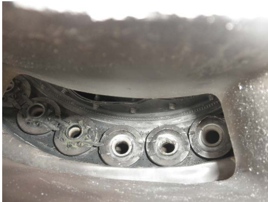
Photo No. 14: The No. 1 engine's combustor dome showing no metal spray.
