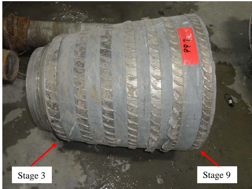
Photo No. 10: The No. 1 engines HPC stage 3-to-9 spool with blades broken off adjacent to platform or bent over opposite the direction of rotation.
