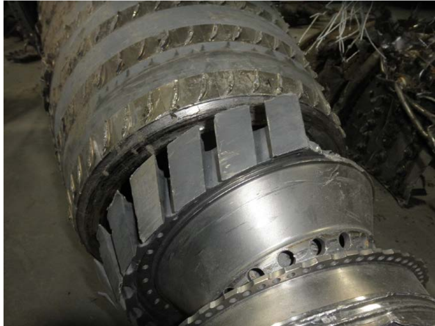
Photo No. 26: Close up of the No. 2 engine's HPC stage 2 disk.
