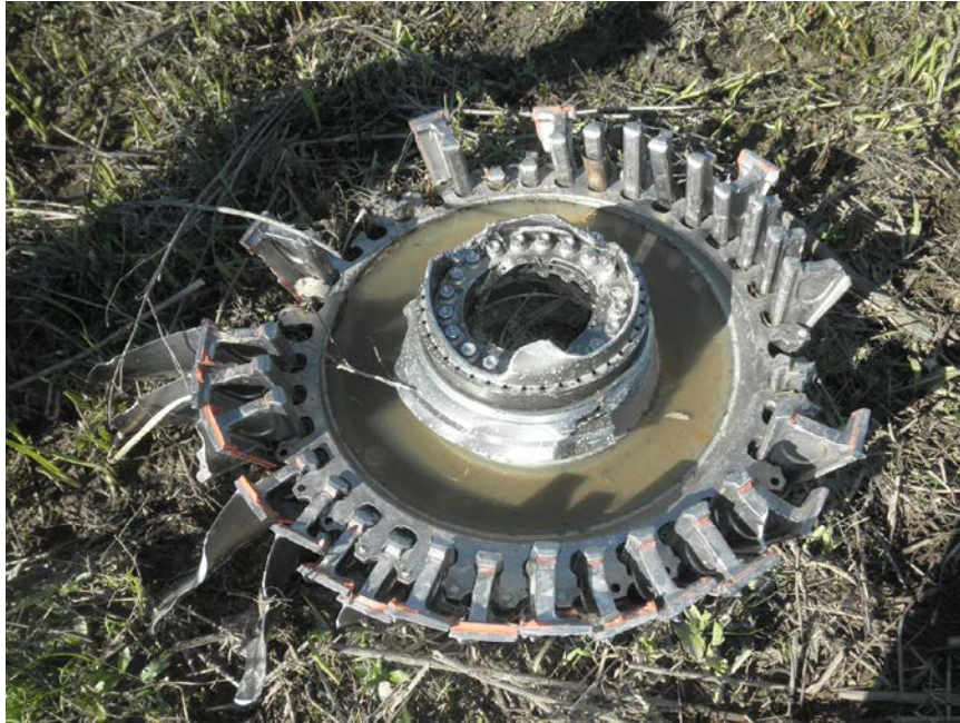
Photo No. 5: Left engine's fan disk, front face down, with 28 of 38 fan blades in place in the blade slots, laying on marshy ground at the crash site. The forward end of the stub shaft is still bolted in place to the rear of the fan disk.
