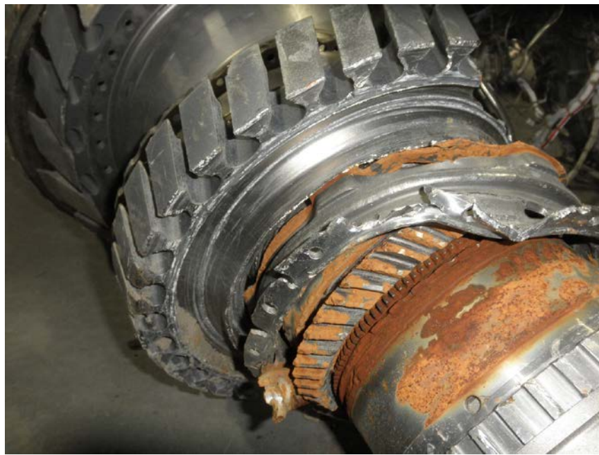
Photo No. 25: Close up of the No. 2 engine's HPC stage 1 disk.
