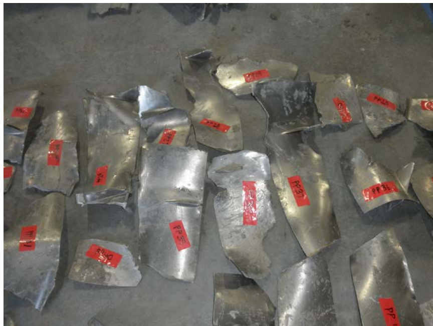
Photo No. 38: Broken pieces of fan blade.
