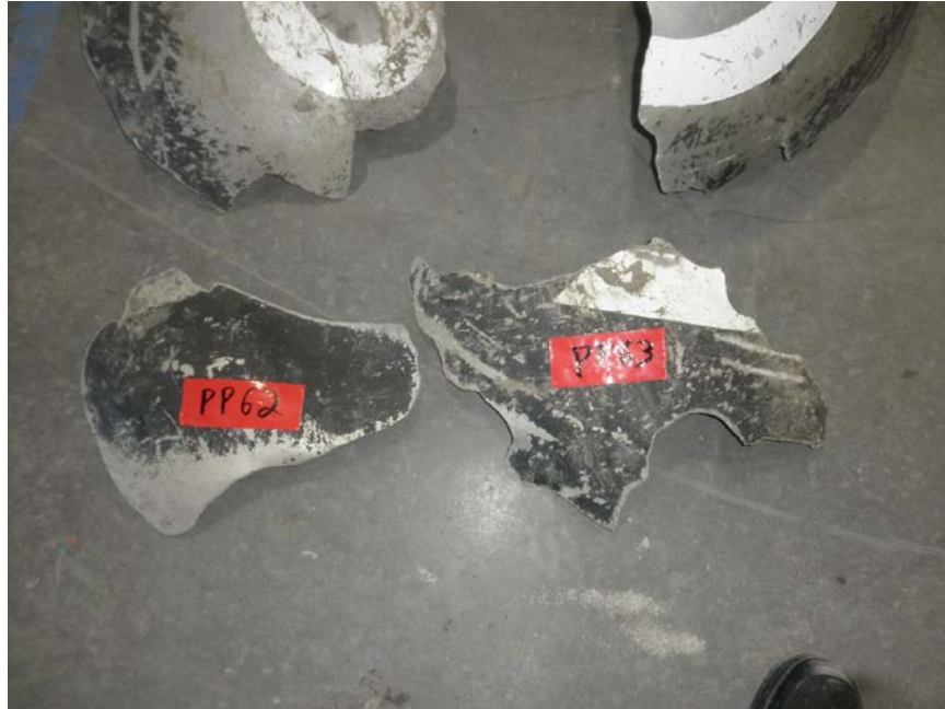
Photo No. 36: Two broken pieces of spinner cap.
