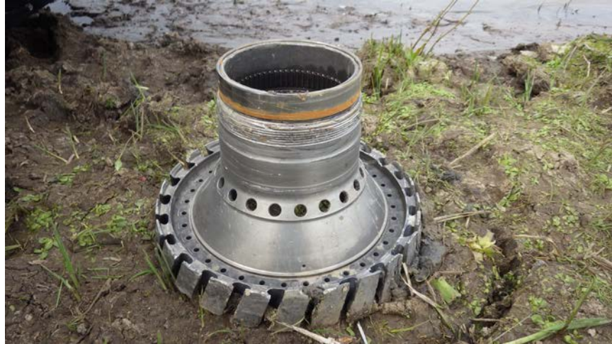
Photo No. 3: HPC stage 2 disk, PN 9380M27P03 SN SNG05682, laying on the ground, front side up, at the crash site identified from records as having been installed in the No. 1 (right) engine. (GE)
