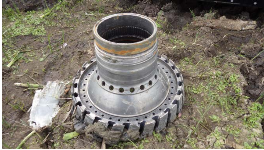
Photo No. 8: The No. 1 engine's HPC stage 2 disk laying on the ground at the crash site. (GE)
