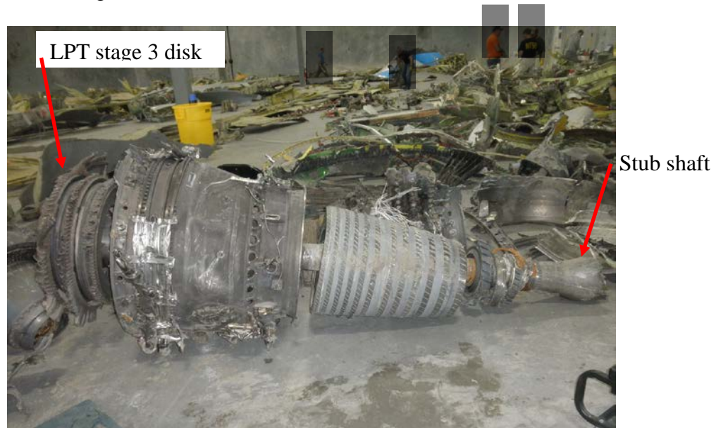
Photo No. 2: Largest piece of No. 2 (right) engine recovered that extended from stub shaft on the right to LPT stage 3 disk on the left.
