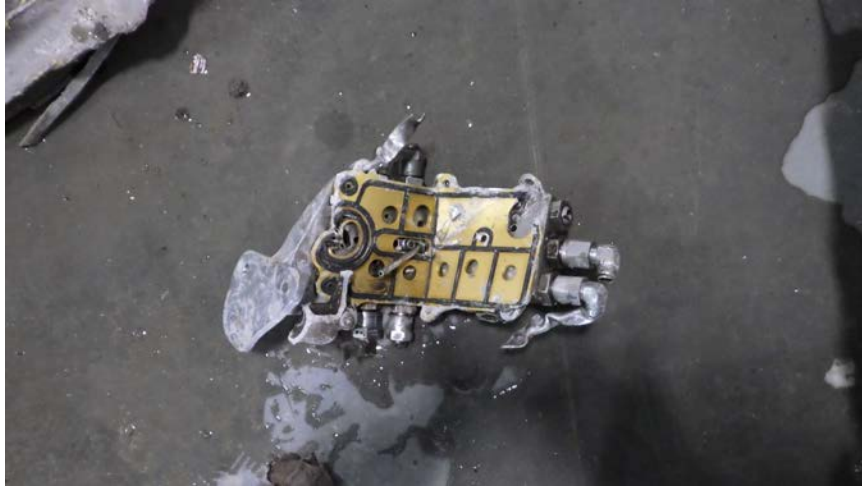
Photo No. 49: Drain mast manifold. (GE)
