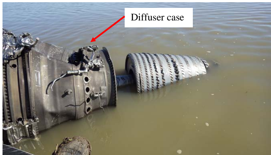
Photo No. 28: The No. 2 engine's diffuser case when it was still in the water at the crash site. (GE)
