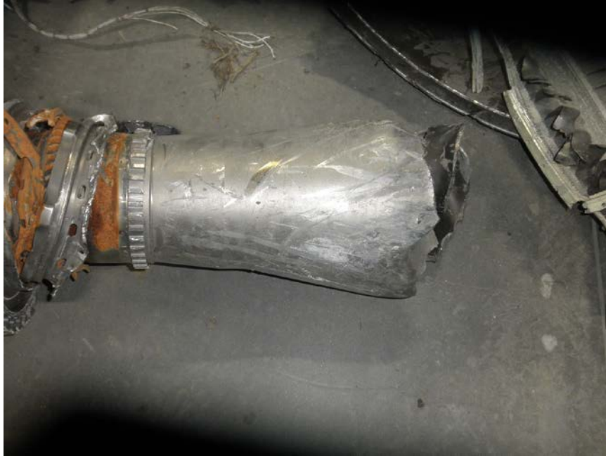
Photo No. 30: The No. 2 engine's stub shaft.
