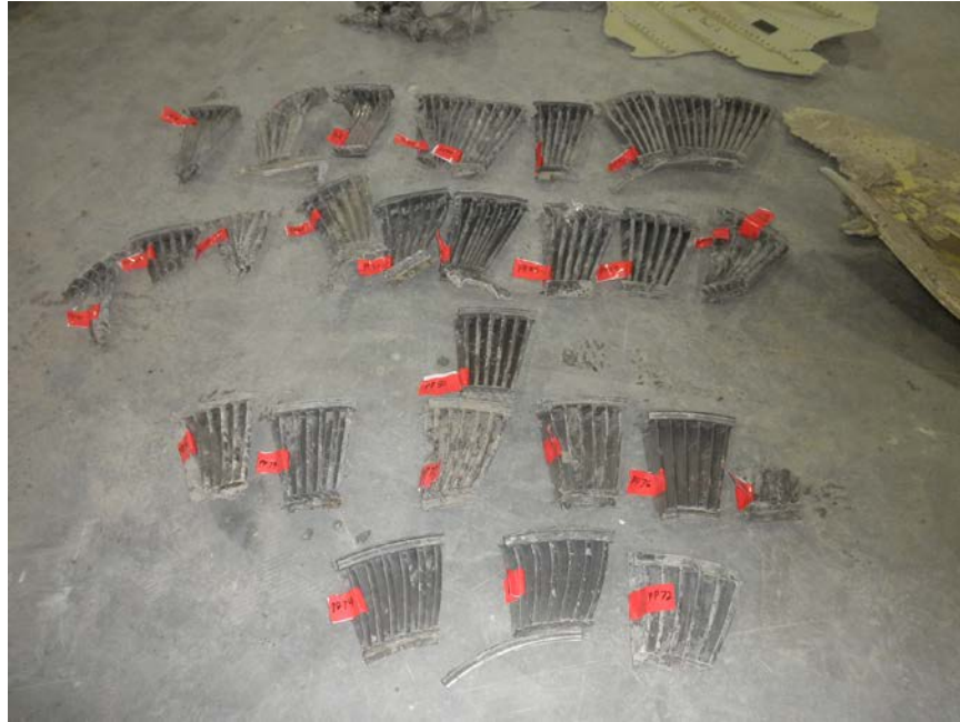
Photo No. 44: LPT vane segments.
