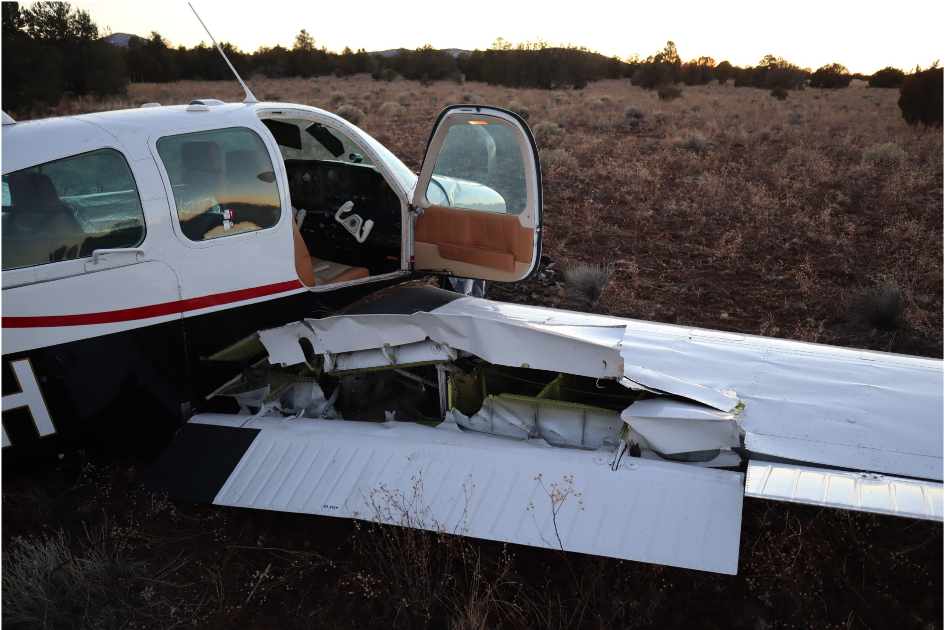
Photo 3 - Rear view of right-wing damage (photo courtesy of the FAA)
