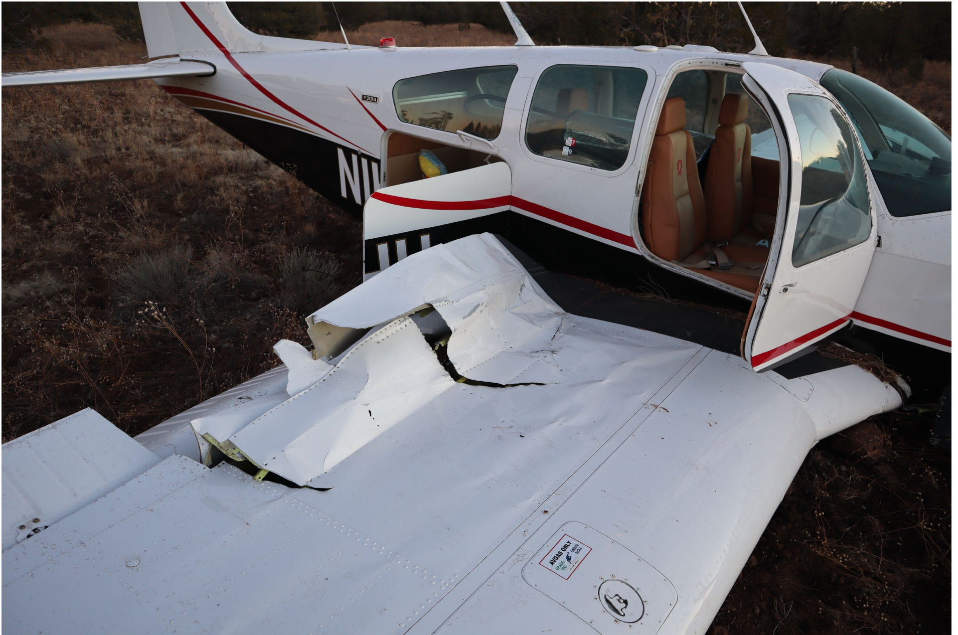
Photo 2 - Front view of right-wing damage (photo courtesy of the FAA)
