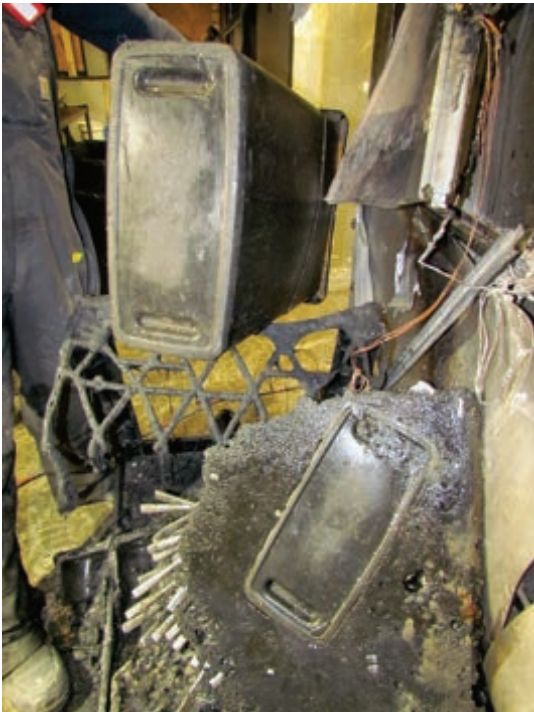
232. Remains of melted plastic trash can removed from port aft wait staff station for contents examination.
