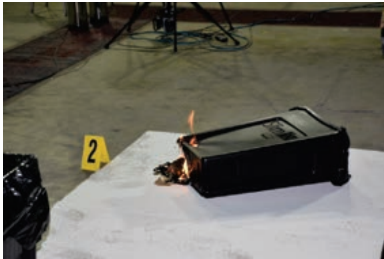
247. Screen capture of ambient environment and forward looking infrared (FLIR) camera video of exemplar plastic trash can fire research testing.
