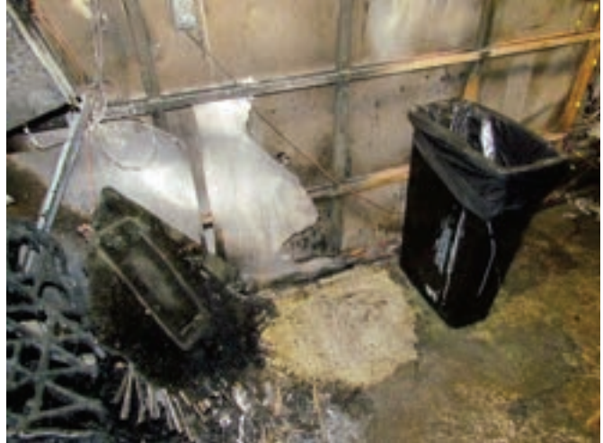
232. Remains of melted plastic trash can removed from port aft wait staff station for contents examination.
