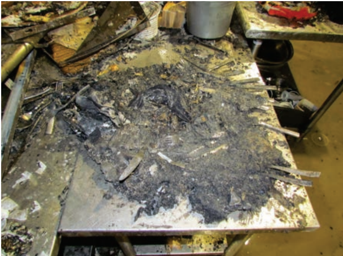
232. Remains of melted plastic trash can removed from port aft wait staff station for contents examination.
