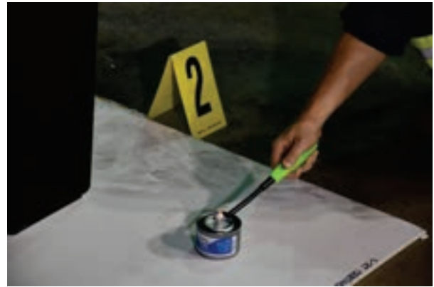
246. Sequential photographs of exemplar plastic trash can FRL testing.
